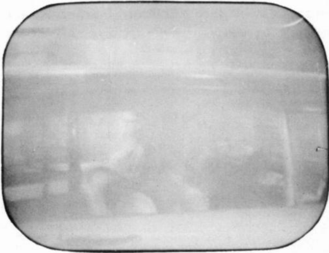
Fig. 410. Excessive agc bias voltage can produce a weak, washed-out picture.
