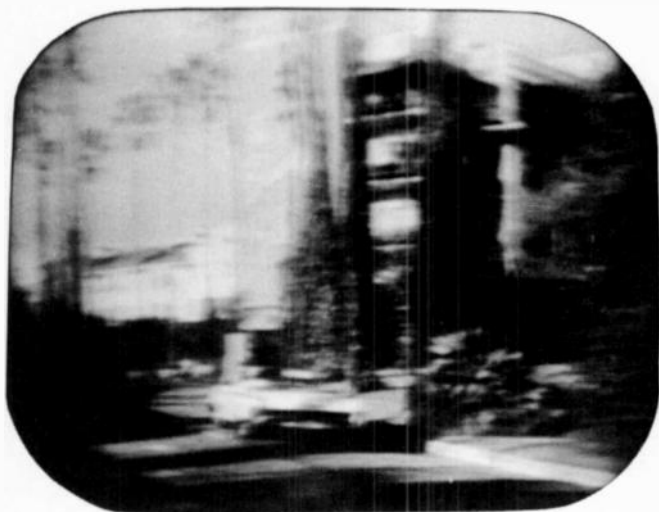
Fig. 506. Poor video amplifier low-frequency response is characterized by picture smear.
