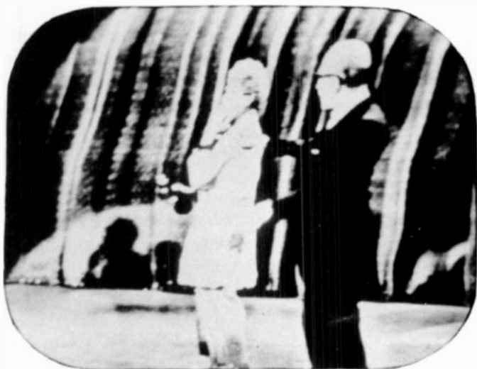
Fig. 411. Excessive signal voltage at amplifier inputs may result in too much contrast and picture bending. An extreme condition may result in an almost blank raster.
