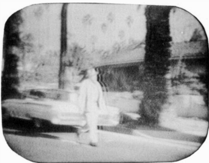
Fig. 507. The effects of overpeaking.
