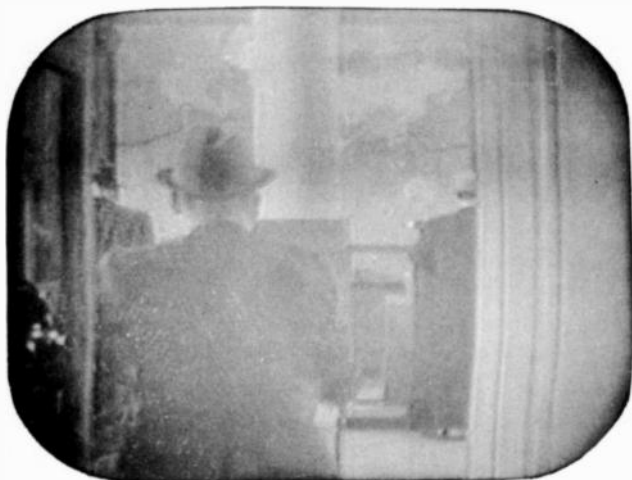
Fig. 505. Video if, detector or video amplifier trouble is indicated if a weak washed-out picture has no snow.
