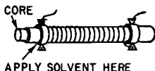
Fig. S-6. If the ferrite core is cemented into position, a few drops of solvent will loosen it enough to permit core adjustment.
