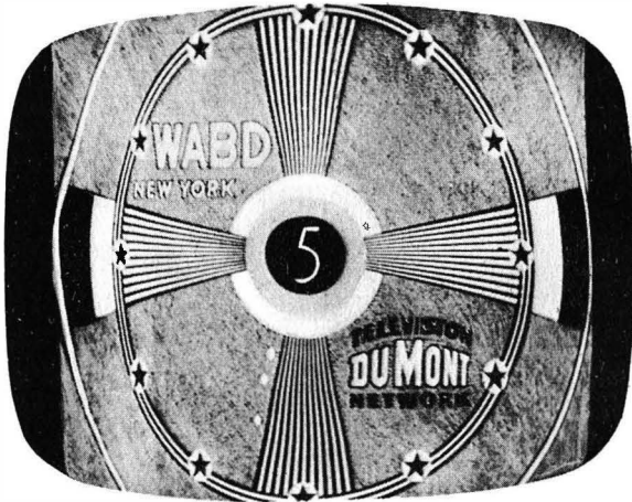
Fig. 305. Photo of test pattern indicates insufficient width.
