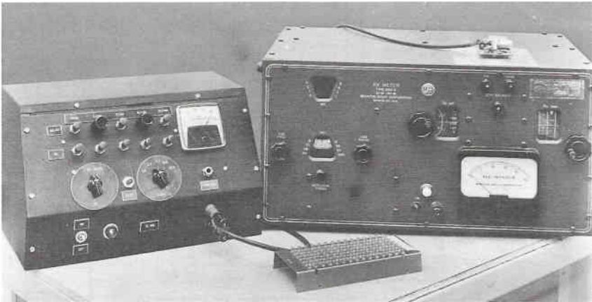
PHOTOGRAPH OF CAPACITY TEST SET UP
