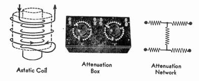
attenuation equalizer.—A device which increases the transmission loss at certain frequencies so that the loss for all transmitted frequencies within a certain range is made substantially the same. Frequencies originally over-emphasized are reduced in amplitude to equal all other frequencies. A system of inductances, capacities and resistances which attenuates certain frequencies.
