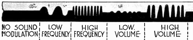
FIG. 4.—Changes in Variable Area Sound Track.
