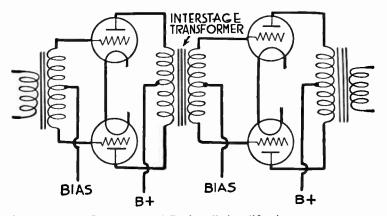
Fig. 12.-Dual Push-pull Amplification.
