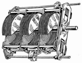
A Ganged Condenser for Tuning Three Circuits.
