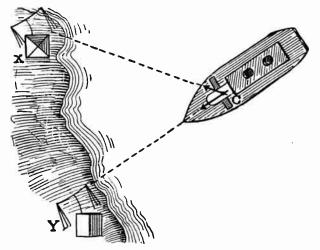
FIG. 2.-Determining Ship's Position with Radio Compass.
