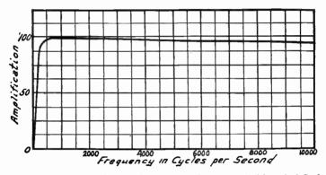
F10, 4.--Curve for Good Audio Transformer Drawn on Arithmetical Scale
