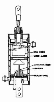
FIG. 3.—A General Electric Sealed Ignitron Having Two Ignitors and an Auxiliary Anode.
