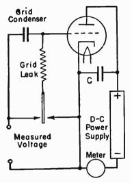
FIG. 2.—Grid Leak Detector Used as VT Voltmeter.
