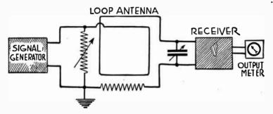
FIG. 12.-Method of Measuring Field Intensity.
