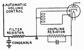
FIG. 3.—Double-diode in Automatic Volume Control.
