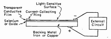
FIG. 1.—Principal Parts of Barrier Layer Photocells.
