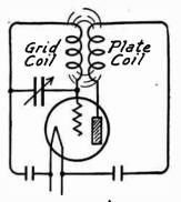
Fro. 2.—Feedback from Plate Circuit to Grid Circuit Causing Regeneration.
