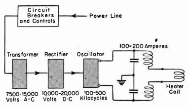
FIG. 5.—Principal Parts of an Induction Heating System.
