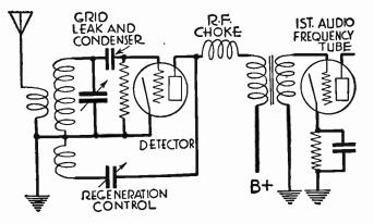
FIG. 4.—Regenerative Detector for Short Wave Reception
