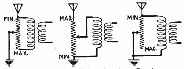
FIG. 13.—Antenna Circuit Volume Controls for Transformers.
