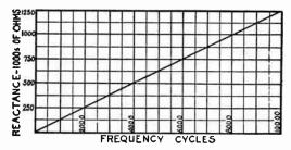
Fig. 5.—Frequency Effect on Inductive Reactance.
