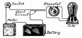
FIG. 2.--Testing for Short Circuit with Voltmeter.
