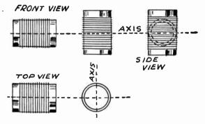
Relative Coil Positions for Minimum Coupling.
