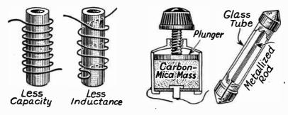
FIG. 1.—Space Winding and Non-inductive Winding of Resistors.
