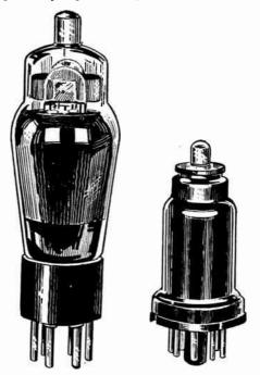
FIG. 4.—Glass Envelope Tube and Metal Type Having Generally Similar Performance.
