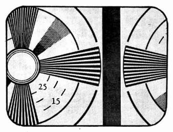
FIG. 36.-Effect of Wrong Adjustment of Phase Control.
