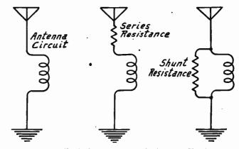
FIG. 2.--Equivalent Resistances in Antenna Circuit.
