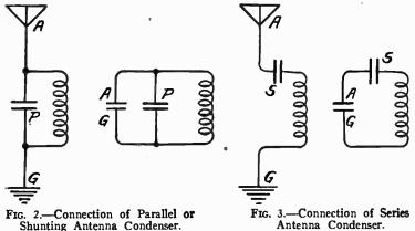
other. Any two condensers in series have a combined capacity less than the capacity of either one alone, therefore this lessened capacity used with the coil allows resonance or tuning at higher frequencies or lower wavelengths.
