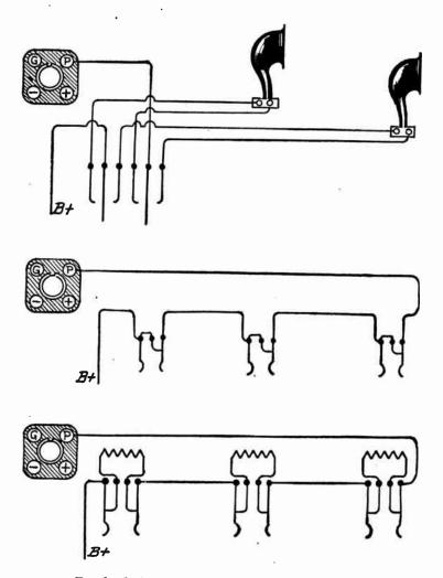
FIG. 6.-Jacks for Connection of Several Speakers.
