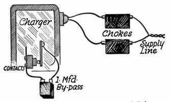
Fro. 5.-Handling Interference of Vibrators and Flashers.
