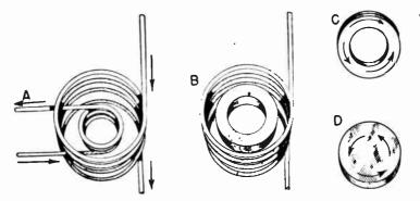
FIG. 1.-Elementary Principle of Induction Heating.
