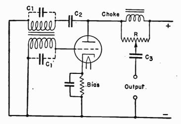
FIG. 1.-Feedback Type of Audio-frequency Oscillator.
