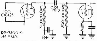
FIG. 5.-Typical Values for Resistance Coupling.
