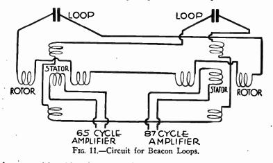
beacon with which are used three modulating frequencies; 65 cycles, 86.7 cycles and 108.3 cycles.
