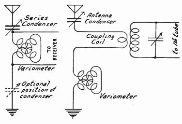
FIG. 4.—Variometer and Series Condenser for Antenna.
