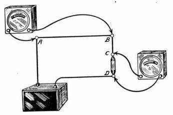
FIG. 1.—Principle of Testing for Open Circuits.
