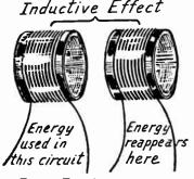
Energy Transfer by Electromagnetic Induction. If the induction is brought about by the magnetic field around a conductor or coil, the voltage and current which are induced may be set up either in the conductor or coil having the field or in any other nearby conductor or circuit. If the induced voltage is in the same conductor whose field causes the induction, the action is called selfinduction. If the voltage is induced in a nearby circuit the action is called mutual-induction.
