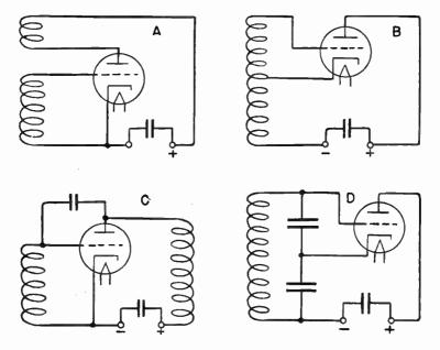
FIG. 2.-Methods of Providing Feedback.
