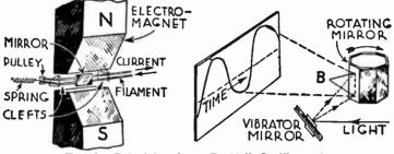
FIG. 2.—Principle of the Duddell Oscillograph.
