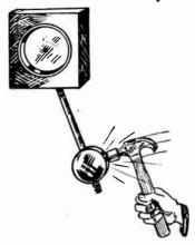
Fig. 3.—Mechanical Resonance Between Pendulum and Hammer. As the frequency is lowered, either the inductance, the capacity of both must be increased to maintain resonance. If the frequency is increased, then the capacity, the inductance, or both must be decreased to maintain resonance. In other words, the greater the frequency the less must be the capacity and inductance and the lower the frequency the greater must be the capacity and inductance.
