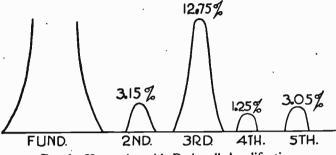
FIG. 6.—Harmonics with Push-pull Amplification.
