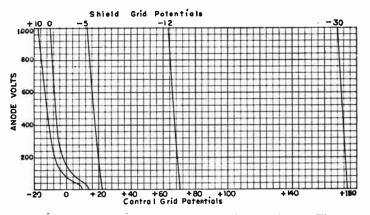
FIG. 3.-Control Grid Breakdown Potentials of Four-element Thyratron.
