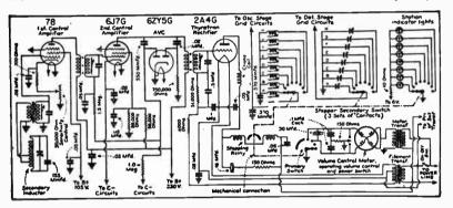
FIG. 9.—Philco Mystery Control Amplifier and Station Selector Switching Arrangement.
