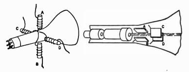
Fig. 2.—Electromagnetic Deflection of the Electron Beam.
