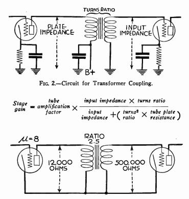
FIG. 3.-Simplified Diagram of Transformer Coupling.
