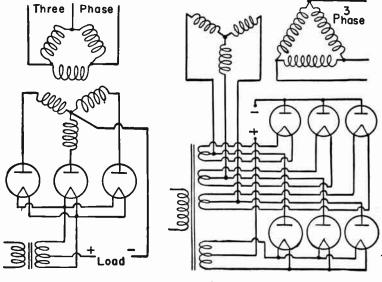
FIG. 1.—Polyphase Half-wave Rectifier.
