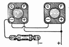
FIG. 2.—Single Filament Resistor for Two Tubes.
