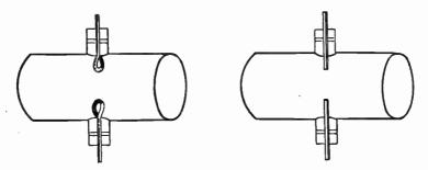
FIG. 2.-Energy Transfer Probes for Cavity Resonator.
