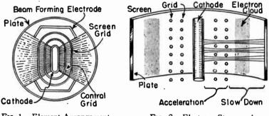
FIG. 1.—Element Arrangement in Beam Power Tube.
