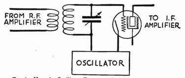
FIG. 4.-How the Oscillator Frequency Is Added to the Carrier.
