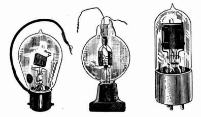
FIG. 1.-Early Experimental Types of Vacuum Tubes
