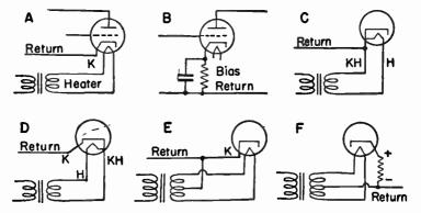
FIG. 2.—Returns for Heater-cathode Type Tubes.
