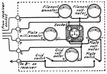
FIG. 8.—Receiver Tester with Attached Meters.
