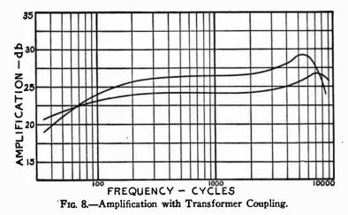
rent is increased by this resonance effect at and near one particular frequency and the amplification shows a sudden rise and fall around this frequency.
