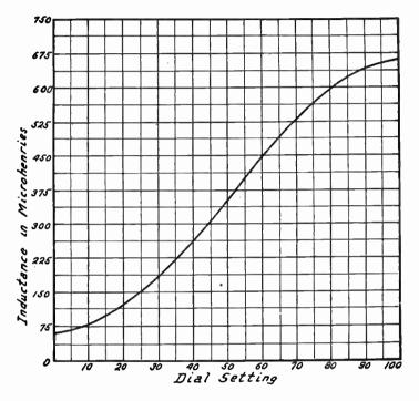
F10. 5.—Change of Inductance with Rotation of Variometer Rotor.
