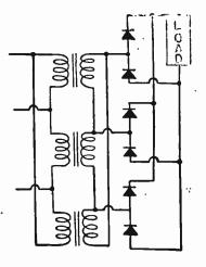
FIG. 4.—Six Elements with Center-tapped Transformer.
