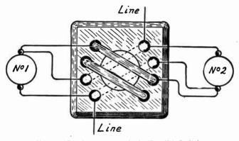
FIG. 1.-Special Form of Series-Parallel Switch.
