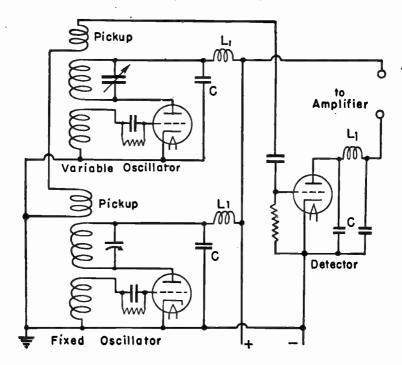
FIG. 1.—Circuits of a Beat Frequency Oscillator.
