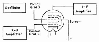
FIG. 26.—Connections for a Pentagrid Mixer.
