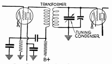
FIG. 1.—Transformer Coupling for Radio Frequencies.
