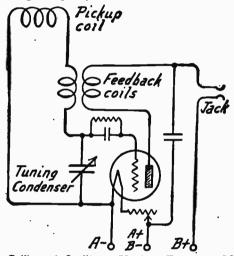
Fr. 5.—Calibrated Oscillator Used as Frequency Meter by Heterodyning with Frequency to Be Measured.
