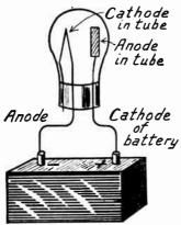
**ELECTRODE.**—Either one of the terminals of an electric source is called an electrode. The terminal, connection or conductor through which electric current or an electron stream enters or leaves anything is called an electrode. The terminal through which the current enters is called the anode, the terminal through which the current leaves being called the cathode. See Anode and Cathode.
