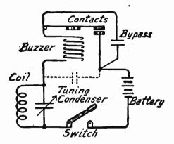
Oscillator Circuit Excited by Buzzer.
