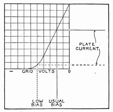
FIG. 5.-Biasing Points on Characteristic Curve.
