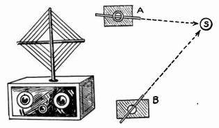
FIG. 1,-Elementary Principle of Radio Compass.
