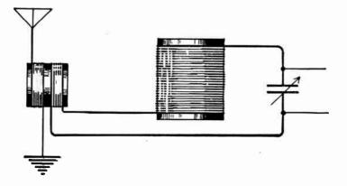
FIG. 2.—Separate Coupling Coil for Antenna Circuit.
