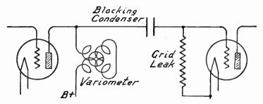
FIG, 1.--Tuned Impedance Coupling with Variometer.
