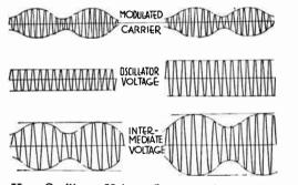
FIG. 12.-How Oscillator Voltage Increases Intermediate Voltage.
