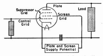
FIG. 3.-Typical Connections for Pentode Power Amplifier.
