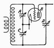
FIG. 7.—The Isofarad Method of Balancing.
