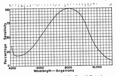
FIG. 4.-Wavelength Sensitivity of One Type of Phototube.
