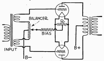
Fig. 8.—Equalizing Plate Currents in Push-pull Tubes.
