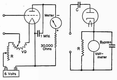
FIG. 5.—Circuit for Moullin Type VT Voltmeter. Fig. 6.—Diode Used for a VT Voltmeter.
