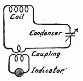
FIG. 2.—Frequency Meter with Coupled Indicator Circuit.
