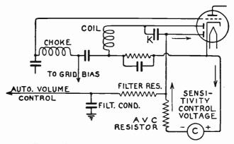
FIG. 5.—Sensitivity Control with Double-diode.
