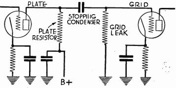
FIG. 1.-Resistance-capacity Coupled Amplifier.
