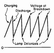
FIG. 5.—Output Wave Form of Neon Oscillator.
