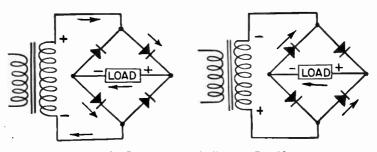
FIG. 6.-Bridge Type Full-wave Rectifier.
