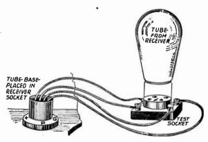
FIG. 7.-Tester Connection To Receiver.
