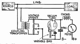
FIG. 2.-Vacuum Tube Type of Volume Indicator.
