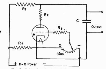
FIG. 6.-Relaxation Oscillator Using Thyratron Tube.
