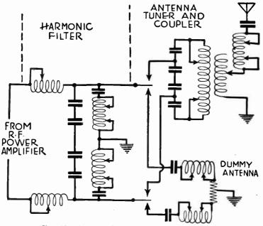
FIG. 10.—Antenna System and Harmonic Filter.
