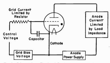
FIG. 2.-Grid and Plate Circuits of Gas-filled or Vapor-filled Triode.
