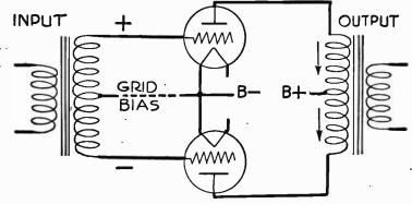
FIG. 1.--Elementary Push-pull Circuit.
