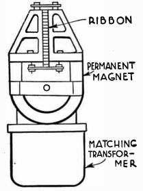
Fig. 1.-Constructional Details of Velocity Microphone.
