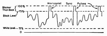
FIG. 7.—Horizontal Sync Pulses During Blanking Intervals.
