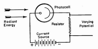
FIG. 3.-The Basic Phototube Circuit.
