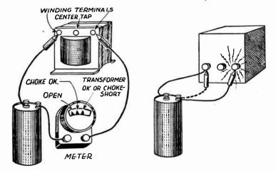
FIG. 14.—Test for Open Circuit or FIG. 15.—Test for Short Circuited Short in Transformer or Choke. Transformer Winding.
