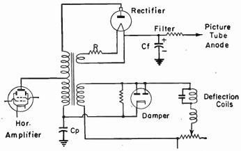
FIG. 37.—Flyback Type of High-voltage Supply.
