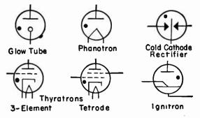
Fig. 1.—Symbols for Gas-filled Tubes.
