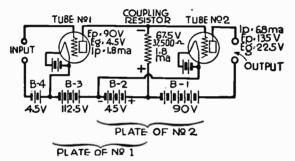
Fig. 1.-Simple Form of Direct Coupled Amplifier.
