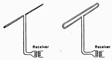
FIG. 2.—Connections to receiver input from a single straight dipole and from a folded dipole.
