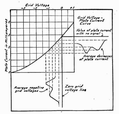
fIG. 3.—Action of the Grid Leak Detector. Variations of grid voltage cause corresponding variations of plate current, the latter decreasing in value as detection takes place.
