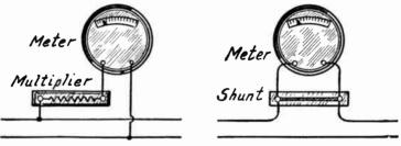
FIG. 3.—Multiplier Used with Voltmeter.
