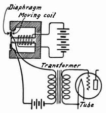
FIG. 4.—Moving Coil Microphone.
