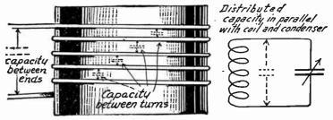
Distributed Capacity and Its Effect in a Coil.
