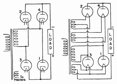
FIG. 7.-Four Tubes in Full-wave Bridge Circuit.
