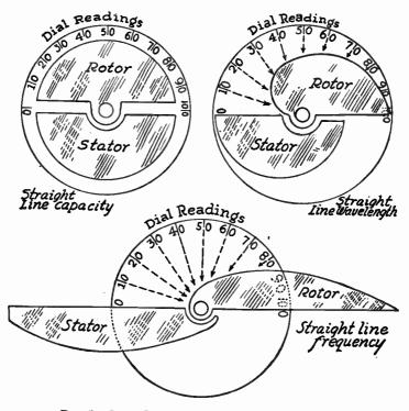
FIG. 5.-Basic Forms of Condenser Rotor Plates.
