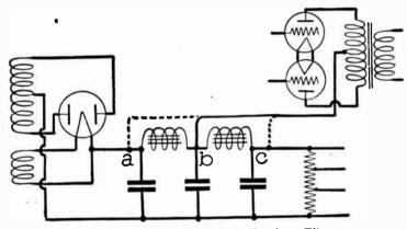
FIG. 7.--Connections of Plate Circuit to Filter.
