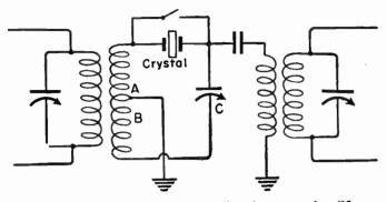
FIG. 27.-Crystal Used in Intermediate-frequency Amplifier.
