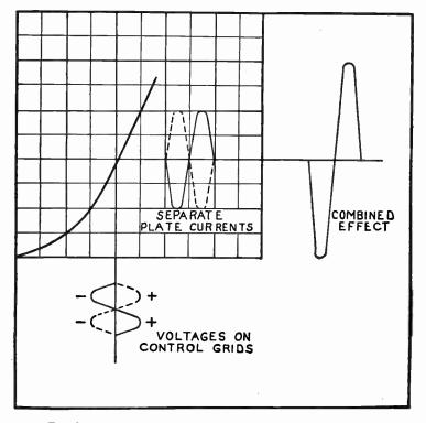
FIG. 2.-Combining Plate Currents in Push-pull Amplifier.
