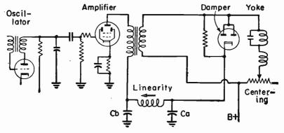
FIG. 28.—Sweep Circuits for Magnetic Deflection.
