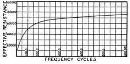
FIG. 6.—Frequency Effect on Apparent Resistance.
