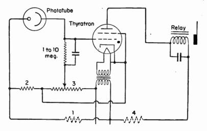
FIG. 12.—Phototube and Thyratron for Pull-in of Relay upon Increase of Light.
