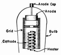
FIG. 1.—Arrangement of Elements in One Style of Thyratron.
