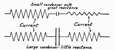
FIG. 4.-Effect of Large and Small Filter Condensers on Alternating Currents.
