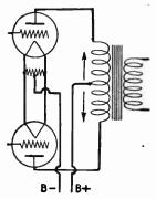
FIG. 3.—D.C. In Output Transformer Primary. produce proportionate changes in magnetic flux rather than being cut off by a saturation bend in the magnetization curve of the iron.
