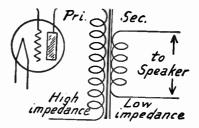
FIG. 2.-Matching Impedances with Special Transformer.
