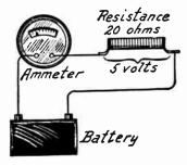
FIG. 2.—Determining Voltage Drop with Ohm's Law.
