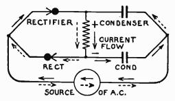
Fig. 2.—Equivalent Circuit for Voltage Doubler.
