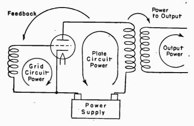
FIG. 1.—Principle of the Feedback Oscillator.
