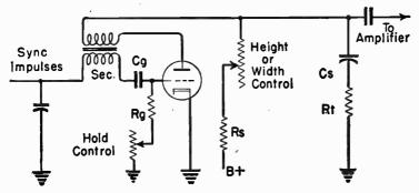
FIG. 26.-Blocking Oscillator Used in Sweep Circuits.
