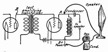
FIG. 4.--First Test of Audio Amplifier with Choke Speaker Coupling.
