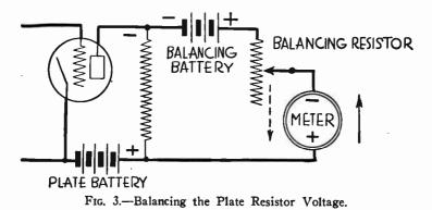
It is possible to construct a direct current amplifier to operate without batteries by taking all plate voltages and biasing voltages from suitable taps on a single voltage divider. This method is similar to that described for a direct coupled amplifier under
