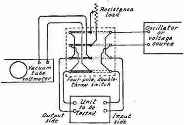
FIG. 8.—Checking Amplifier Unit with VT Voltmeter.
