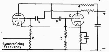
FIG. 3.—Circuit of Multivibrator Oscillator.
