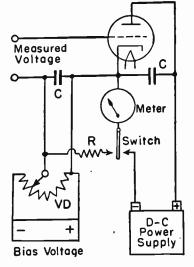
FIG. 3.—Slide Back Instrument Using Two Meters.
