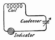
FIG. 1.—The Simplest Frequency Meter Circuit.
