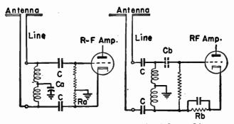
FIG. 17.-Untuned Input Circuits for 300-ohm Lines.
