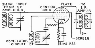
FIG. 25.—Complete Pentagrid Converter Connections.
