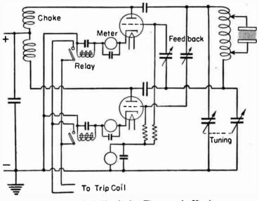
FIG. 3.-Typical Circuit for Electrostatic Heating.
