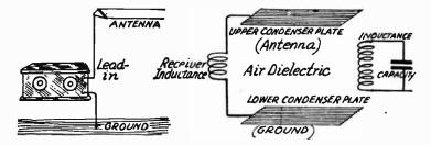
FIG. 2.-The Principle of the Capacity Antenna.
