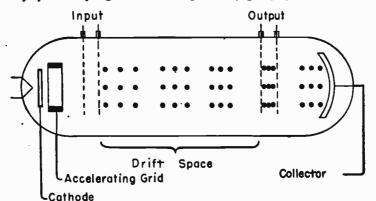
FIG. 3.—The Drift Space Method of Changing Velocity Modulation to Intensity Modulation.
