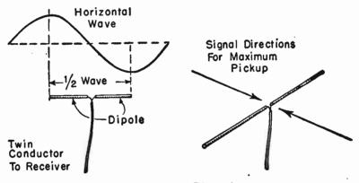
FIG. 14.-Half-wave Dipole Antenna.
