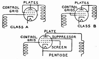
FIG. 6.—Connections for Voltage-amplifier Pentodes.
