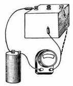
Fig. 16.—Test for Capacity, Short or Open Circuit on Condenser.
