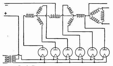
FIG. 3.—Three-phase Double-Y Parallel Rectifier.
