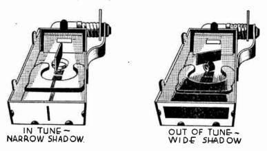
FIG. 12.-Iron Vane Tuning Meter
