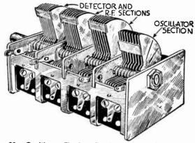
FIG. 20.-Oscillator Tuning Condenser with Special Plates.
