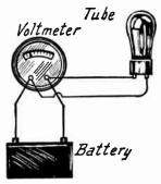
FIG. 3.—Determining Current with Ohm's Law.
