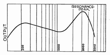
FREQUENCY~ CYCLES FIG. 9.—Output of Record and Pickup Working Together.
