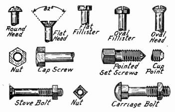
Screws and Bolts Used in Construction Work.
