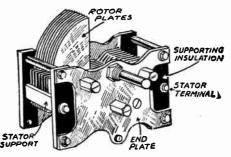
FIG. 3.—Terminal Positions Considered in Condenser Design.
