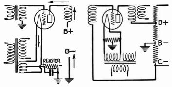
FIG. 7.—Biasing for Filament Tubes.
