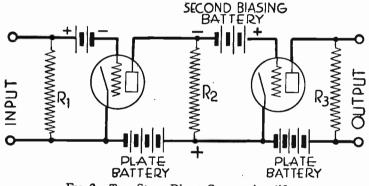
Fig. 2 .-- Two-Stage Direct Current Amplifier.
