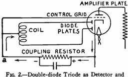
IG. 2.—Double-diode Triode as Detector and Amplifier.
