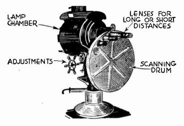
FIG. 6.-Television Scanner Employing an Arc Lamp.
