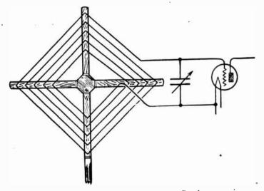
Connections from Spiral Loop to Receiver.
