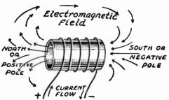
FIC. 2.-Electromagnetic Field around a Solenoid or Coil.
