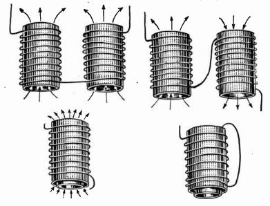
FIG. 3.—Coils Working Together to Add Their Inductances as in a Variometer. Ket. 4.—Coils Opposing Each Other to Destroy Inductance as in a Variometer.
