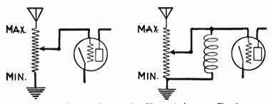
FIG. 14.-Volume Controls for Untuned Antenna Circuits.
