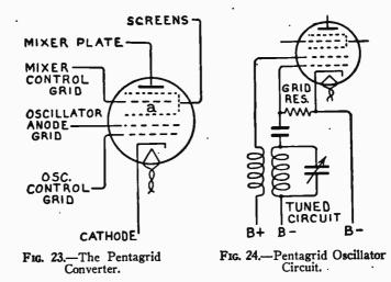
Next in the order of the grids, moving away from the cathode, comes one part of the screen. Then comes the control grid for the mixer, and just outside of it the second or outer part of the screen. Both parts of the screen are connected to the same prong on the tube base. The final electrode is the regular plate which acts as the plate for the mixer section.
