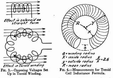
when the outside radius equals 1.7 times the inside radius, but the highest ratio of inductance to resistance is obtained with an outside radius equal to 2.6 times the inside radius. The diameter of the turns should be small and the number of turns large in order to keep the overall size within reasonable limits.
