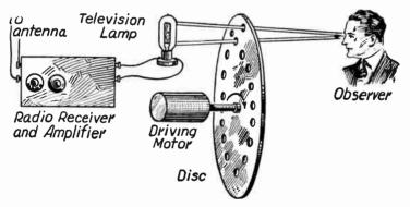
FIG. 2.-Nipkow Disc Reproduction at Television Receiver.
