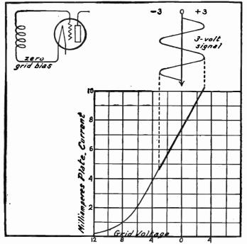
FIG. 1.-Effect of Zero Grid Bias, Distortion.
