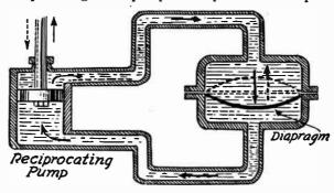
FIG. 5.-Hydraulic Explanation of Condenser Action.
