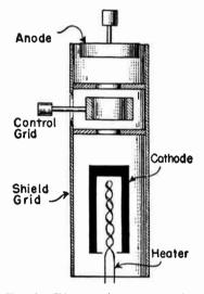
FIG. 1.—Element Arrangement in Heavy-duty Four-element Thyratron.
