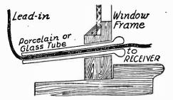
Antenna Lead-in Carried Through Tube.
