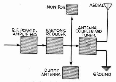
FIG. 3.—High Power Equipment Used at Transmitter.
