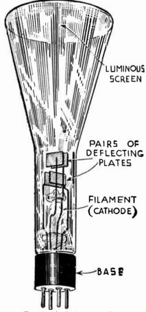
FIG. 1.-A Cathode-ray Tube.
