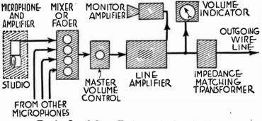
FIG. 1.-Speech Input Equipment for Broadcasting.
