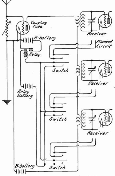
Connections for Operating Several Receivers from One Antenna.
