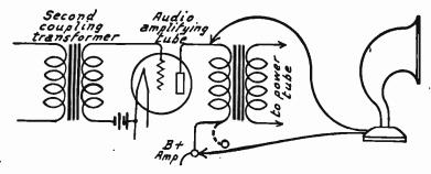
FIG. 5.-Second Test on Audio Amplifier.
