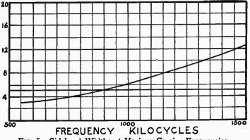
FIG. 5.—Sideband Widths at Various Carrier Frequencies.
