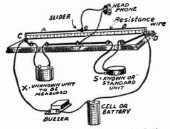
FIG. 5 .- Practical Form of Slide Wire Bridge.
