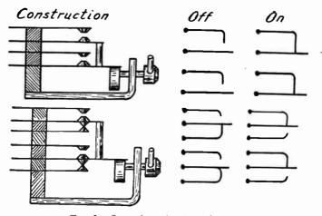
FIG. 2.—Operation of a Jack Switch.
