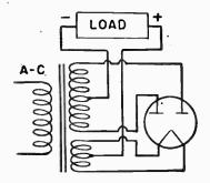
FIG. 3.—Full-wave Filamentcathode Rectifier.
