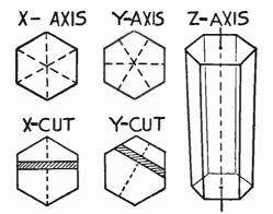
FIG. 2.-Methods of Cutting Quartz Plates.
