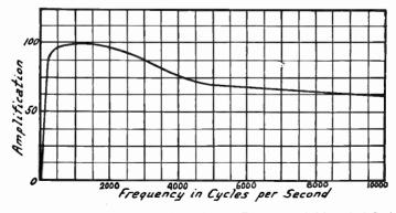
F10. 5.--Curve for Poor Audio Transformer Drawn on Arithmetical Scale.
