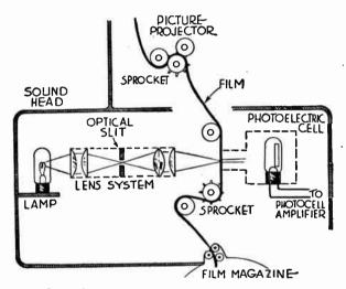
FIG. 12.-Principal Parts of a Sound Head.
