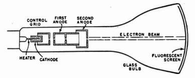
FIG. 1.—Principal Parts of a Cathode-ray Tube.
