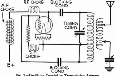
FIG. 3.-Oscillator Coupled to Transmitting Antenna.
