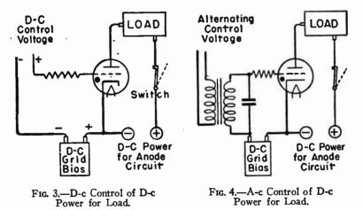
the cathode. Current will stop every time that the anode potential drops back to zero, which will be at the end of each positive halfcycle. With a-c supply for the anode circuit it is not necessary to provide a switch for opening the anode circuit when current is to
