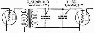
FIG. 7.-Capacities in Transformer Secondary Circuit.
