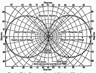
FIG. 4.—Polar Response Curve of Velocity Microphone.
