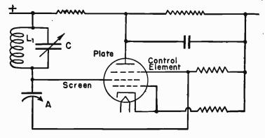
FIG. 8.—Negative Transconductance Oscillator.
