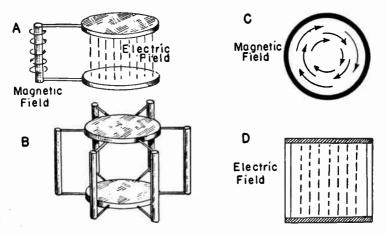
FIG. 1.—Principle of the Cavity Resonator.
