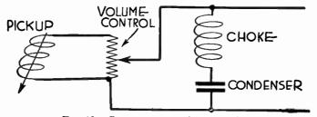
FIG. 10.-Connections for Scratch Filter.
