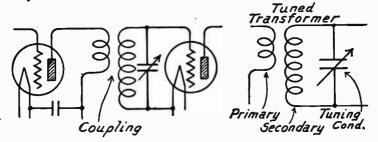
FIG. 1.-Tuned Radio Frequency Transformer Used as Coupler.
