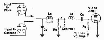
FIG. 19.-Typical Connections for Video Detectors.
