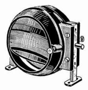
FIG. 1.---Variometer with Spherical Windings.
