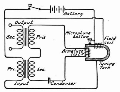
FIG. 2.-Tuning Fork Audio Oscillator.
