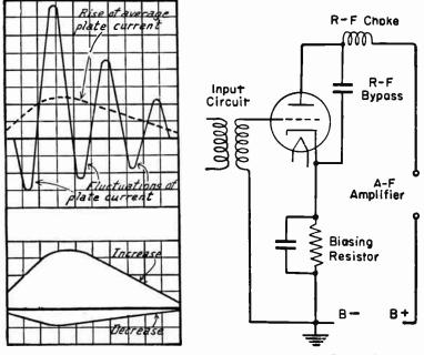
FIG. 2.—Current Change During Plate Current Detection.
