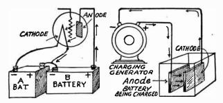
Anodes and Cathodes in Electric Circuits.
