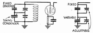
FIG. 21.—Arrangement of Capacities for Oscillator Tuning
