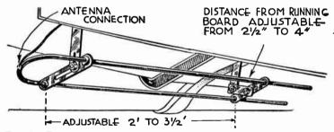
Frs. 4.—Folded Doublet or Di-pole Automobile Antenna Installed under Running Board.
