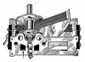
FIG. 6.-Modified Straight Line Frequency Condenser.
