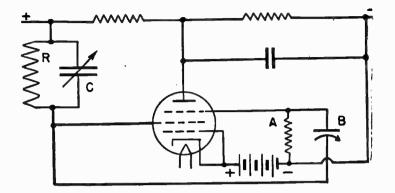
FIG. 9.—Negative Resistance Oscillator Employing Resistancecapacity Circuits.
