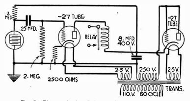
FIG. 7.-Photoconductive Cell Amplifier for Power Line,
