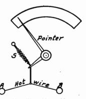
FIG. 7.-Hot Wire Meter Movement.
