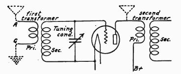
FIG. 1.—Antenna Connections for Testing Radio Stages.
