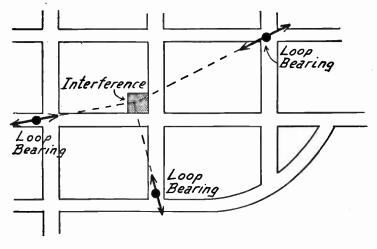
FIG. 2.-Locating Interference with Portable Receiver.
