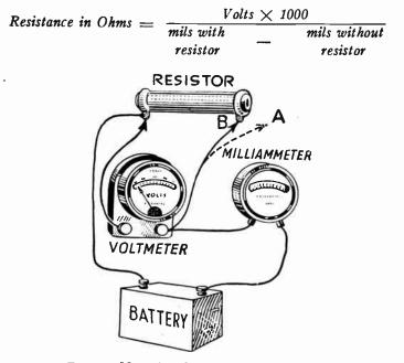
FIG. 18.-Measuring the Resistance of a Resistor.
