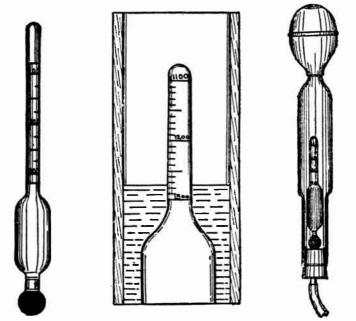
FIG. 3.—A Hydrometer, Its Scale, and a Hydrometer Syringe for Storage Battery Tests.
