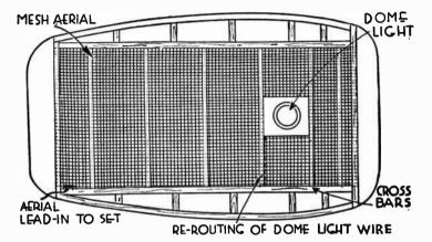
FIG. 2.—Construction of Copper Mesh Roof Type Automobile Anténna.
