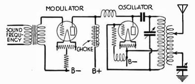
FIG. 6.—Connection of Modulator to Oscillator.
