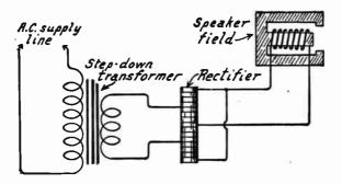
FIG. 7.-Rectifier Field Current Supply.
