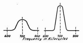
FIG. 3.-Effect of Regeneration on Signal.
