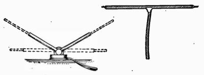
FIG. 15.—Two types of indoor antennas.
