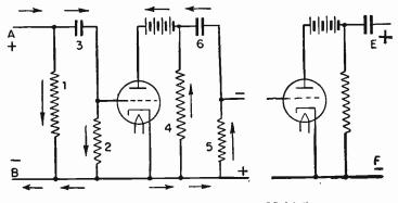
FIG. 2.—Operating Principle of the Multivibrator.
