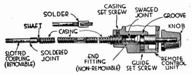
Fis. 5.—Construction at "Dental Cable" Flexible Control Shaft.
