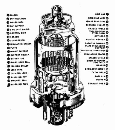
FIG. 1.-Construction of One RCA Type of Voltage-amplifier Pentode.
