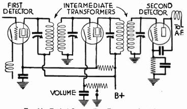
FIG. 14.-Typical Intermediate Frequency Amplifier.
