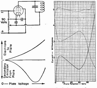
FIG. 6.—Connections and Action of Dynatron Oscillator.
