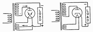
FIG. 1.-Tubes Used as Half-wave Rectifiers.
