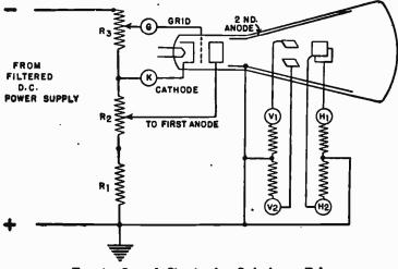
FIG. 4.-Control Circuits for Cathode-ray Tube.
