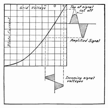
FIG. 2.--Distortion Caused by Zero Grid Bias.
