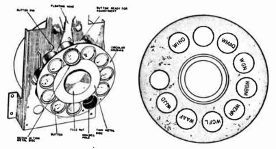
FIG. 6.—Telephone Type Tuning Dial.
