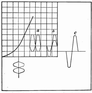
FIG. 4.—Balancing Unequal Changes of Plate Current.
