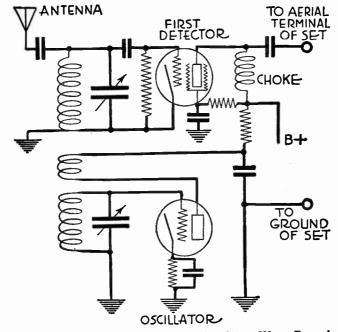
FIG. 6.-Superheterodyne Converter for Short Wave Reception
