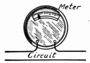
FIG. 1.—Ammeter in Series with Circuit.
