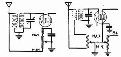
FIG. 20.—Dual Control with One FIG. 21.—Twin Control for Antenna Potentiometer. and Screen Voltage.
