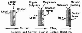
Elements and Current Flow in Contact Rectiners.
