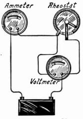
FIG. 1.—Determining Rheostat Resistance with Ohm's Law.
