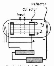
Fig. 1.—The Elements Employed for Velocity Modulation.
