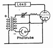
FIG. 10.—Phase-shift Control by Means of a Vacuum Triode Connected to a Bridge Rectifier.
