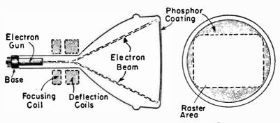
FIG. 5.—Television Picture Tube for Magnetic Deflection.
