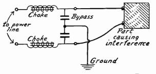
FIG. 8.—Interference Filter with Grounded Center Tap.
