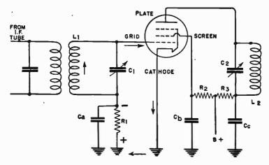
FIG. 3.—Connections for a Typical Limiter,
