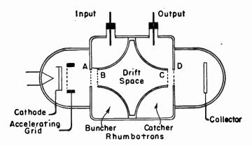
FIG. 1.—Arrangement of Elements in a Klystron.
