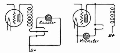
FIG. 4.-Meter Connections Made with Switches.
