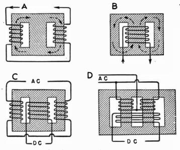
Windings of Saturable Reactors.
