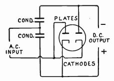
FIG. 1.-Voltage Doubler Connections.
