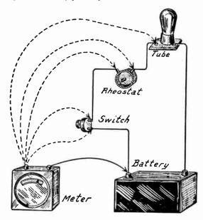
FIG. 2.-Testing Filament Circuit for Opens.
