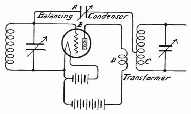
FIG. 2.-Neutrodyne Method of Balancing.
