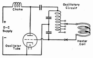
FIG. 2.-Simplified Circuit for Induction Heating.
