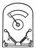
FIG. 6.—Thermocouple Meter.
