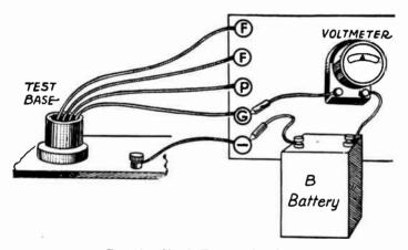
FIG. 10.-Circuit Tests on Receiver.
