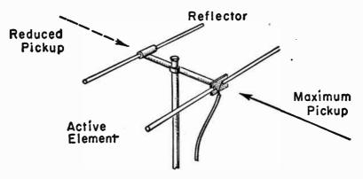
FIG. 15.—Half-wave Dipole with Reflector.
