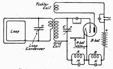
Circuits of Super-Regenerative Single Tube Receiver.
