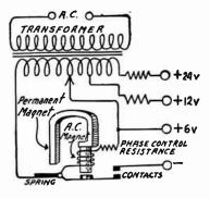
FIG. 2.—Half-wave Vibrating Rectifier.
