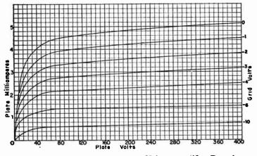
FIG. 4.—Plate Characteristics of a Voltage-amplifier Pentode.
