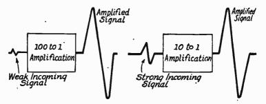
The Effect of Amplification on Signal Strength.
