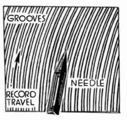
FIG. 2.—Unmodulated Record Grooves.
