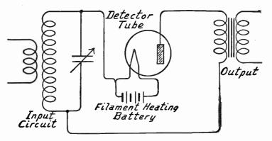
Elementary Principle of Diode Detector.
