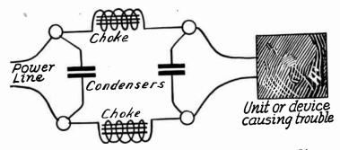
FIG. 7 .-- Filter Placed between Interfering Device and Power Line.
