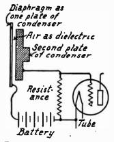
FIG 3.—Condenser Microphone.
