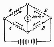
FIG. 5.-Balancing Principle of the Wheatstone Bridge.
