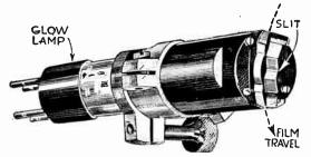
FIG. 10.-Glow Lamp Holder with Slit.
