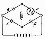
FIG. 8.—The Isofarad Balanced Circuit in Bridge Form.
