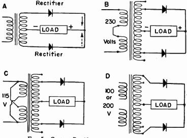
FIG. 5.-Contact Rectifiers in Full-wave Circuits.
