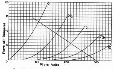
Load Line Used for Computing Voltage Amplification.
