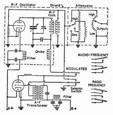
Modulated Oscillator or Signal Generator.
