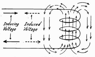
FIG. 1.-Effect of Self-Inductance in a Coil.
