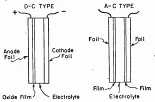
Elements Used in Electrolytic Condensers.
