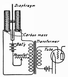
FIG. 2.—Double-button Carbon Microphone,
