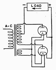
FIG. 1.—Two Filament-cathode Tubes in Full-wave Rectifier.
