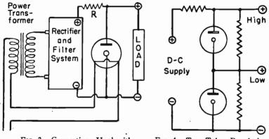
FIG. 3.—Connections Used with Single Regulator Tube.
