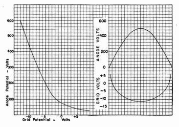
FIG. 1.—Average Breakdown Potentials for a Gas-filled Tube. Anode Volts for Breakdown.
