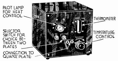
FIG. 4.—Temperature Control Box for Quartz Plates.
