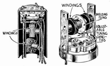
FIG. 16.--Construction of Intermediate Frequency Transformers.
