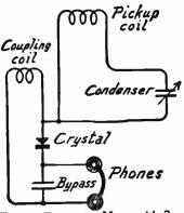
Fig. 3.—Inductively Coupled Indicator Fig. 4.—Frequency Meter with Spe-Circuit for Frequency Meter. cial Coupling for Indicator. Circuit for Frequency Meter.
