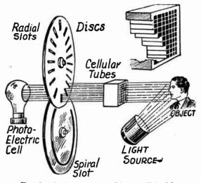
FIG. 3.-Action of Baird Discs in Television.
