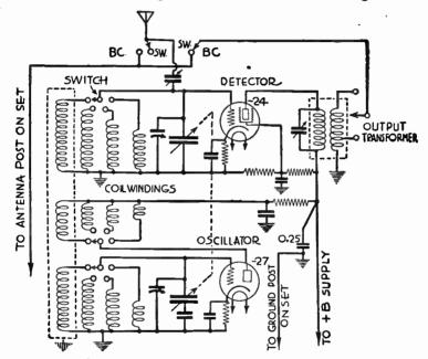
FIG. 8.—Circuit Diagram of Superheterodyne Converter
