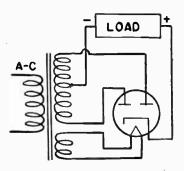
FIG. 4.—Full-wave Heatercathode Rectifier.
