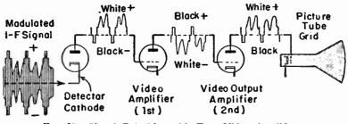
FIG. 21.—Signal Polarities with Two Video Amplifiers.
