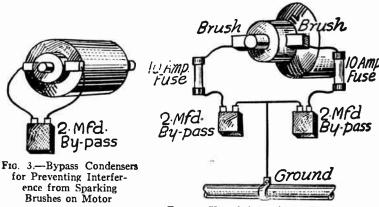
FIG. 4.—Use of Ground and Fuses on Interference Filter.
