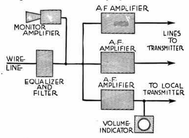
FIG. 5.—Bridging System Used in Chain Broadcasting.
