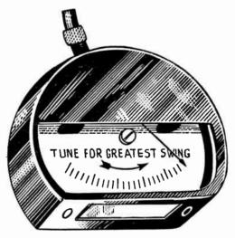
FIG. 11 .- Reversed Scale Meter Tuning Indicator
