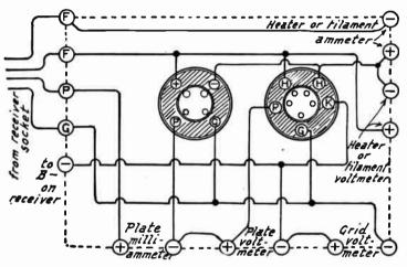
FIG. 9.-Test Board with Sockets.
