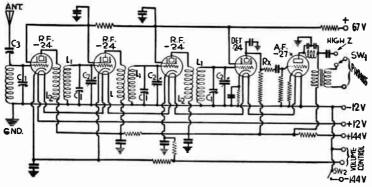
FIG. 15.—Circuits of Typical Airplane Receiver.
