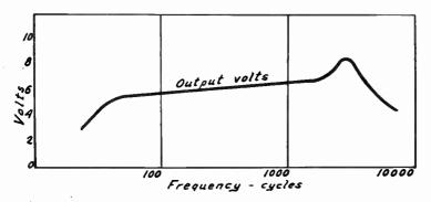
FIG. 5.-Result of Frequency Distortion in Amplifier.
