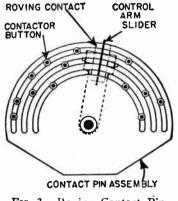
FIG. 3.—Roving Contact Pin Assembly.
