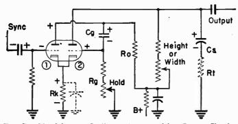
FIG. 27.-Multivibrator Oscillator for Television Sweep Circuits.
