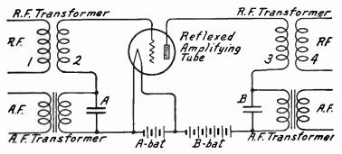
FIG. 2.-Circuits of Reflexed Amplifying Tube.
