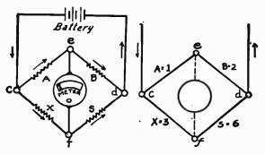
FIG. 1.—Principle of the FIG. 2.—Obtaining a Balance Wheatstone Bridge. in the Bridge.
