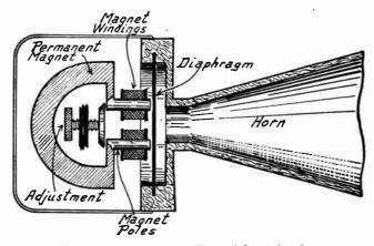
FIG. 1.-Electromagnetic Type of Loud Speaker.
