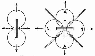
FIG. 4.—Radiation from Loop Antennas.
