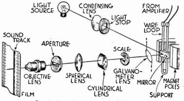
FIG. 5.—Variable Area System of Recording.
