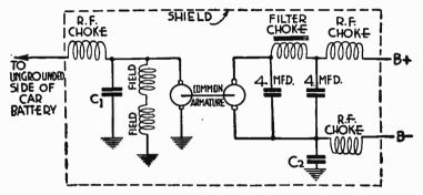
FIG. 6.—Circuit Diagram of Dynamotor Type Automobile "B" Supply. C<sub>1</sub> and C<sub>2</sub> Are .3 mfd.
