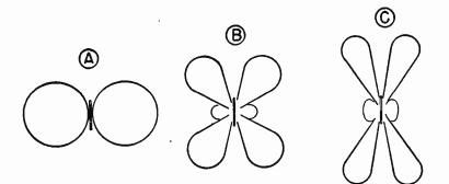
FIG. 7.—Changes of directional pattern of a straight dipole with increase of received frequency.
