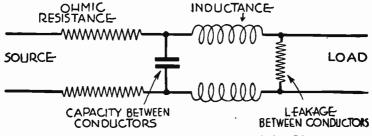
FIG. 4.-Electrical Elements of Transmission Line.
