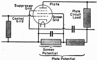
FIG. 2.-Typical Connections for Pentode Voltage Amplification.
