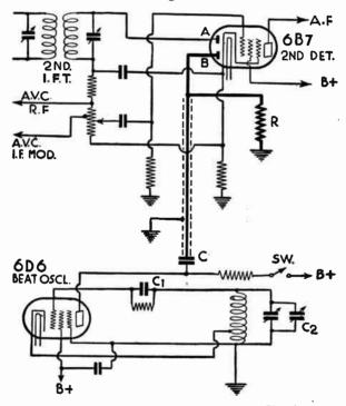
FIG. 10.—Beat Frequency Oscillator Circuit
