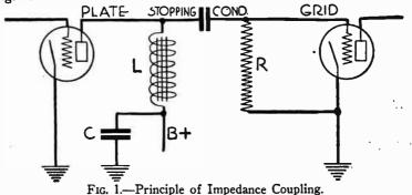
The plate circuit for audio frequency changes in the left hand tube includes impedance coil L, bypass condenser C and the ground connection to the cathode. The grid circuit of the right hand tube includes the stopping condenser, the coil L, bypass C and the ground connection to this tube's cathode. Thus the coil L is included both in the first plate circuit and the second grid circuit. Signal voltages developed across this impedance by the first tube are applied to the following grid circuit.
