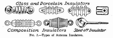
The far end of the antenna should be fitted with one or two of these insulators as in Fig. 1. To the far end of the insulator should be attached at least five to ten feet of strong galvanized wire or any other strong wire. This is used for making the mechanical connection to whatever post or other support is used.
