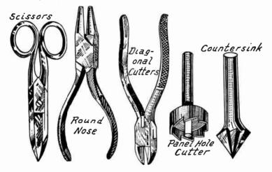
FIG. 2.—Pliers and Cutting Tools.
