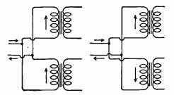
FIG. 11.-Connections of Transformers to Supply Line.
