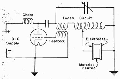
FIG. 1.—Simplified Circuit for Electrostatic Heating.
