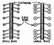
FIG. 2.—Control Grid Spacing in Variable-mu Tube.
