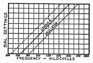
FIG. 5.-Relation of Oscillator and Carrier Frequencies.
