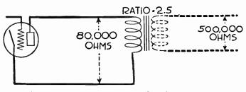
FIG. 4.-Secondary Load as Reflected in Primary.
