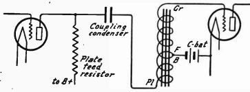
FIG. 11.-Parallel Feed with Resistor and Transformer.
