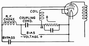
FIG. 4.-Double-diode Half-wave Detector.
