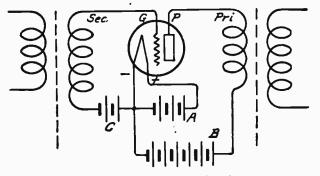
FIG. 6.—Circuits of Amplifying Stage.
