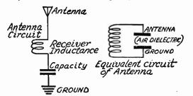
The Antenna Circuit and Its Electrical Equivalent.
