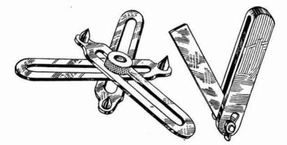
FIG. 1.—Adjustable Template and Adjustable Square.
