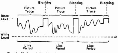
FIG. 6.-Horizontal Blanking Intervals Between Picture Signals.
