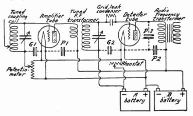
FIG. 2.—Bypass Condensers in a Receiver.
