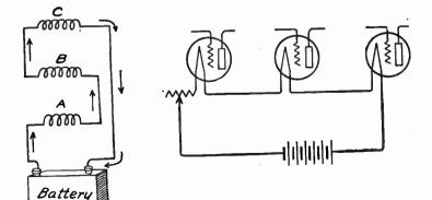
FIG. 1.—A Series Circuit.
