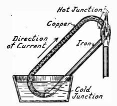
FIG. 1.--Principle of the Thermocouple.
