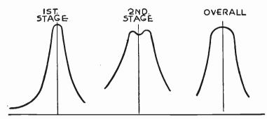
FIG. 15.-Resonance Curves for Intermediate Amplifier.
