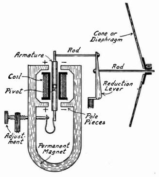
FIG. 2.-Balanced Armature Type of Loud Speaker.
