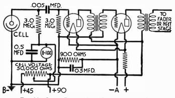
FIG. 14.—Sound Picture Amplifier with Phototube.
