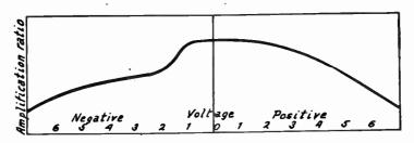
FIG. 7.-Variation of Amplification with Changes of Input Voltage.
