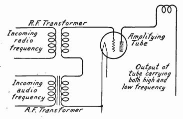
FIG. 1.-Effect of Reflexing on Amplifying Tube.
