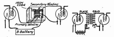
FIG. 1.-Transformer Coupling for Audio Frequency Amplifier.
