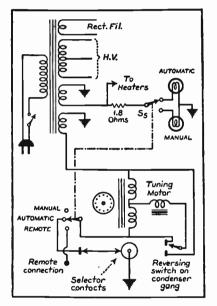
FIG. 2.-Electric Tuning Circuit.
