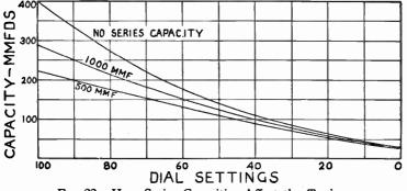
FIG. 22.-How Series Capacities Affect the Tuning.
