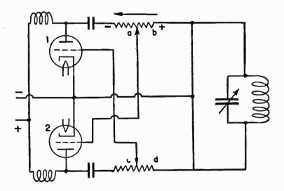
FIG. 10.-Negative Resistance Oscillator with Two Tubes.
