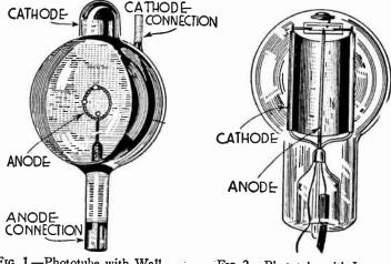
FIG. 1.—Phototube with Wall Type of Cathode.
