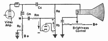
FIG. 24.-A Diode Used for Restoration of the D-c Component.
