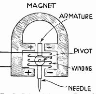
FIG. 6.—Sidewise Motion of Needle Point.
