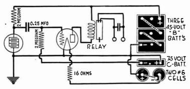
FIG. 6.—Photoconductive Cell Amplifier for Batteries.
