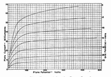
FIG. 1.—Plate Characteristics of a Power Pentode.
