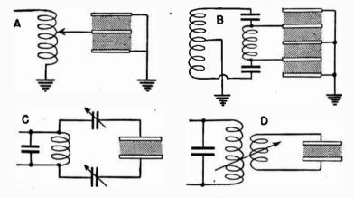
FIG. 2.-Electrode Arrangements for Electrostatic Heating.
