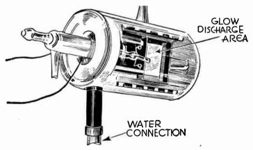
FIG. 7.-High Power Glow Lamp for Television.
