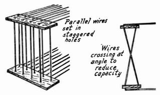
Arrangement of Wire on Loop Framework.
