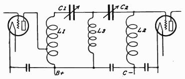
FIG. 7.-Circuit Arrangement of Vreeland Band Selector.
