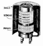
FIG. 2.-Shielded Radio Frequency Transformer.
