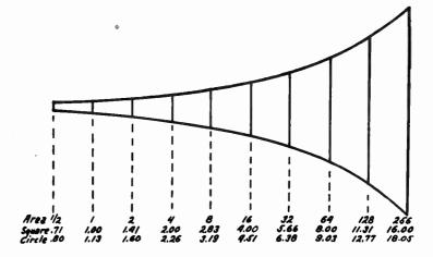
FIG. 3.-Design of Exponential Horn.
