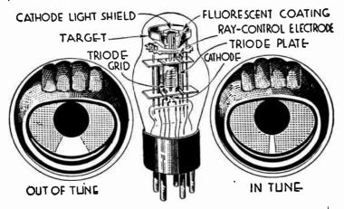
FIG. 13.—Cathode Ray Tuning Meter
