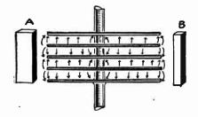
Frc. 2.-The Electrostatic Field Affecting Design of a Condenser.
