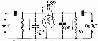
FIG. 7.-Tube Capacities Affecting Amplification.
