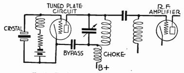
FIG. 3.-Circuit of Crystal Controlled Oscillator.
