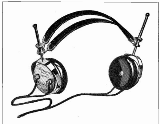
Fig. 101. This photo shows a pair of earphones or headphones as they are often called. Phones of this type are very useful for receiving weak signals that are not strong enough to operate a speaker, and also for testing radio devices and circuits.
