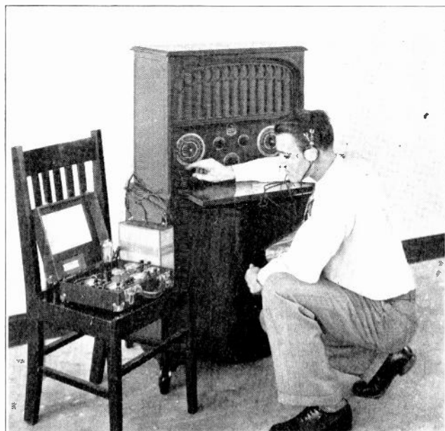
Fig. 123. This photograph shows a service man on the job with a set analyzer, making trouble tests on a radio receiver.
