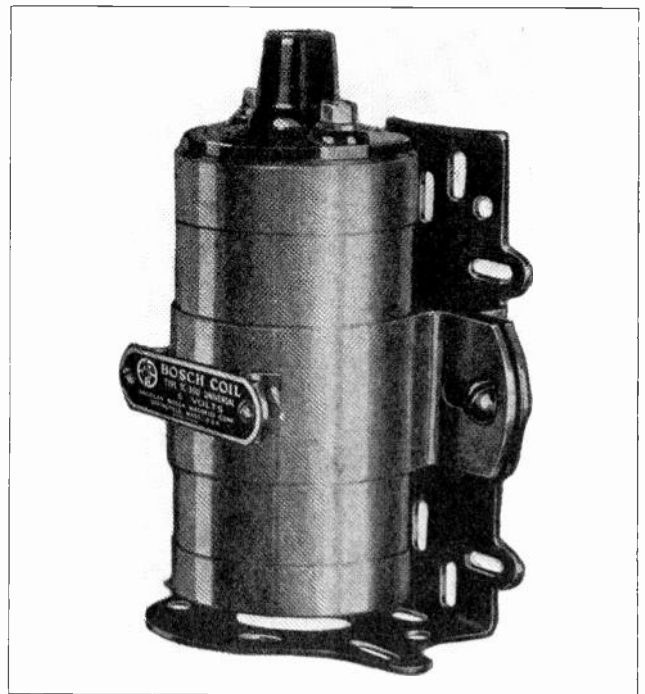
Fig. 22. High-tension ignition coil such as used for supplying high voltage impulses to the spark plugs on the ignition systems of automobiles. The heavily insulated bushing on the top of the coil is where the high voltage lead connects.
