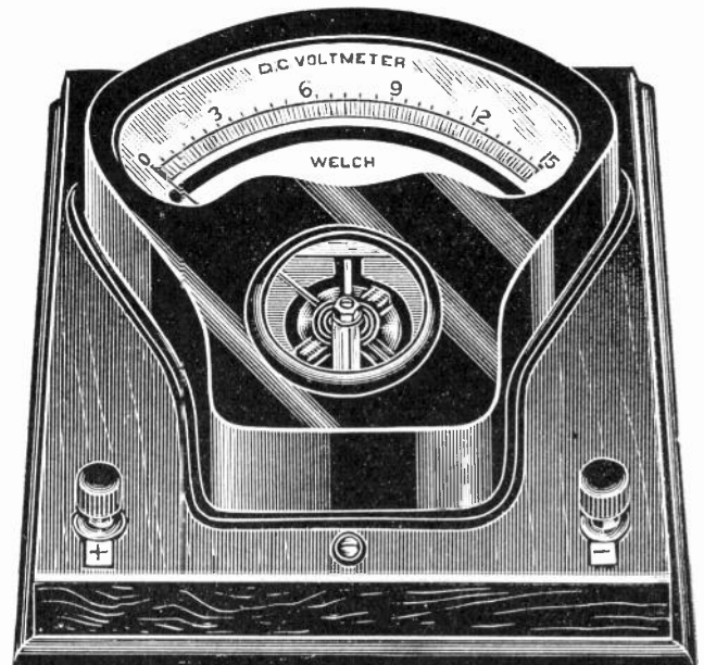
Fig. 4. Portable voltmeter used to measure electric pressures or voltages.
