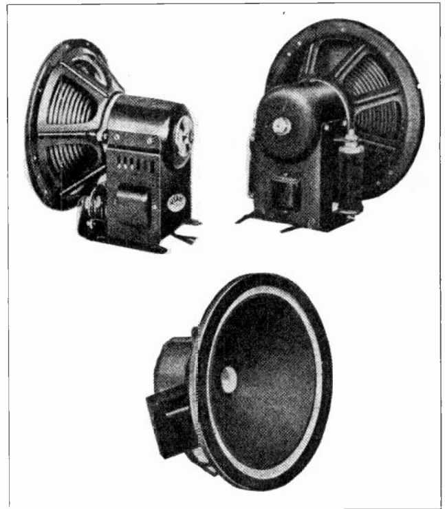
Fig. 108. This photo shows several views of dynamic speakers such as are very commonly used with modern radio receivers.
