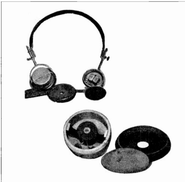
Fig. 102. The top photo shows a pair of phones with the cover and diaphragm removed from one to show the magnets, and below is shown an open view of a single large phone unit for use on a speaker horn.
