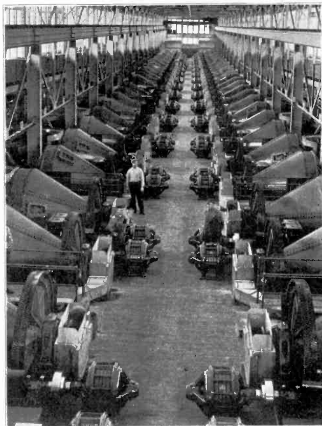
Fig. 475. This photo shows an installation of A. C. motors in a copper mill. Hundreds of thousands of motors in thousands of electrified factories and plants require the services of trained electrical maintenance men.
