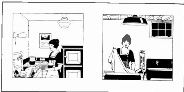
Fig. 251. At the left is shown the arrangement of ceiling unit and wall bracket light for kitchen. On the right a very efficient type of reflector for laundry rooms and basement lighting.
