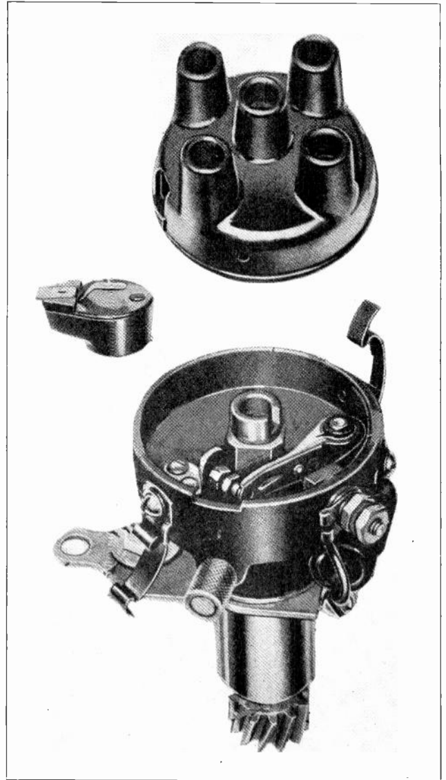
Fig. 33. This view shows a distributor with the high tension cap and rotor removed so that the primary breaker points and cam can be clearly seen in the distributor housing.
