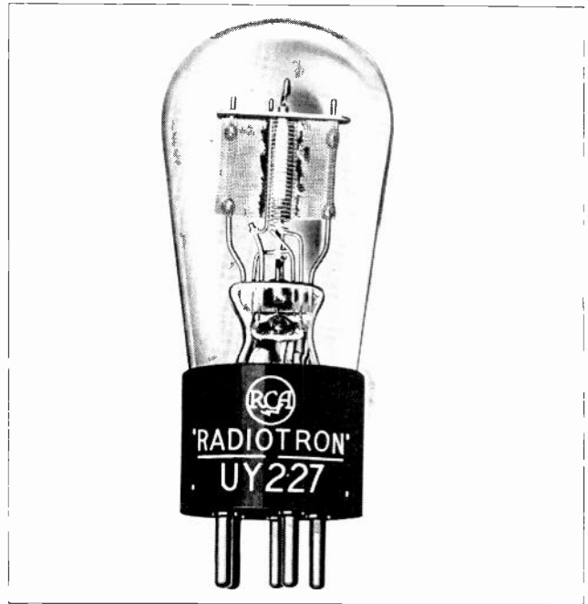
Fig. 61-A. Photograph of an A. C. heater-element vacuum tube with part of the plate removed to show the grid and the cathode inside of which the heater element or filament, is located. (Photo courtesy of R. C. A. Radiotron Co., Inc.)
