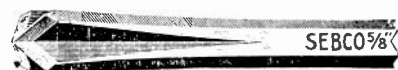
Fig. 66. This view shows the cutting nose of a star drill, such as used for drilling holes in masonry for attaching or running conduit in buildings of masonry construction.
