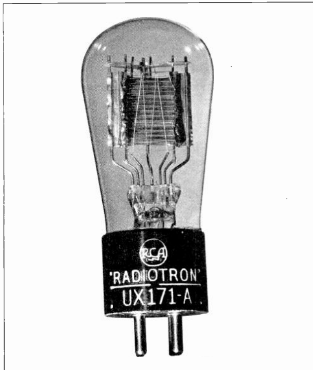
Fig. 44. Photograph of a vacuum tube with the plate opened up on one side to show the location of the grid and filament which are surrounded by the plate.
