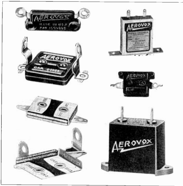
Fig. 87. Above are shown several types of fixed condensers used for coupling radio circuits and for bypassing certain frequencies around some of the inductive or high resistance devices in the circuits. (Photo courtesy of Aerovox Wireless Corp.)
