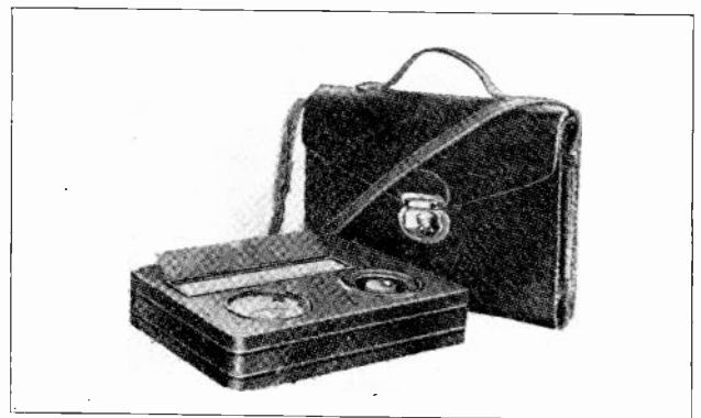
Fig. 166. A foot-candle meter is a very convenient instrument used for measuring illumination intensities right on the job.
