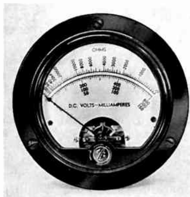
Fig. 3.—A single instrument with which may be measured voltage, current, and resistance.
