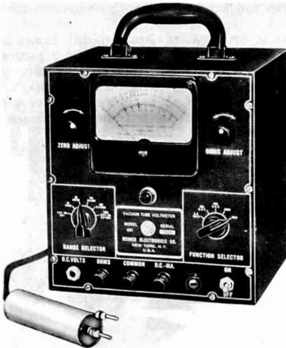
Fig. 22.—The Reiner electronic voltmeter with its high-frequency probe.
