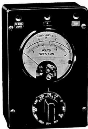
Fig. 13.—A Weston power level meter having 20,000 ohms constant impedance, and reading in volts and decibels.
