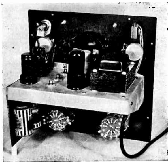
Fig. 26.—Calibration adjusters are on the shelf panel between the tubes.
