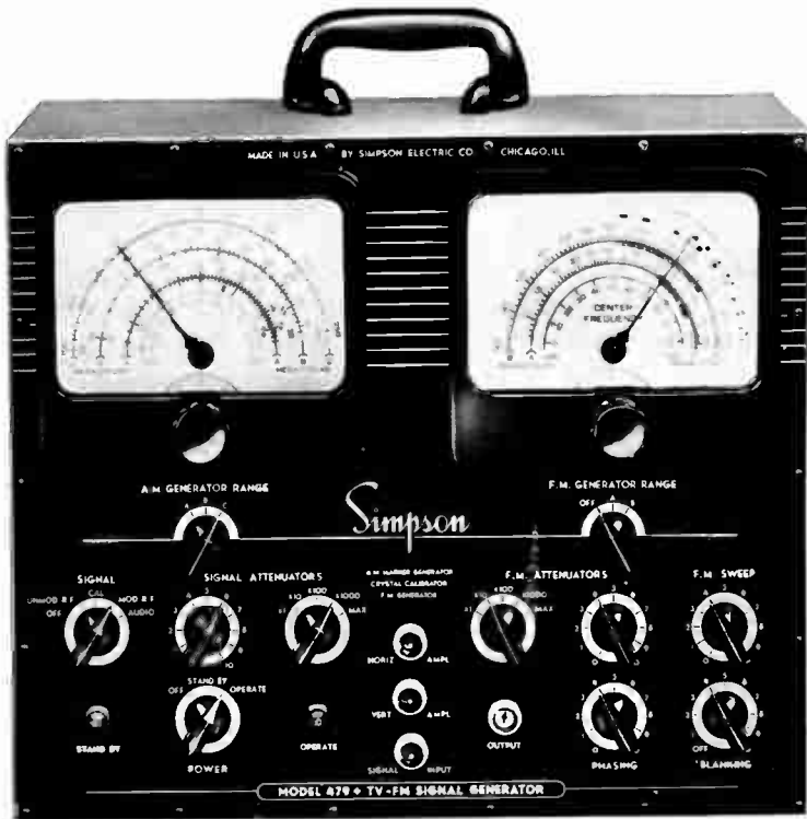
Fig. 1.—External appearance of the Simpson Model 479 FM-TV Signal Generator. Instrument is utilized chiefly for developing visual-response curve with markers for alignment of TV receivers.
