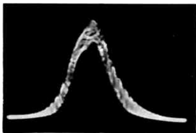
Fig. 31.—Effect of interfering station with frequency-modulated input.
