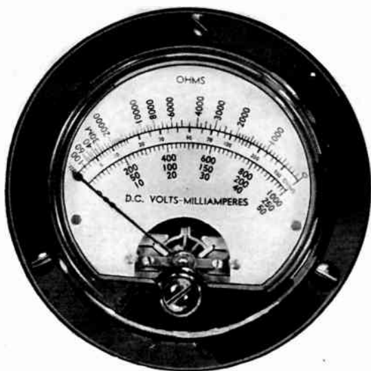
Fig. 2.—Meter scales for d-c volts and milliamperes, also for low and high resistances.
