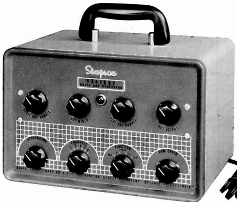
Fig. 1. —A typical white dot generator. This is a signal generator providing r-f output over the low VHF channels on pure fundamentals and over the high VHF channels on the second harmonics. Modulation of the output is complex amplitude modulation comprising negative pulses gating pulses, and horizontal and vertical sync pulses.
