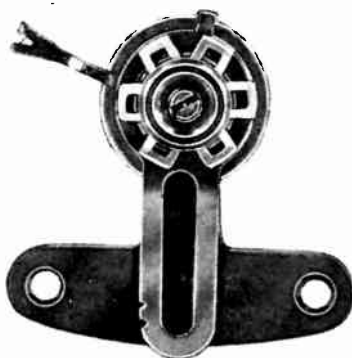
Fig. 13.—A zero adjuster with the jewel screw showing in the center.
