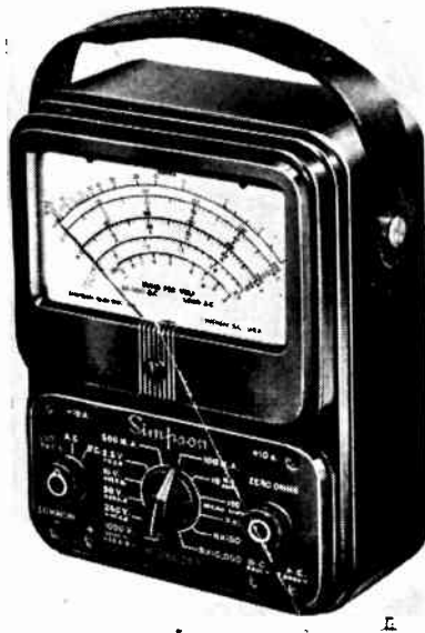
Fig. 1.—A Simpson analyzer for measuring various types of testing works, with several ranges for each kind of measurement.
