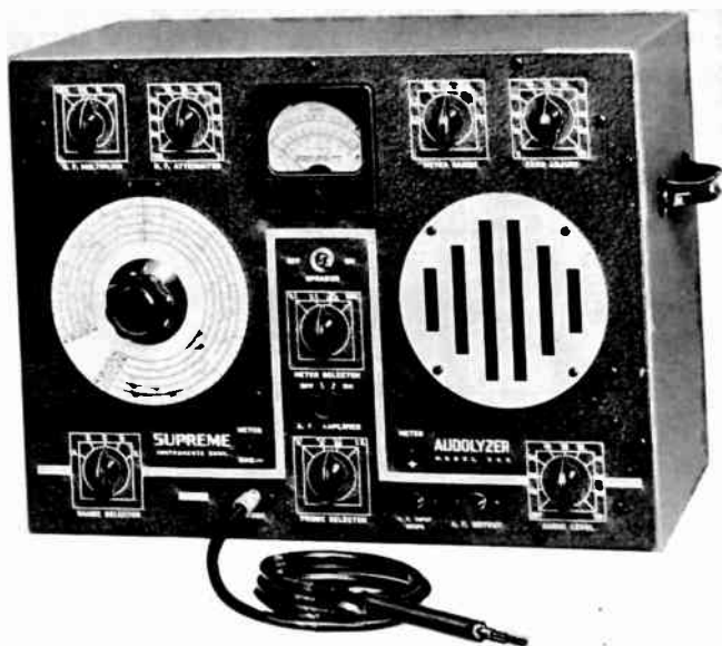
Fig. 1.—The Supreme Audolyzer, showing meter of electronic voltmeter, frequency measuring dial, speaker grille, test probe, and controls.
