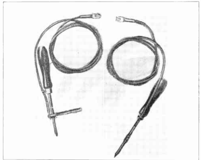
Fig. 19. This view shows a pair of test leads, one of which is equipped with a Cadmium stick for making Cadmium tests on storage batteries.
