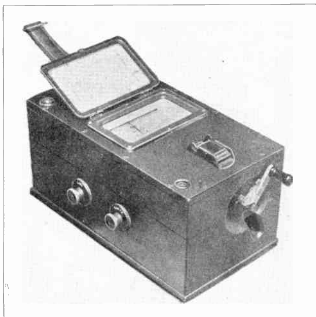
Fig. 102. The above photo shows a "Megger", or device used for measuring the resistance of insulation and high resistance circuits. This instrument contains its own D. C. generator as well as meter element.
