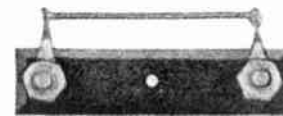
Fig. 96-A. Fire alarm fuse which melts when heated above normal temperature, opening the circuit and causing alarm to sound.
