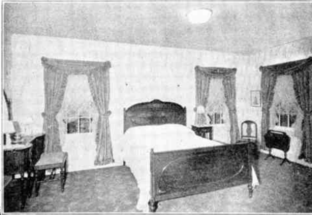
Fig. 251-A. This photo shows a well lighted bedroom, using the dome light in the ceiling and portable lights on the dresser and table.
