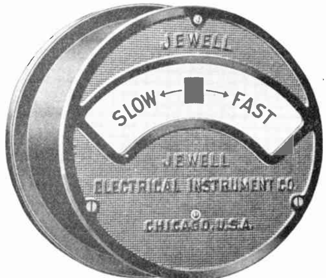
Fig. 76. Switchboard type frequency meter. With this type of instrument the pointer swings back and forth behind a transparent scale when the machines are out of phase.
