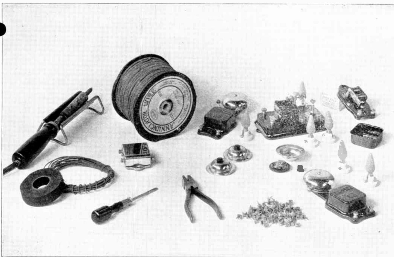
Fig. 107-B This photo shows a view of the more common parts and materials used in signal and alarm wiring.
