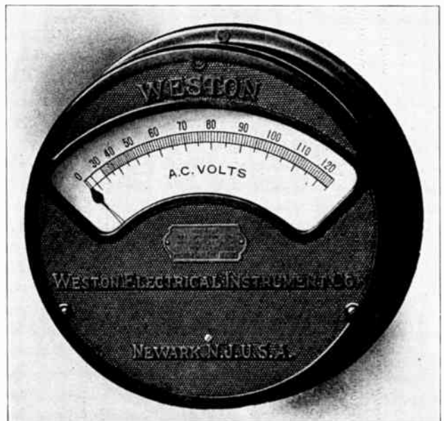
Fig. 52. Switchboard type A. C. voltmeter. Note the tapering graduation at the left end of the scale.
