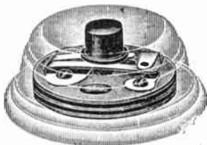
Fig. 12. Double circuit push button switch, showing clearly the arrangement of contacts and parts with respect to base and cover.
