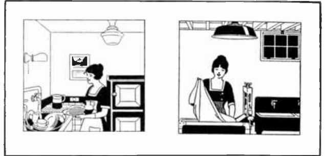
Fig. 253. At the left is shown the arrangement of ceiling unit and wall bracket light for kitchen. On the right a very efficient type of reflector for laundry rooms and basement lighting.
