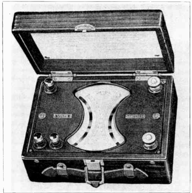
Fig. 51. This portable meter has two elements and two scales, and can be used to measure either volts or amperes. The voltmeter element has an extra terminal to provide increased voltage range of this instrument. (Photo courtesy Jewell Instrument Company)
