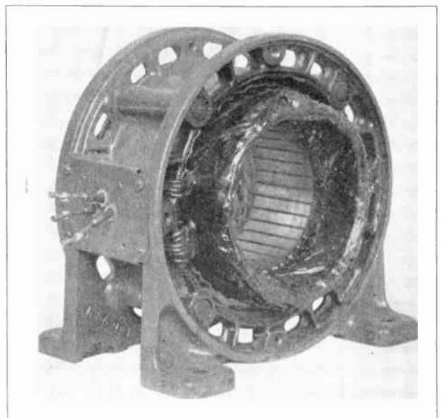
Fig. 89-B. The above photo shows a stator winding heavily impregnated with insulating compound. Note how insulation of this type affords mechanical strength and protection to the windings and would also prevent dirt, oil and moisture from getting in between the coils.
