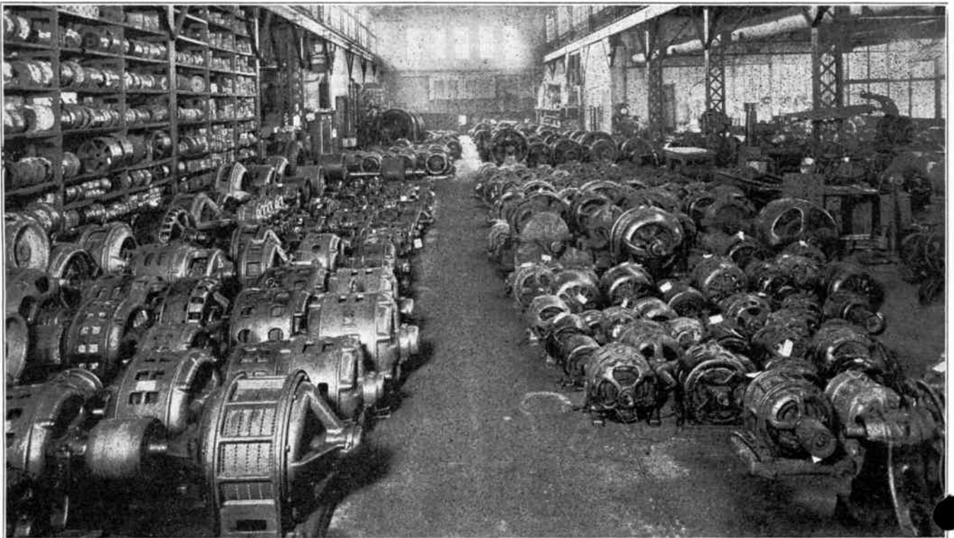
Fig. 1. This photo shows a view in a modern electric repair shop. Note the great number and variety of electrical motors and generators which go through this shop by the thousands each year. They are tested, rewound, reinsulated, and generally repaired before going back in service.
