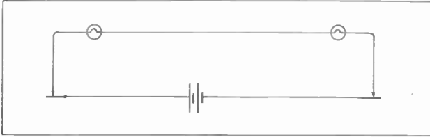
Fig. 15. Two closed circuit switches connected with lamps for a return call signal.
