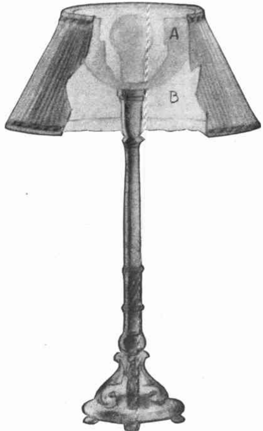
Fig. 255. Sectional view of new type student or reading lamps, showing diffusing bowl, shade and stand.
