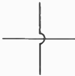
WIRES CROSSED NOT CONNECTED
