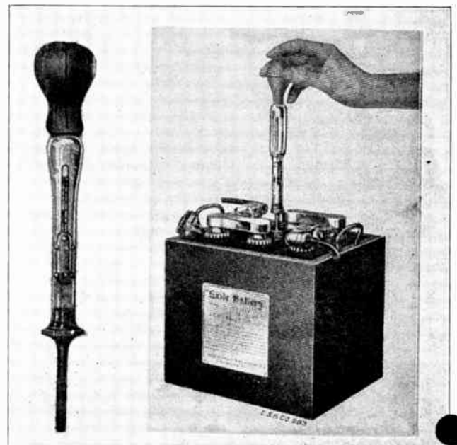
Fig. 12. On the left is shown a common battery hydrometer. Note the small float within the glass barrel of the hydrometer and also the rubber bulb on the top for drawing in the electrolyte. The view on the right shows the method of using a hydrometer for testing the electrolyte of a battery.
