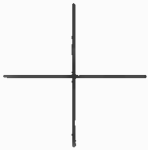
WIRES CROSSED NOT CONNECTED
