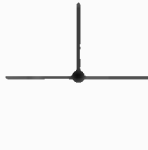
WIRES JOINED OR CONNECTED
