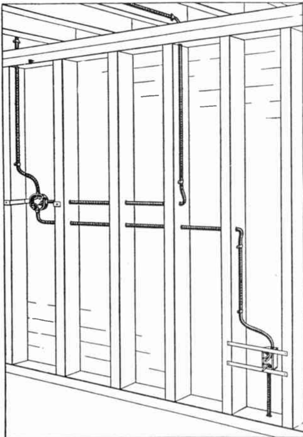
Fig. 54. A section of an installation of RomeX, showing how it is run through and along joists of a building.
