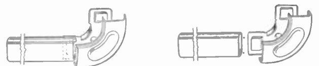
Fig. 93. A common form of elbow used with metal raceways or moldings
