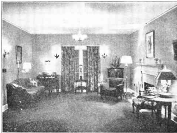
Fig. 245. Here we have the same room lighted by the ceiling unit, wall lights, and portable lamps. Compare carefully the different effects in the three photographs on this page.
