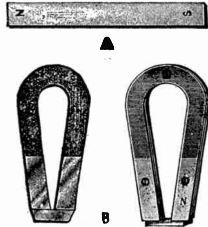
Fig. 67A. Common bar magnet. Fig. 67B. Horseshoe magnets with "keepers" across poles.
