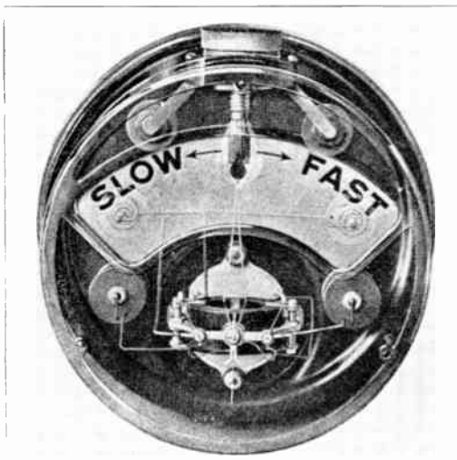
Fig. 77. This view shows the inside of a synchroscope and the arrangement of the various parts, including the lamp and meter coils.
