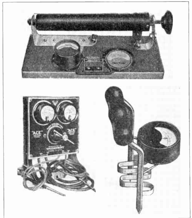
Fig. 22. Several styles of hy-rate discharge test sets. The one above is for either portable or bench use. The one at the lower left for bench use, and the one at lower right for portable use for testing individual cells.
