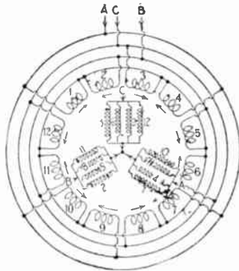
Fig. 81. Again we have the three-phase, four-pole winding. This diagram has all four poles of each phase connected in parallel and the three phase groups connected star as shown by the center sketch.
