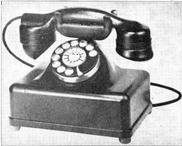
Fig. 159. Modern desk type telephone equipped with dial for automatic operation.
