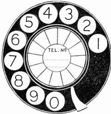
Fig. 152. Front view of dial, showing finger plate, holes, numbers and finger stop.
