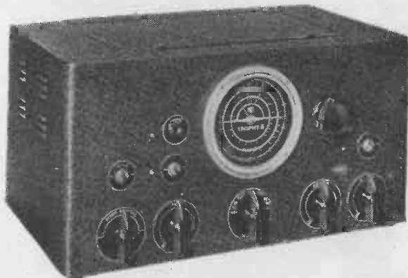
Fig. 2.—A typical modern short-wave receiver of the "communications" type, utilising all-metal construction.
