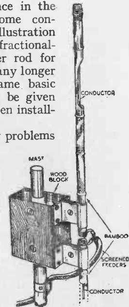
Fig. 33.—Using bamboo for supporting U.S.W. conductors.
