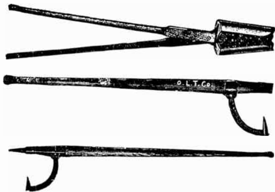
FIGS. 930 to 932.—Pole line construction tools. Fig. 930, split wooden handle post hole auger; fig. 931, cant hook; fig. 932, socket peavey.
