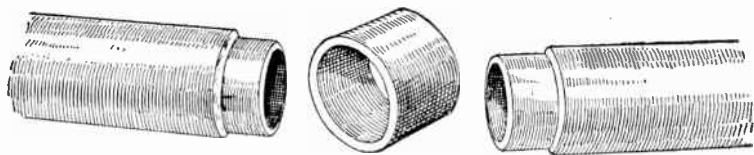
FIG. 985.—Sleeve joint type of fibre. Both the socket type (fig. 984), and the sleeve type here shown are easily aligned without the use of a mandrel.
