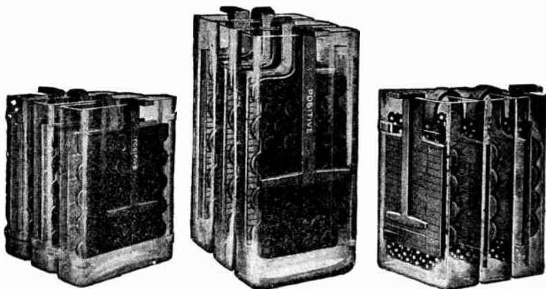
Figs. 1,124 to 1,126.—Electric Storage Battery Co. chloride cells. The voltage of cells of all capacities is slightly above 2 volts on open circuit, and during discharge at the 8 hour rate it varies from that point at the beginning to 1.75 volts at the end.
