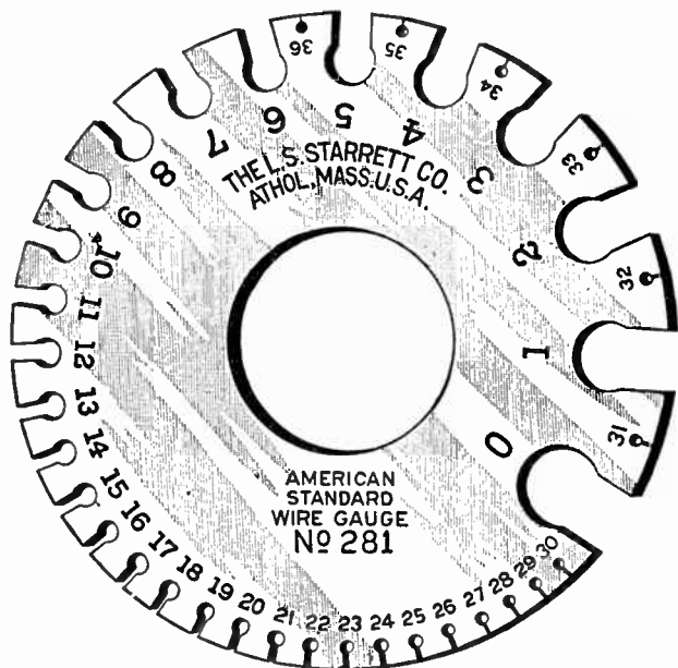
FIG. 822.—Brown and Sharpe (B. & S.), or American Standard wire gauge. This gauge was adopted by the brass manufacturers Jan., 1858. The cut is full size, and therefore shows the actual sizes corresponding to the gauge numbers.
