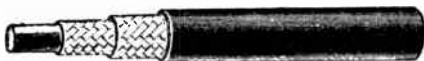
FIG. 811.—Slow burning weather proof wire. The insulation is composed of two braids thoroughly saturated with a fire proof composition, over which is a highly polished weather proof third braid. This wire was formerly known as "fire and weather proof" wire.
