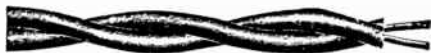
FIG. 815. —Pothead wires. The standard wire for pothead work is either No. 19, 20 or 22 B. & S. gauge, either single conductor or twisted pair, insulated to a diameter of \frac{3}{32} inch over rubber, without any outer braid or protection. In the case of twisted pairs one conductor is usually made of a differently colored rubber than the other, so as to distinguish between them.
