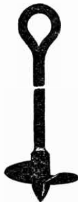
FIG. 943.—Stombaugh guy anchor. It is made of cast iron and can be screwed into the ground like an auger.
