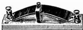
FIG. 1,030.—Thermal flasher. This simple flasher consists of a brass strip fixed at each end to a porcelain base and slightly arched upwards. The amount of this arching, however, is much less than is shown in the figure. The center of the strip carries a platinum contact on its upper surface, and opposite this is a platinum tipped contact screw which is carried in a brass angle piece fixed to the base. One terminal is fitted on one end of the strip, and the other is connected, through the angle piece, with the contact screw. The strip is wound from end to end with an insulated resistance wire, one end of this being soldered to the strip, and the other connected to the right hand terminal. When this device is switched into circuit with the lamps, the current first flows through the resistance, which cuts it down so much that the lamps are not visibly affected. The heat generated in the resistance causes the strip to curve still more, till at length contact is made, the resistance short circuited, and the lamps lighted.
