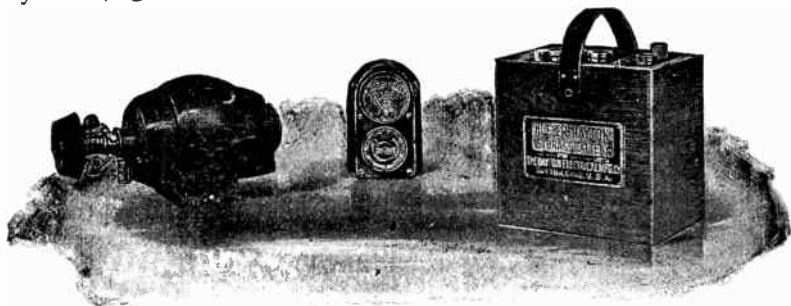
FIG. 1,192.—Dayton launch lighting outfit. It consists of an "Apple" dynamo, switchboard and storage battery. The dynamo is fitted with a bevel friction drive governor. The dynamo gives a three ampere charging rate on a six volt battery at its normal speed of 1,050 R. P. M. The switchboard is provided with a combination vol-ammeter which shows the voltage of the battery, the ampere charging rate of the dynamo and the ampere discharging rate of the battery. The automatic cut out in the back of the switchboard automatically severs the connections between the dynamo and the storage battery when the engine stops and so prevents the storage battery current running back through the dynamo when the dynamo is not generating current. A 6 volt, 60 ampere hour battery, consisting of 3 five plate units connected in series, is used with the size dynamo shown in the illustration.
