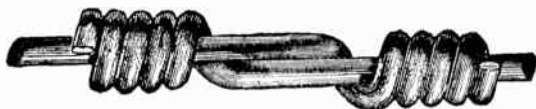
FIG. 961.—American wire joint. This is a simple method of connecting the ends of the sections of wire by tightly twisting the ends around each other for a few turns; it is the standard Western Union wire joint.
