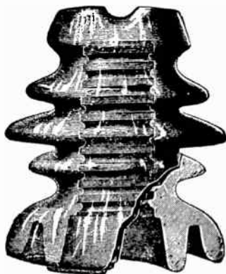
FIG. 967.—Type of insulator used in making a transposition.
