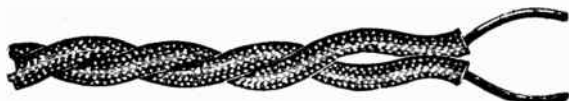
FIG. 809.—Twisted weather proof wires. The insulation consists of two or three thicknesses of braided cotton saturated with a moisture resisting insulating compound.
