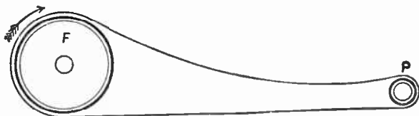
FIG. 448.—Right way to run a belt. The pull should come on the lower side bringing the slack on top.
