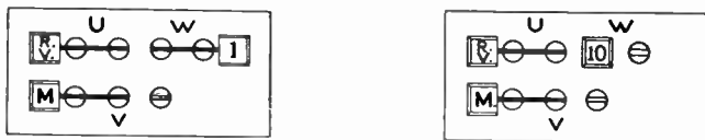
FIG. 605.—To use galvanometer of Leeds and Northrup fault finder in series with the battery: Set switches as shown, and connect between posts Gr. and 2 (see figs. 587 and 588). The galvanometer will have the maximum sensibility with the pointer at 1,000 and the minimum at zero.
