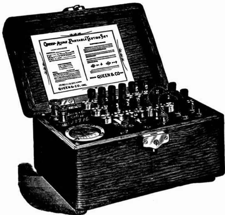
FIG. 576. —Queen Acme portable testing set. It consists of a Wheatstone bridge, with reversible arms, battery of four dry cells, D'Arsonval galvanometer, battery and galvanometer keys. There are sixteen resistance coils, having a combined resistance of 11,110 ohms. Each bridge arm is provided with three coils of 1, 10, 100 ohms, and 10, 100, 1,000 ohms respectively. The commutator admits of a ratio of 1 to 1,000 on either bridge arm, giving the set a theoretical range from .001 of an ohm to 11,110,000 ohms. For resistances above 1,000,000 ohms, the normal battery power must be increased. The contact keys are located as shown. The battery key has single contact, but the galvanometer key has double contact; depressing it closes the galvanometer circuit, and releasing it short circuits the galvanometer, bringing the latter quickly to rest.
