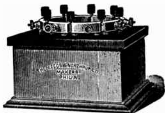
FIG. 563. —Standard resistance box: 100,000 ohms, in four units of 10,000, 20,000, 30,000, and 40,000 ohms. An "infinity" plug separates each coil from the ones adjacent. Segments are elevated from the hard rubber top by special washers in order to increase insulation. Binding posts are so arranged as not to be in the way when plugs are used.
