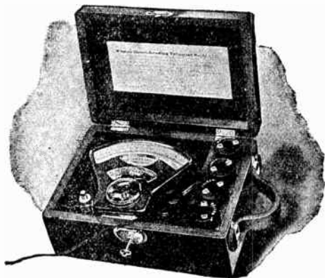
FIG. 632.—Weston portable voltmeter, inspector's style. This instrument is provided with a reversing key. Instead of the regular binding posts, pins are used with which connections are made by means of contact cups, attached to flexible cords. These contact cups are convenient in making connections, or in changing quickly from one range to the other, if the instrument have a double scale. Connections for the different ranges are made in precisely the same way as with the regular double scale voltmeters. For the upper scale values, the contact pin to the right and the front contact pin to the left being taken, and for the lower scale values, the left contact cup is changed to the rear contact pin.
