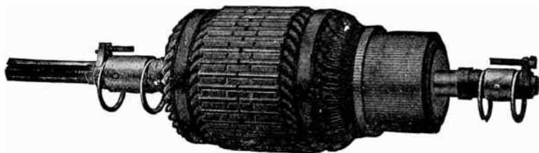
FIG. 400.—Fairbanks-Morse armature for 7\frac{1}{2} H.P., 1300 R.P.M., TR type motor. The armature core is built up of thin sheet steel laminations with notches in the circumference, which, when the discs are placed together, form grooves or slots to receive the armature coils. The armature cores for the larger machines are mounted on a cast iron spider, which also carries the commutator, making the two parts entirely self-contained, and with this construction, it is possible to remove the armature shaft, without disturbing the core, commutator or windings. Cores of all sizes are provided with ventilating spaces, running from the surface to the central opening of the core, so that air is drawn through the core and blown out over the windings by the revolution of the armature.
