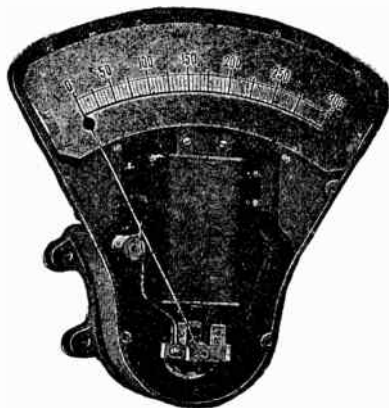
FIG. 640.—Thompson astatic instrument without cover. When current passes through the coils of the moving element, the lines of force parallel to the shaft produce a torque which tends to turn the shaft and cause the needle to travel across the scale. This action is, of course, opposed by the magnetic field at right angles to the shaft acting on the two pieces of magnetic metal. These astatic instruments have no controlling springs. The two small silver spirals which conduct the current to and from the armature are made of untempered silver and exert no force as springs. The actuating and restraining forces are dependent upon the same electromagnets. The damping effect in these instruments is produced by an aluminum disc moving in a magnetic field, and is proportional to the square of the magnet strength.
