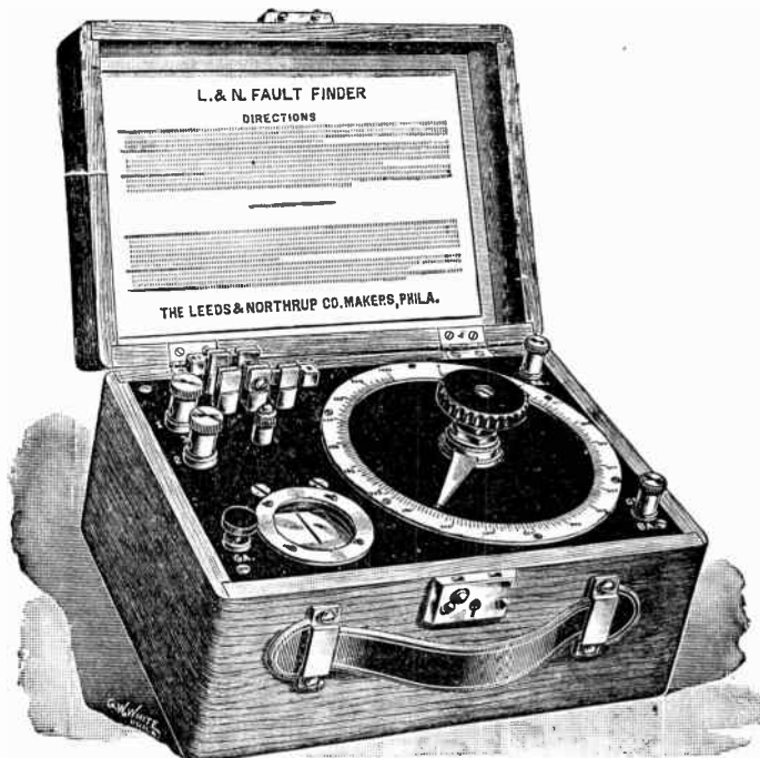
FIG. 587.—Leeds and Northrup fault finder. A lineman's instrument for the location of faults, crosses, grounds, and opens in telephone and telegraph circuits, and for the measurement of conductor and insulation resistance.
