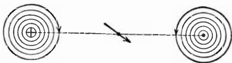
FIG. 517.—Horizontal section through middle of tangent galvanometer, showing magnetic whirls around the coil and corresponding deflection of needle.
