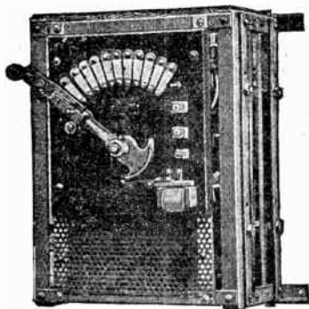
FIG. 760.—Cutler-Hammer speed regulator with no voltage release, regulation by armature resistance only , reducing speed of motor below normal . No resistance in the armature circuit. No provision is made in regulators of this type for increasing the speed of the motor. The maximum speed obtainable when these regulators are used is, therefore, the normal speed at which the motor is designed to operate with no resistance in circuit. With all resistance in circuit and the motor taking normal current these regulators will reduce the speed of the motor 50 per cent. If the motor be taking less than normal current the percentage of speed reduction obtainable will be correspondingly less. The notched fan tail extension on the lower end of the lever engages with a magnetically operated pawl to hold the lever squarely on any contact so long as the no voltage release magnet is energized.
