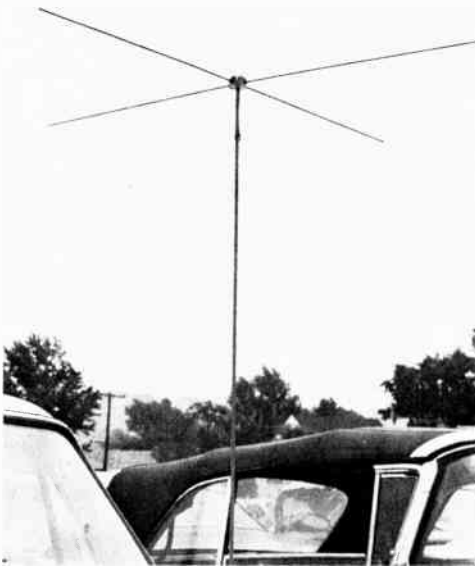
Fig. 19-20—Two-meter turnstile antenna shown mounted on the front of an automobile. The miniature coax cable which feeds the antenna is topped to its 1/4-inch diameter steel supporting rod. The ends of the antenna elements should be flattened, or rounded, to make them safer in the event of accidental contact with the human body.
