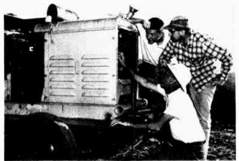
Fig. 19-5—Gasoline-powered ac generators used for portable/emergency operation should be treated for ignition noise in the same manner as automobile engines are. The frame of the gas generator should be connected to an earth ground, and the entire unit should be situated as far from the operating position as possible. This will not only reduce ignition noise, but will minimize ambient noise from the power unit. (Shown here are WA6LXX, WA6HUB, and W6PQH during portable operations.)
