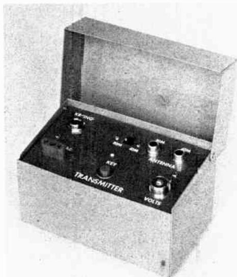
Fig. 6-35—This version of the solid-state transmitter is housed in a small recipe box. All controls and jacks are accessible from the top panel.
