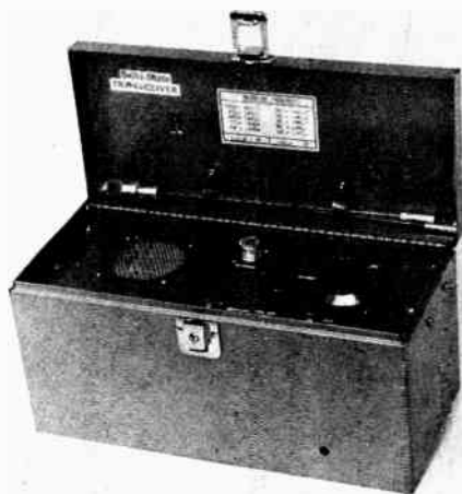
Fig. 19-34—The 2-meter transceiver is housed in a legal-bond box. A homemade dial-calibration chart for the receiver is posted on the inside of the lid. Two plastic cable clamps serve as holders for the two-section \frac{1}{4} -wavelength whip antenna (inside lid) when the unit is not in use. The antenna is held together at the center by a homemade \frac{1}{4} -inch diameter threaded coupling.
