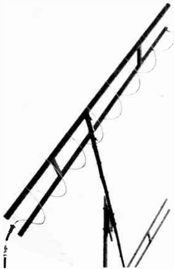
Fig. 18-13—An 8-turn 432-Mc. helical array. The helix is made from aluminum clothesline wire, but copper tubing could be used as well. The screen reflector is fashioned from galvanized hardware cloth. This beam is wound for left-hand circular polarization.
