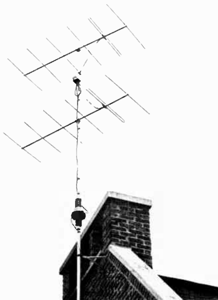
A stacked array for 144 Mc. (W1AW) which uses \frac{5}{8} -wavelength spacing. The phasing lines and the \frac{1}{2} -wavelength balun are joined in a weatherproof box. Element lengths for such an array can be taken from table 18-1. Element spacing is 0.2 wavelength.
