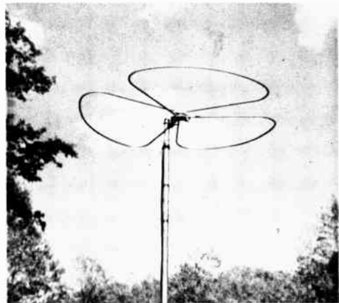
Fig. 19-18—The Big Wheel, an omnidirectional horizontal antenna for the 144-MHz band designed by W1FVY and W1IJD. Radiating elements occupy an area approximately 40 inches in diameter.
