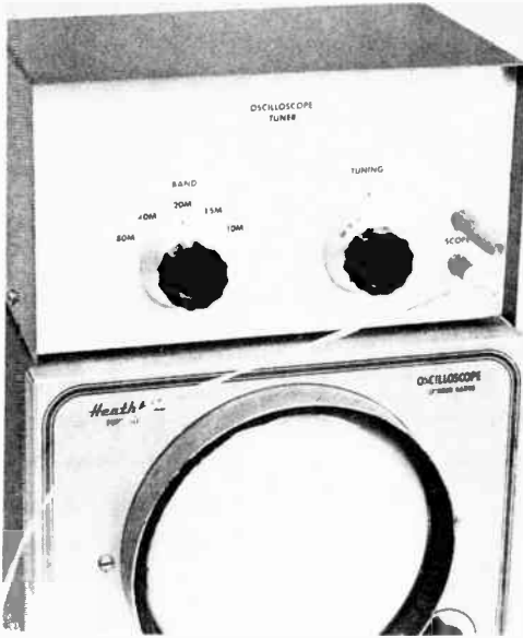
Fig. 9-21—An oscilloscope adaptor permits monitoring of the output rf envelope from an hf transmitter. Any shop-type oscilloscope may be used.
