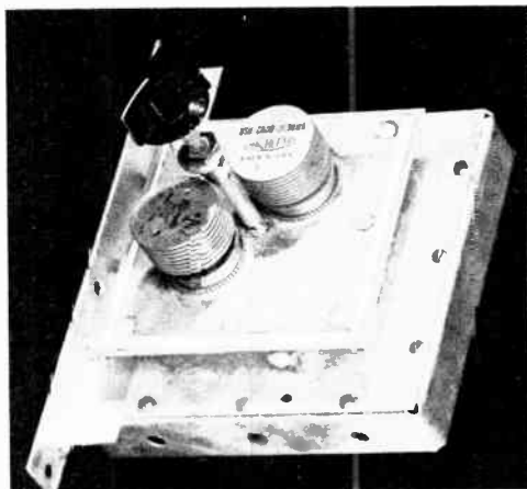
Fig. 17-33—The 2-tube 1296-Mc. amplifier. Two 2C39As are used in this grounded-grid setup. The large square base unit houses the cathode input circuit. The plate cavity is not visible, as it is obscured by the plate bypass assembly seen here. (Built by WB6IOM)
