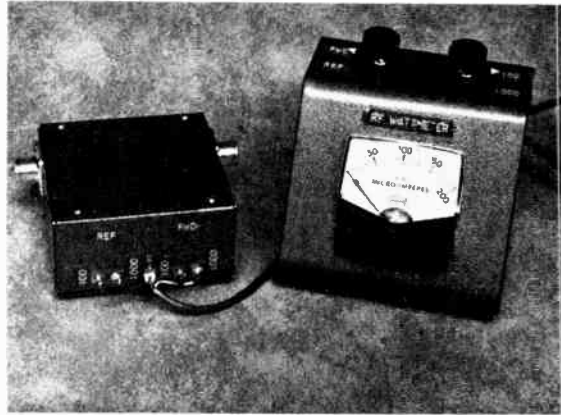
Fig. 21-47—Outside view of the power meter. The rf head is built in a 4 x 4 x 2-inch utility box. A sloping-panel cabinet houses the controls and meter. A four-wire shielded cable joins the two pieces.
