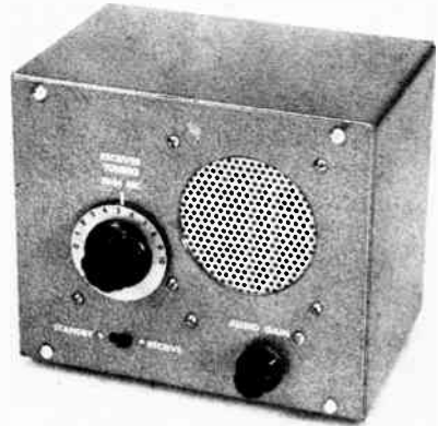
The transistorized 6-meter receiver uses two FETs and three bipolar transistors in a sensitive superregenerative lineup. The main-tuning control does not need a vernier drive because of the broad-tuning effect of this type of detector. A vernier drive can be added, however, if the operator wishes.
