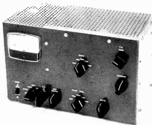
Fig. 6-41—This 120-watt cw transmitter can be operated at 75-watts dc input for Novice-band use. The slide switch puts the meter in the grid or cathode circuit of the 6146B amplifier. Directly to the right of the slide switch is the FUNCTION switch and crystal socket. Continuing at this level, farther to the right is the GRID TUNING, grid BAND SWITCH, and the DRIVE level control. The controls to the upper right are the final BAND SWITCH, FINAL TUNING, and FINAL LOADING.
