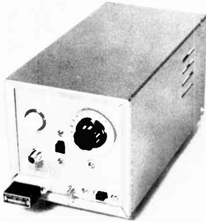
Exterior view of the 15-watt transmitter. All controls are located on the front panel.
