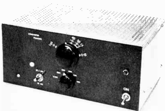
Fig. 5-47—Outside view of the five-band converter. The peaking control is at the top center with the band switch directly below. A homemade cabinet encloses the equipment, and the front panel is painted a royal blue to set off the white decal labels.
