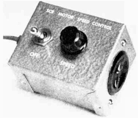
Fig. 20-B—Small enough to fit in the palm of your hand, the SCR motor-speed control is housed in a small Minibox.
