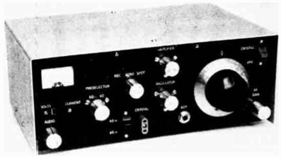
Fig. 19-40—Front view of the cw transceiver. The chassis and cabinet are homemade, and consist of two U-shaped pieces of thick aluminum stock. The panel is painted dark green to permit the white decal labels to stand out prominently.
