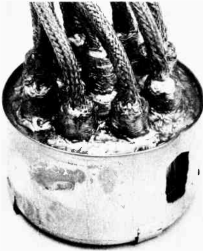
Fig. 19-4—A close-up view of the distributor shield can. The shield braid over each spark-plug wire is soldered to the top of the can, and the can is grounded to the engine block.
