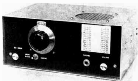
Fig. 5-51—Front view of the direct-conversion receiver. The panel is finished in machine gray spray paint. The two controls are main tuning and audio gain.
