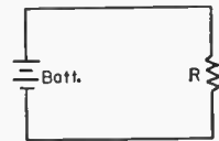
Fig. 2-3—A simple circuit consisting of a battery and resistor.
