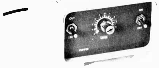
Fig. 9-16—Front view of the rf speech clipper. The unit is built in an LMB CO-3 cabinet.
