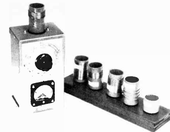
Fig. 21-42—Absorption frequency meter for 1.6-300 MHz.
