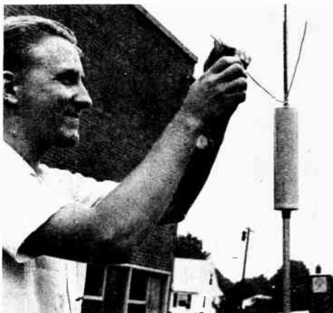
Fig. 19-15—K1MET prunes a capacity hat for antenna resonance at the low end of the 160-meter band. The Webster Big-K antenna is first tuned for the high segment of the band. The capacity hat is clipped on when operation on the "low end" is desired. Fine adjustments can be made by increasing or decreasing the spacing between the two No. 10 wires.
