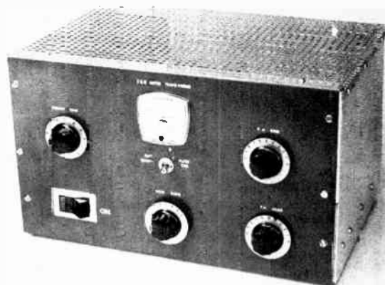
Fig. 9-43—The transceiving converter is housed in a homemade aluminum cabinet which measures 8 \times 8 \times 12 inches. Perforated aluminum is used for the top and back sides of the cabinet to assure good ventilation.
