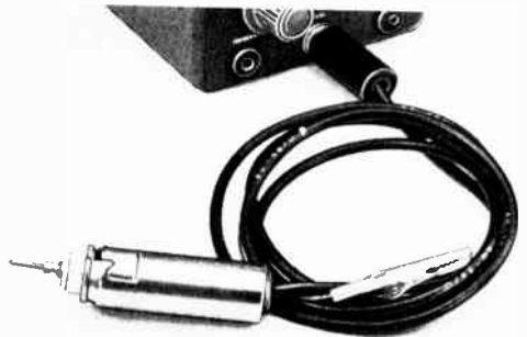
Fig. 21-56—Rf probe for use with an electronic voltmeter. The case of the probe is constructed from a 7-pin ceramic tube socket and a 2¼-inch tube shield. A half-inch grommet at the top of the tube shield prevents the output lead from chafing. A flexible copper-braid grounding lead and alligator clip provide a low-inductance return path from the test circuit.
