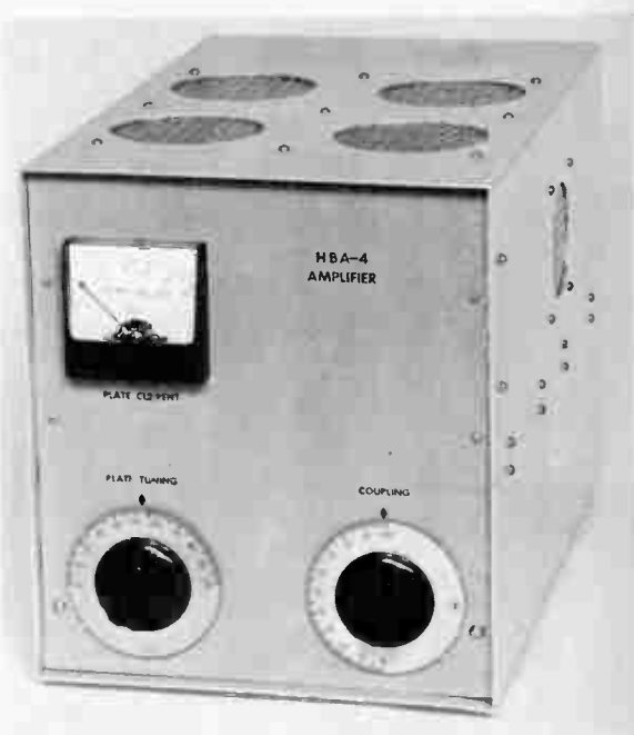
Fig. 6-60—The amplifier has one vent hole on each side of the home-made cabinet, and four holes on the top. Each hole, and the back side of the cabinet, is enclosed by means of perforated aluminum. The cabinet was formed by making two U-shaped sections of \frac{1}{8} -inch thick aluminum and mating them. They are held together by means of two 1-inch wide aluminum strips (inside) and 4-40 hardware.
