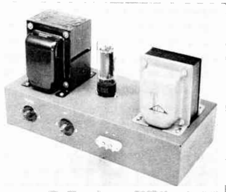
Fig. 7-33—A typical low-voltage power supply. The two o.c. connectors permit independent control of filament and high voltage.
