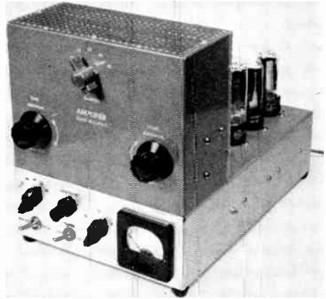
Fig. 6-47—Front view of the 6146 all-purpose amplifier. The upper panel is part of an 8 × 6 × 3½-inch Minibox (Bud CU-2109); the ventilated shielding of Reynolds Aluminum cane metal is fastened to the Minibox and base with sheet-metal screws.
