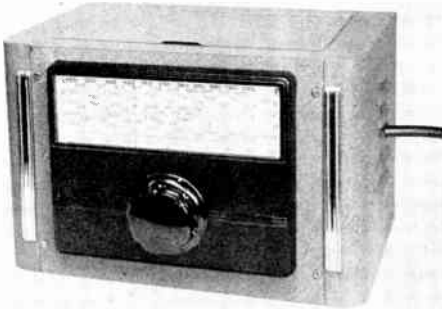
Fig. 6-57—The remote v.f.o. tuning unit is housed in a standard metal cabinet. The cable at the right plugs into the main chassis.
