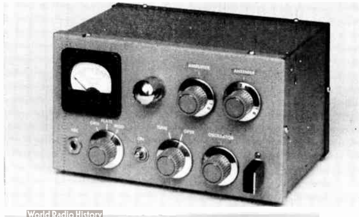
Fig. 19-14—A panel-illuminating lamp is mounted to the right of the meter, along with the amplifier-tank and antenna-link tuning controls. Along the bottom, from left to right, are the microphone jack, meter switch, filament switch, tune-operate switch, oscillator tuning control and the crystal.
