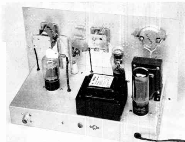
Fig. 6-37—Rear view of the transmitter showing the placement of components above chassis. The loading capacitor, C_3 , is at the left, L_1 is the vertical coil and L_2 the horizontal one. Rubber grommets are used to prevent chafing and to furnish additional insulation on the leads coming from below chassis.
