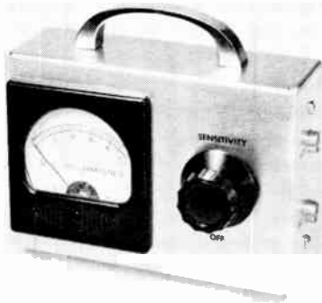
Fig. 19-40—A front view of the field-strength meter. Sensitivity control R_1 is to the right of the 0-1 indicating meter. Antenna input and output connectors are mounted on the right end of the box.
