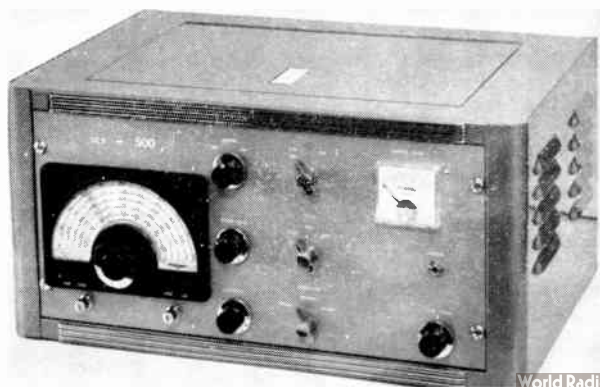
Fig. 5-54—The DCS-500 double-conversion superheterodyne. Left bottom, antenna trimmer, 100-ke. calibrator switch; center, left, top to bottom, noise-limiter switch, volume control, sensitivity control; center, right, b.f.o. switch, a.g.c. speed, selectivity; right, headphone jack, b.f.o. pitch control. The dial is a National ICN. Front panel is 8¾ inches high; the receiver is mounted in a Bud CR-1741 rack cabinet.
