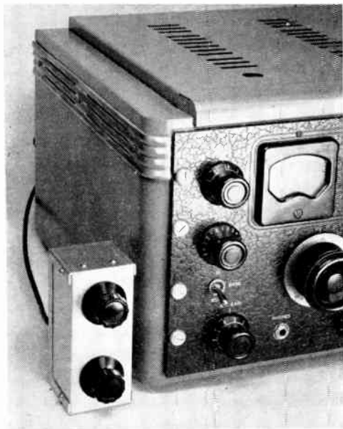
Fig. 5-63—View of the Q multiplier showing its single connecting cable to the receiver. The box can be placed in any convenient spot on or around the receiver.
