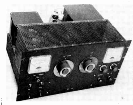
Fig. 6-67—This amplifier operates at a plate input of approximately 500 watts, uses a pair of 811As in grounded-grid, and is complete with power supply on a 13 × 17 × 4-inch chassis. The rack panel is 10½ by 19 inches. Front-panel controls include the plate tuning capacitor and band switch in the center, filament and plate power switches with their pilot lights at the lower left, sensitivity control and forward-reflected power switch for the directional coupler at the lower right, variable loading capacitor and auxiliary loading-capacitor switch underneath the 0-1 milliammeter at the right, and the grid-cathode milliammeter with its switch at the upper left. The filter choke, 866As and plate transformer occupy the rear section of the chassis.
