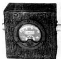
Fig. 21-27—R.f. ammeter mounted for connecting into a coaxial line for measuring power. A "2-inch" instrument will fit into a 2 \times 4 \times 4 metal box.
