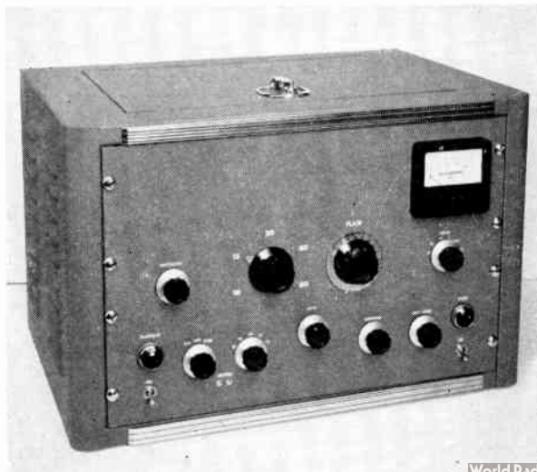
Fig. 6-53—A 500-watt transmitter. Power supplies and a differential keyer are included. It operates with the external v.f.o. tuner shown in Fig. 6-57. Controls along the bottom, from left to right, are for low-voltage power, v.f.o./crystals/s.s.b. switch, driver tank switch, driver tank capacitor, final loading, v.f.o. set switch, and high-voltage. Above, from left to right, are controls for excitation, final tank switch, final tank capacitor and meter switch. The band-switch pointer is made by cutting down the metal skirt of a dial similar to the one to the right.
