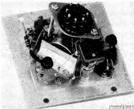
Fig. 5-61—Inside view of the calibrator unit. The 100-ke. oscillator coil, L_{15} , is at the right, the oscillator transistor, Q_2 , is in the foreground mounted to the crystal socket, and the amplifier transistor, Q_1 , is mounted at the right on a terminal strip. The 100-ke. crystal is mounted horizontally between the plate and the octal plug. The plug can be mounted on 2-inch screws as shown in the photograph, or on the bottom plate of the Minibox, with flexible leads to the circuit. If the calibrator is to be used as a self-contained unit (see text) the octal plug is not necessary.
