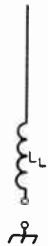
Fig. 19-30—The capacitive reactance at frequencies lower than the resonant frequency of the whip can be canceled out by adding an equivalent inductive reactance in the form of a loading coil in series with the antenna.
