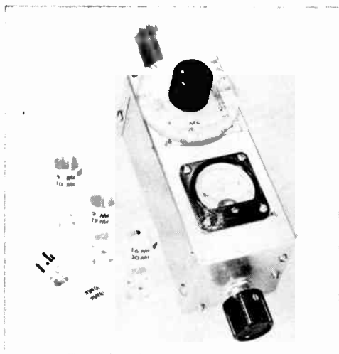
Fig. 21-19—Transistor circuit-checker or "grid-dip meter" covering 3 to 40 Mc. in five ranges. The circuit and battery power supply are contained in the 2\frac{1}{4} \times 2\frac{1}{4} \times 5 -inch aluminum box (Bud CU-3004) so the instrument is completely independent of the a.c. line. The dial is white cardboard with an inked-on calibration; the hairline indicator is on a Lucite disk cemented to the tuning knob. The d.c. meter is a miniature type, but the box is large enough to take a standard 2-inch instrument. The control on the near edge is R_2 , for setting the d.c. meter reading to a suitable on-scale value.
