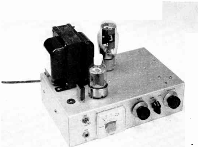
Fig. 6-39—This view of the 50-watter shows the panel arrangement and layout of the components above chassis. The crystal is between the 6146 and dial-light grommet. Behind the 6146 is the power transformer and to its right is the rectifier tube.
