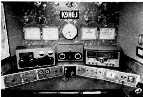
In this station arrangement, eight small panels near the front of the table carry the auxiliary gear. From left to right: (1) loud speaker with selector switch to receivers or monitor; (2) conelrad receiver and automatic transmitter disabler; (3) Monimatch; (4) antenna selector switch; (5) intercom to other rooms in house; (6) station control switch; (7) beam rotator control; (8) transmission timer and monitor. All eight accessory units are completely enclosed in perforated aluminum and are plug in. (K9HGJ, Milwaukee, Wisc.)
