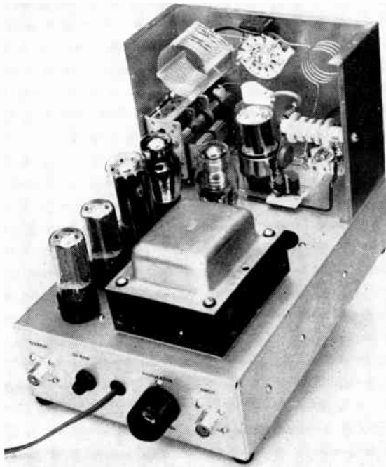
Fig. 6-48—Rear view of the 90-watt all-purpose amplifier with the cane-metal cover removed. One voltage-regulator tube has been removed from its socket (right edge of transformer) to allow the neutralizing capacitor and plate blocking capacitor to be seen. The plate r.f. choke (RFC 3 in Fig. 6-49) is mounted on one side wall, and the load capacitor and safety choke ( C_4 and RFC 4 in Fig. 6-49) are mounted on the far side wall.
