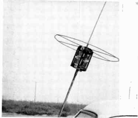
Fig. 19-34—The top-loaded 4-Mc. antenna designed by W6SCX. The loading coil is a B & W transmitting coil. The coil can be tuned by the variable link which is connected in series with the two halves of the coil.
