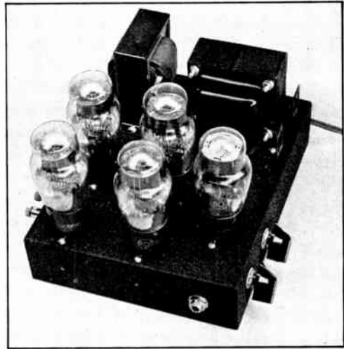
Fig. 8-9 — A vacuum-tube keyer, built up on a 7 X 9 X 2-inch chassis with space for four or less keyer tubes and the power-supply rectifier. The resistors and condensers that produce the lag are underneath, controlled by the knobs at the right. The jack is for the key, while terminals at the left are for the keyed circuit.
