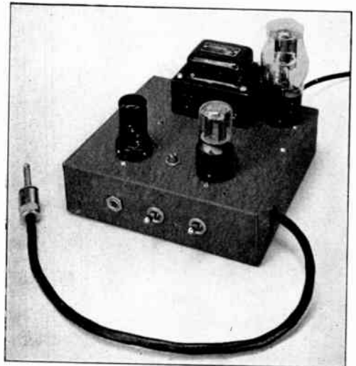
Fig. 8-15 — A top view of the "Monitone." The shaft of the screwdriver-adjusted potentiometer controlling tone and volume is located between the 6J5 and 6SL7 tubes. The right-hand switch controls the a.c., and the center switch cuts the tone oscillator in and out.
