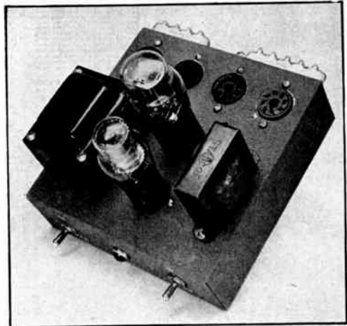
Fig. 7-17 — A receiver-type supply that delivers 250 volts at 35 ma. and a regulated potential of 150 volts at 15 ma. The amount of current which can be drawn from the 150-volt tap can be made higher or lower by selecting a suitable limiting resistor for the regulator tube; the current output will increase as the resistance value is reduced. The total current drain imposed on the supply should not exceed 50 ma. unless a transformer of greater current capacity is used. The four octal tube sockets on top of the chassis are wired in parallel with screw-type terminals and pin jacks at the rear to provide an assortment of terminals to which external circuits may be connected. The wiring diagram for the supply is shown in Fig. 7-18.
