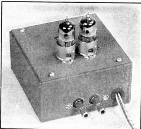
Fig. 15-14 — A transmitter for 420 Mc. using two 6J6 tubes in push-pull-parallel. Antenna coupling terminals project through the front of the chassis,
