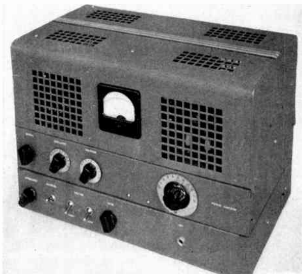
Fig. 6-48 — Front view of the push-pull 807 transmitter showing the arrangement of controls.
