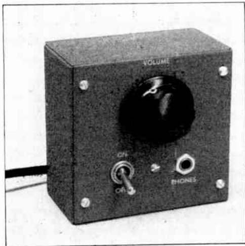
Fig. 5-42 — A simple audio noise limiter for reducing operator fatigue caused by ignition noises, key clicks and static crashes.
