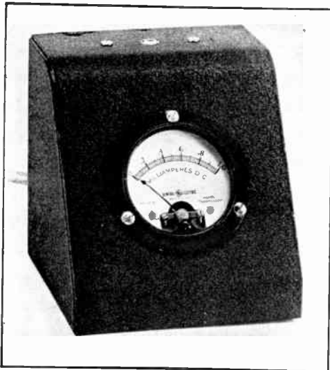
Fig. 5-45 — Front view of the signal-strength indicator. The 0-1 milliammeter is mounted in a metal meter case. The zero-adjustment potentiometer, R_4 , is mounted below the top of the cabinet by means of a "U"-shaped bracket; the potentiometer shaft is slotted so that it can be adjusted with a screwdriver. A new face, calibrated in S-units, can be pasted to the 0-1 ma. scale, or a calibration chart can be attached to the cabinet.
