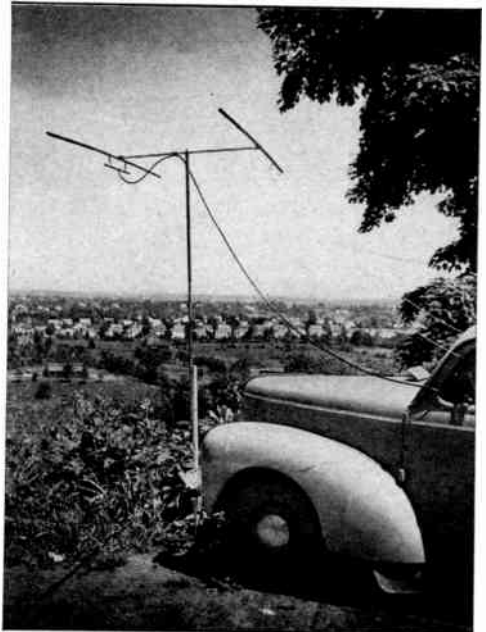
Fig. 14-12 — A 2-element collapsible array for 50-Mc. portable use.
