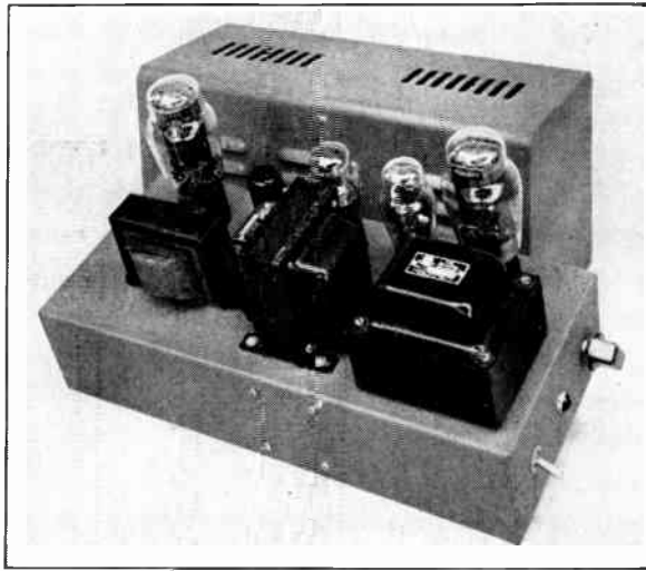
Fig. 7-20 — A heavy-duty electronically-regulated power supply. The unit is assembled on a 6 × 14 × 3-inch chassis fitted with an enclosing cover. The five tubes across the rear, left to right, are the 6AS7G regulator, the 6SJ7 control tube, the VR-105 bias regulator, the 1-V bias rectifier and the 5U4G power rectifier. In the foreground are the two filter chokes and the power transformer. The remainder of the components are mounted underneath.
