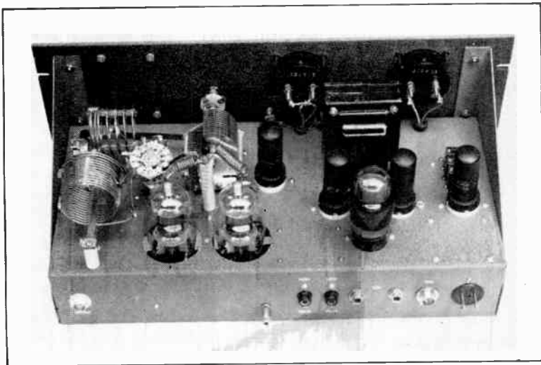
Fig. 6-76 — Rear view of the bandswitching transmitter-exciter.
