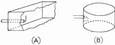
Fig. 15-32 — Coupling to wave guides and resonators.
