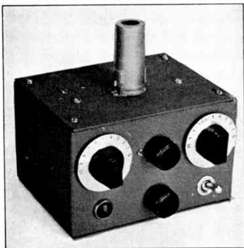
Fig. 5-59 — A front view of the ten-meter converter. The components and controls on the front wall of the case, from left to right, are as follows: top row, r.f. tuning control, oscillator tuning knob, and i.f.-circuit control; bottom row, dial-light assembly, antenna change-over switch, and filament switch.
