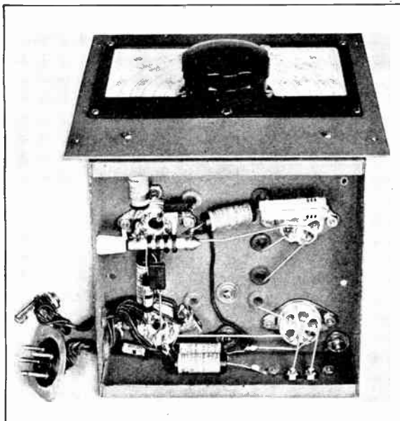
Fig. 1380 — High-frequency connections underneath the chassis of the v.f. exciter unit are made with short, straight sections of heavy wire. The two zero-temperature padding condensers are soldered directly to the oscillator-coil socket. All components are mounted firmly with no opportunity to support mechanical vibration. Washers 1/16-inch thick are placed between the panel and the chassis to provide space for the lower lip of the cabinet opening.
