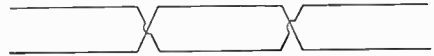
Fig. 1008—Transposing a two-wire open transmission line preserves balance to ground and to near-by objects.
