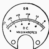
Fig. 1934 — A logarithmic field-intensity meter with db. calibration, employing a variable- \mu d.c. amplifier tube.
