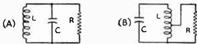
Fig. 239 — The equivalent circuit of a resonant circuit delivering power to a load. The resistor R represents the load resistance. At (B) the load is tapped across part of L , which by transformer action is equivalent to using a higher load resistance across the whole circuit.
