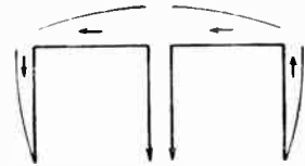
Fig. 1036 — Folded arrangement for shortened antennas. The total length is a half wave, not including the feeders. The horizontal part is made as long as convenient and the ends dropped down to make up the required length. The ends may be bent back on themselves like feeders to cancel radiation partially. The horizontal section should be at least a quarter-wave long.
