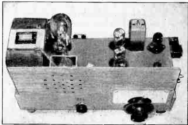
Fig. 1520 — Top view of the superheterodyne receiver. The i.f. amplifier tube and output transformer are in the rear right-hand corner. The detector and audio tubes are in line to the right. Power-supply components and loudspeaker are at the left-hand end of the chassis.
