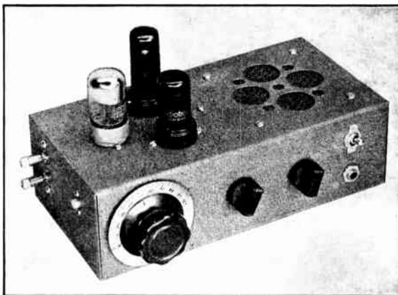
Fig. 1506 — A superregenerative receiver with built-in speaker, constructed on a standard chassis base as a cabinet. The detector trimming condenser is mounted on the left end. The audio gain control is at the right of the tuning dial. The regeneration control is between the gain control and the 'phone jack and on-off switch.
