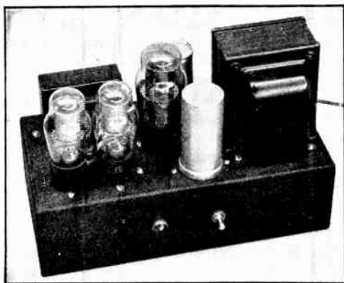
Fig. 1382 — Voltage-regulated power supply for the v.f. exciter unit. L_2 is mounted underneath the chassis.
