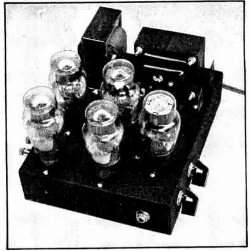
Fig. 1391 — A vacuum-tube keyer, built up on a 7 \times 9 \times 2-inch chassis with space for four or more keyer tubes and the power-supply rectifier. The resistors and condensers which produce the lag are mounted underneath, controlled by the knobs at the right. The jack is for the key, while terminals at left are for the keyed circuit.
