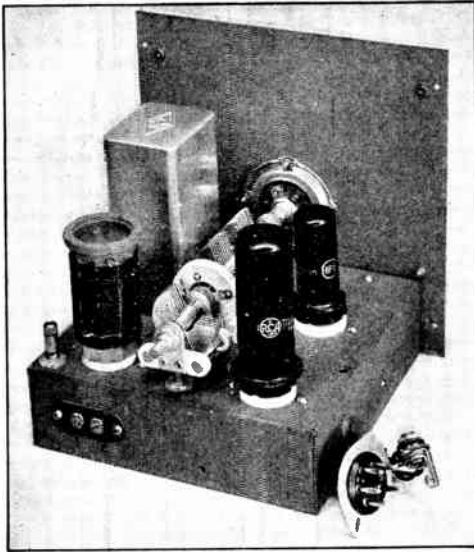
Fig. 1379 — Components for the v.f.o. exciter are assembled on a 7 × 7 × 2-inch chassis. The dual-section condenser is mounted by removing the shield between sections and fastening to the chassis with a single machine screw. The smaller condenser, C 7 , is mounted on National polystyrene button insulators and metal spacers to insulate it from the chassis and bring its shaft in line with that of the dual condenser. It is reverse-mounted, with its tail shaft extension coupled to the tail shaft extension of the dual condenser to reduce the overall mounting space. The stop pin on the shaft must be removed. Leads from the tuning condensers to the sub-mounted coil sockets pass through the chassis via 1/2-inch holes lined with rubber grommets. The jack for the key, which must be insulated, and the male power connector mount in the side of the cabinet. The chassis is fastened firmly in place with long machine screws running through the chassis and the bottom of the cabinet. The terminals at the rear are for link-output connections, the binding post for capacity coupling.
