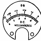
Fig. 2051 — A logarithmic field-intensity meter with db. calibration, employing a variable- \mu d.c. amplifier tube.
