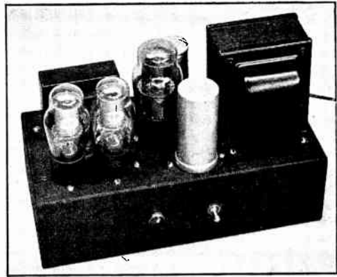
Fig. 1370 — Voltage-regulated power supply for the v.f. exciter unit. L_2 is mounted underneath the chassis.
