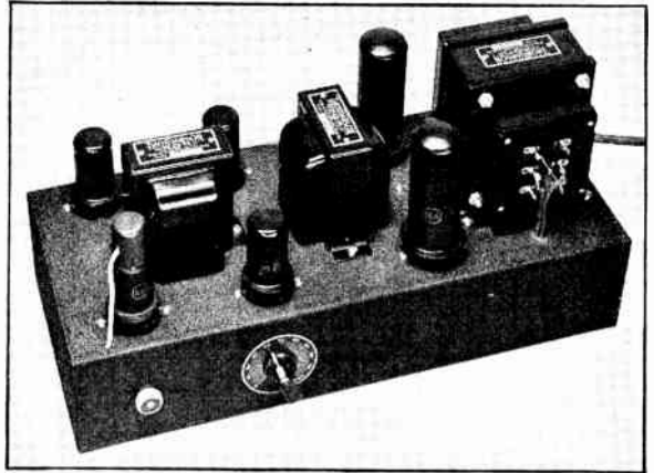
Fig. 1407 — A 40-watt speech amplifier or modulator of inexpensive construction. The 6J7 and first 6J5 are at the front, near the microphone socket and volume control, respectively. T 1 is behind them, and the push-pull 6J5s are at the rear of the chassis behind T 1 . T 2 , in the center, the push-pull 6L6s, and T 3 follow in order to the right.
