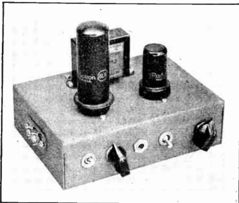
Fig. 1726 — A Class-A 6L6 choke-coupled modulator, using a minimum of transformers. The controls along the front are, left to right, the send-receive switch, 'phone-c.w. switch, key jack, microphone battery switch, and gain control. Terminals for external microphone battery are on the left edge. The microphone jack, not visible, is mounted on the right-hand edge of the chassis.
