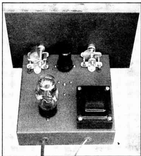
Fig. 1911—Top view of the superheterodyne carrier-current converter. Note the adjusting screw for the output tank condenser, C_6 , in front of the 6SA7 tube.
