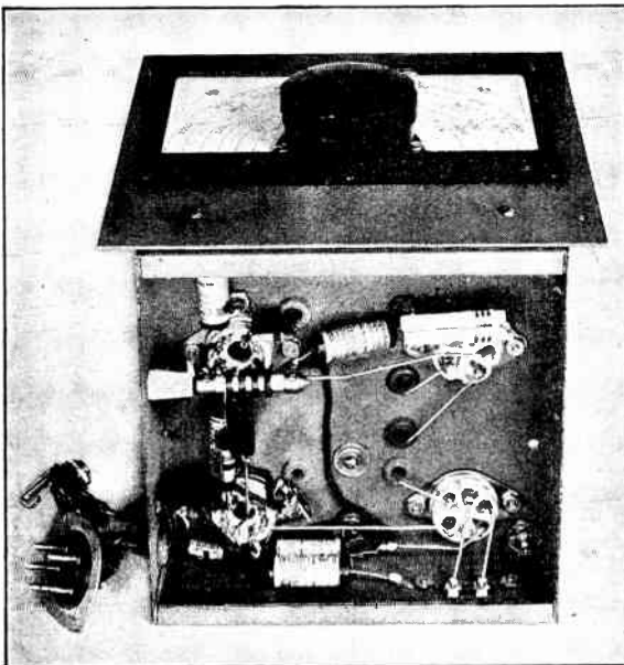
Fig. 1367 — High-frequency connections underneath the chassis of the v.f. exciter unit are made with short, straight sections of heavy wire. The two zero-temperature padding condensers are soldered directly to the oscillator-coil socket. All components are mounted firmly with no opportunity to support mechanical vibration. Washers \frac{1}{16} -inch thick are placed between the panel and the chassis to provide space for the lower lip of the cabinet opening.
