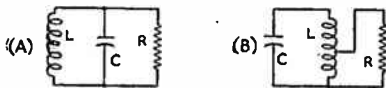
Fig. 241—The equivalent circuit of a resonant circuit delivering power to a load. The resistor R represents the load resistance. At (B) the load is tapped across part of L , which by transformer action is equivalent to using a higher load resistance across the whole circuit.
