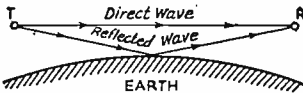
Fig. 902 — Showing how both direct and reflected waves may be received simultaneously in v.h.f. transmission.
