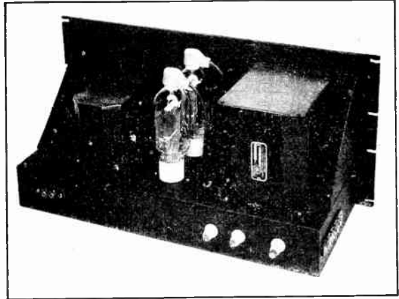
Fig. 1414 — A conventional chassis arrangement for low- and medium-power Class-B modulator stages. The mechanical layout in general follows the typical circuit diagrams given in Fig. 1313.
