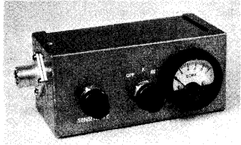
Fig. 21-48—This is the completed Millimatch. At the left is the sensitivity control, R_6 . S_1 is in the center, and Q_1 at the right.
