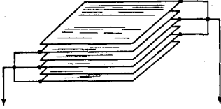
Fig. 2-9—A multiple-plate capacitor. Alternate plates are connected together.
