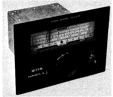
Fig. 6-51—The FET v.f.o. The panel is \frac{1}{8} -inch aluminum, 7 by 10 inches. (Designed and built by G. D. Hanchett, W2YM.)
