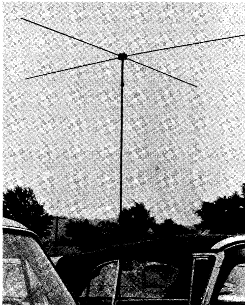
Two-meter turnstile antenna shown mounted on the front of an automobile. The miniature coax cable which feeds the antenna is taped to its \frac{1}{4} -inch diameter steel supporting rod. The ends of the antenna elements should be flattened, or rounded, to make them safer in the event of accidental contact with the human body.
