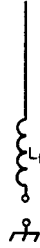
Fig. 19-31 — The capacitive reactance at frequencies lower than the resonant frequency of the whip can be canceled out by adding an equivalent inductive reactance in the form of a loading coil in series with the antenna.
