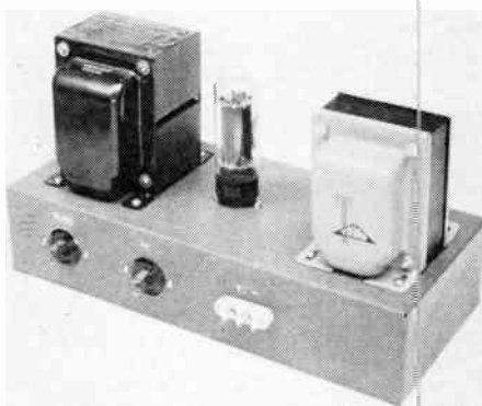
Fig. 7-33—A typical low-voltage power supply. The two a.c. connectors permit independent control of filament and high voltage.
