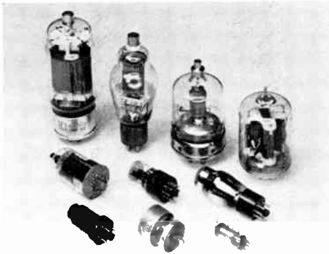
Representative tube types. Transmitting tubes having up to 500-watt capability are shown in the back row. The tube with the top cap in the middle row is a low-power transmitting type. Others are receiving tubes, with the exception of the one in the center foreground which is a v.h.f. transmitting type.
