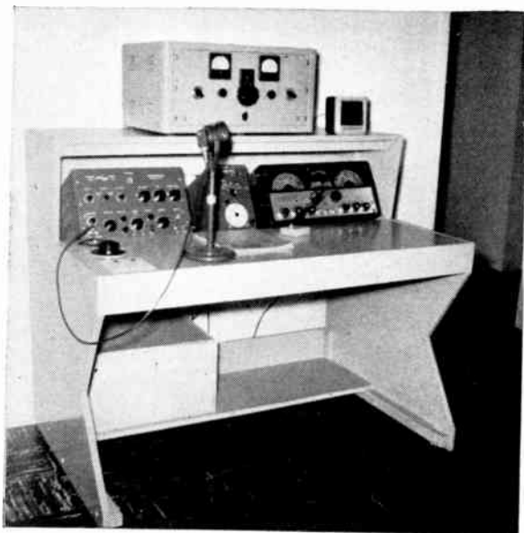
Here's an operating console that was designed with operating convenience in mind. W7EBG built it almost entirely out of \frac{3}{4} " plywood, with strips of 2 X 2 along the bottom edges for caster supports. It is assembled with bolts so that it can be readily dismantled for shipping. Over-all dimensions are 48" wide, 40 \frac{1}{2} " high, with the horizontal desk top 16" wide and the sloping portion 15" wide.
