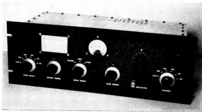
Fig. 6-51—Controls, from left to right, are for band switch, exciter tuning, meter switch, pi-section tank capacitor, rotary inductor and turns counter, and output-capacitor switch. The panel is 7 by 19 inches. The top cover (a chassis bottom cover) is in place in this view.
