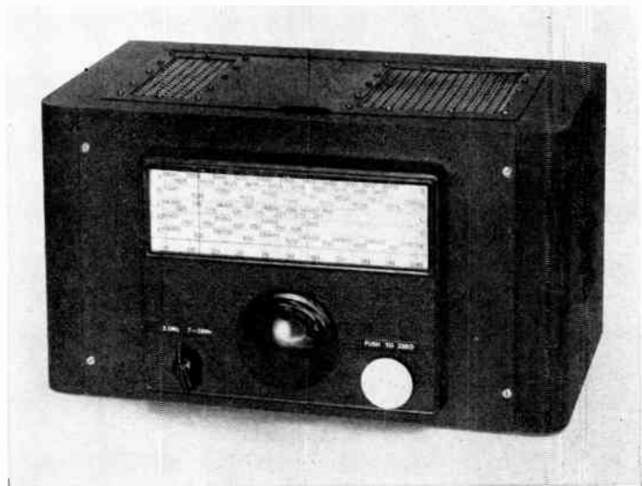
Fig. 6-90—The v.f.o. unit mounted in its cabinet. Holes are drilled in the dial cover to accommodate the switch shafts. At the right, a poker chip has been cemented to the v.f.o. set push-button switch so that it can be operated while tuning the v.f.o.
