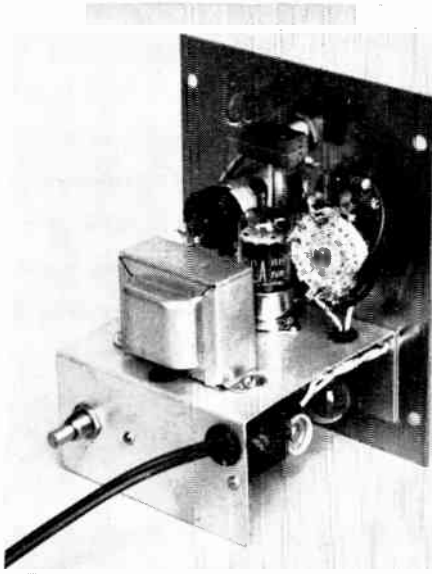
Fig. 21-24—Inside view of the audio oscillator. The a.c. switch, S_3 , is mounted on the output control at the left on the panel. The ceramic capacitors in the frequency-determining circuits are mounted on the rotary switch, S_1 , at the right. S_2 is above the tube, and T_1 is on the near edge of the chassis, which is a U-shaped piece of aluminum 3\frac{1}{2} inches deep with 1\frac{1}{2} inch lips. R_1 is mounted on the near lip at the left.
