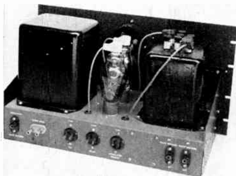
Fig. 9-26—A typical Class B modulator arrangement. This unit uses a pair of 811As, capable of an audio power output of 340 watts, and includes a splatter filter. The modulation transformer is at the left and the splatter choke at the right. All high-voltage terminals are covered so they cannot be touched accidentally.
