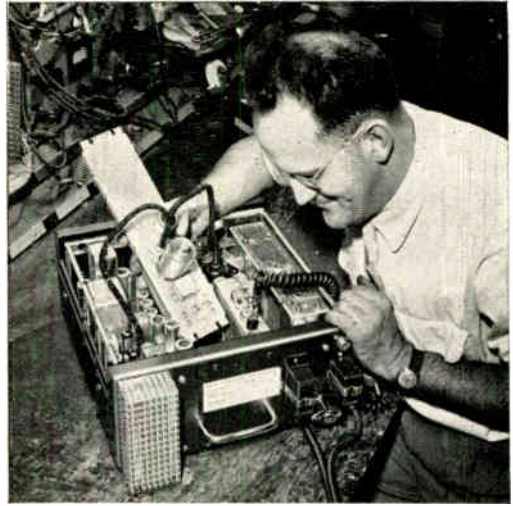
G-E Service Station operator Floyd Ziehl, W2RUI, a second class Commercial Radio Operator and 30-year amateur veteran, installs new 450 mc pre-amplifier containing General Electric's new 7077 micro-miniature tube in a mobile unit. Servicemen are kept up-to-date on new and advanced units like this by a constant flow of information from the General Electric National Service Manager.
