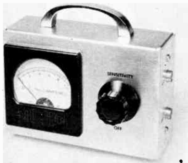
Fig. 19-40—A front view of the field-strength meter. Sensitivity control R_1 is to the right of the 0-1 indicating meter. Antenna input and output connectors are mounted on the right end of the box.
