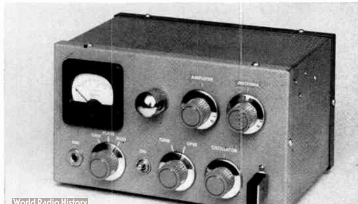
Fig. 19-14—A panel-illuminating lamp is mounted to the right of the meter, along with the amplifier-tank and antenna-link tuning controls. Along the bottom, from left to right, are the microphone jack, meter switch, filament switch, tune-operate switch, oscillator tuning control and the crystal.
