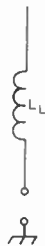
Fig. 19-33—Placing the loading coil at the center of the whip antenna, instead of at the base, increases the radiation resistance, although a larger coil must be used.
