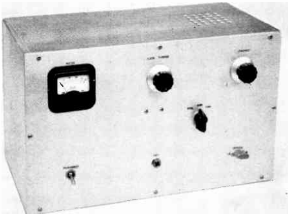
Fig. 6-35—This 30-watt three-band Novice transmitter is enclosed in a 7 \times 9 \times 15 -inch aluminum box. A group of \frac{1}{4} -inch-diameter holes should be drilled in the top of the box over the oscillator tube, as shown, to provide ventilation. A similar set of holes should be drilled in the back cover behind the oscillator circuit.
