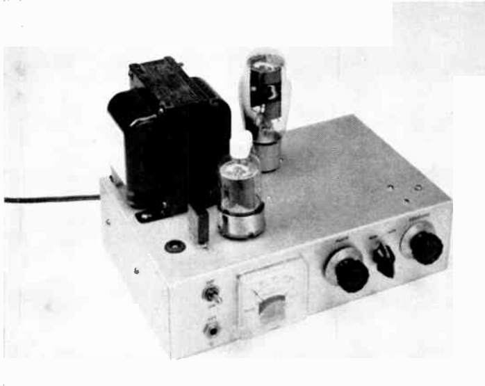
Fig. 6-39—This view of the 50 wattter shows the panel arrangement and layout of the components above chassis. The crystal is between the 6146 and dial-light grommet. Behind the 6146 is the power transformer and to its right is the rectifier tube.
