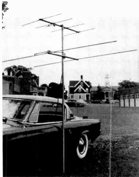
Fig. 18-5—Two-element 50-Mc. and four-element 144-Mc. arrays designed for portable use. Support is sectional TV masting clamped to car door handle. Elements of 50-Mc. array are made in three sections, far stowing in back of car. Antenna for 144 Mc. is cut-down TV array. Both use gamma match, as shown in Fig. 18-6.
