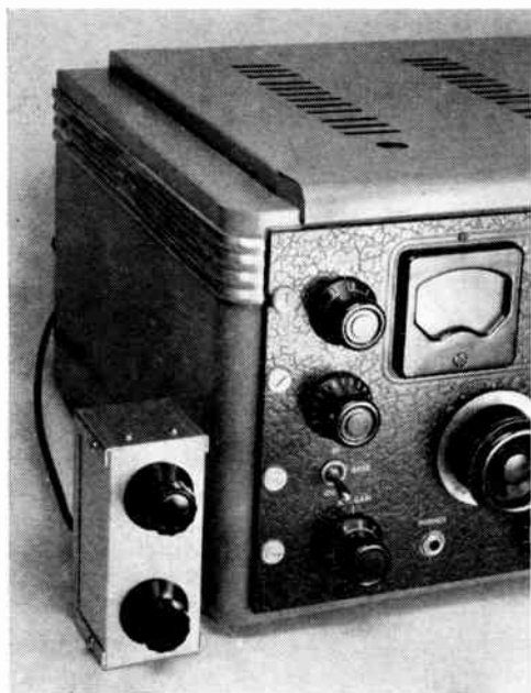
Fig. 5-64—View of the Q multiplier showing its single connecting cable to the receiver. The box can be placed in any convenient spot on or around the receiver.
