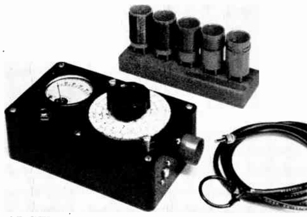
Fig. 21-11—The indicating frequency meter, plug-in coils, and pick-up cables. The meter is built in a bakelite meter case measuring 6\frac{1}{4} \times 3\frac{3}{4} \times 2 inches. The 3-inch dial is cut from a piece of aluminum and has a paper hand-calibrated scale cemented on. Hairline indicators are clear plastic mounted on small metal pillars. A 2-inch d.c. instrument is used. Pick-up loops are one turn of No. 14, spaghetti covered, soldered to the ends of the cables. The longer cable (5 feet) is useful to 30 Mc.; the shorter (13 inches) can be used for the full frequency range. Both are RG-58/U.
