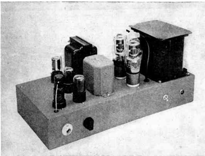
Fig. 9-33 — A speech amplifier and 807 modulator for plate modulation of transmitters up to 200 watts input. The microphone jack and the gain control are at the left end of the chassis. The audio components and tubes occupy the front section and the power supply for the driver tubes is laid out along the rear edge.
