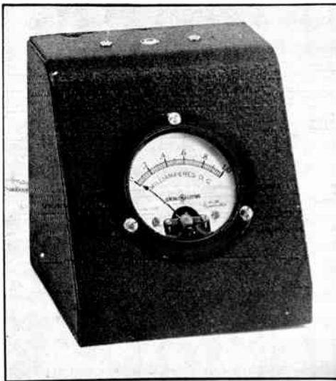
Fig. 5-39 — Front view of the signal-strength indicator. The 0-1 milliammeter is mounted in a metal meter case. The zero-adjustment potentiometer, R 4 , is mounted below the top of the cabinet by means of a "U"-shaped bracket; the potentiometer shaft is slotted so that it can be adjusted with a screwdriver. A new face, calibrated in S-units, can be pasted to the 0-1 ma. scale, or a calibration chart can be attached to the cabinet.
