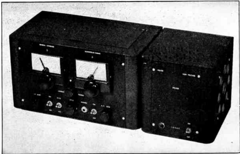
Fig. 5-33 — A front view of the six-tube receiver. The general-coverage and the band-spread-tuning dials are to the left and right of the panel. The antenna trimmer condenser is centered below the main tuning dials. The i.f. gain control, noise-limiter switch, a.v.c.-b.f.o. switch, b.f.o. pitch control, head-phone jack, stand-by switch, and a.f. gain control are shown from left to right across the bottom of the panel. A suitable power supply for the receiver is mounted in the 'speaker cabinet shown at the right of the receiver.
