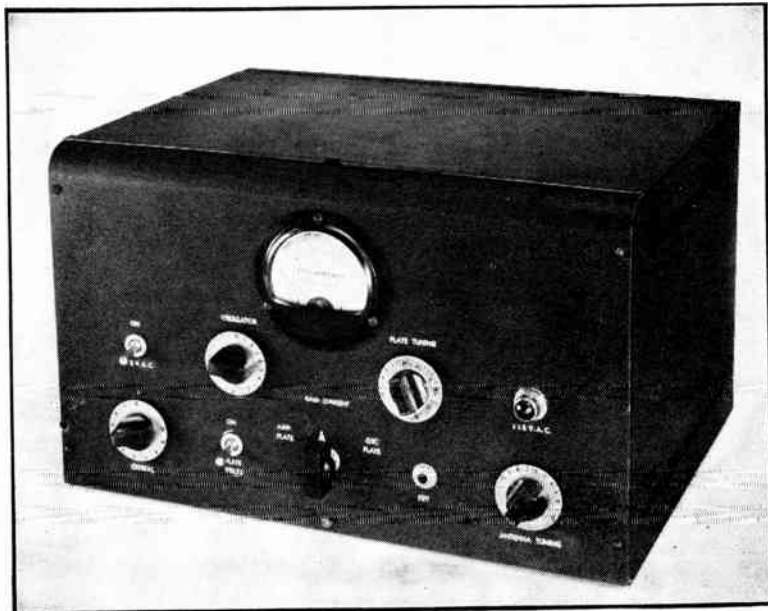
Fig. 6-42 — A two-stage 60-watt transmitter for three bands. To either side of the milliammeter are the oscillator and amplifier plate-tuning controls. Along the bottom are the crystal switch, the plate-voltage switch, the meter switch, the key jack and the antenna tuning control.
