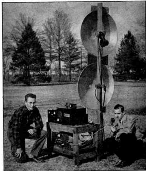
Fig. 15-36 — The first amateur microwave communication was accomplished by W6BMS (left) and W2LGF, who used two sets of similar equipment to open the 5300-Mc. amateur band on November 15, 1945, the date that the first microwave bands were released for amateur use.
