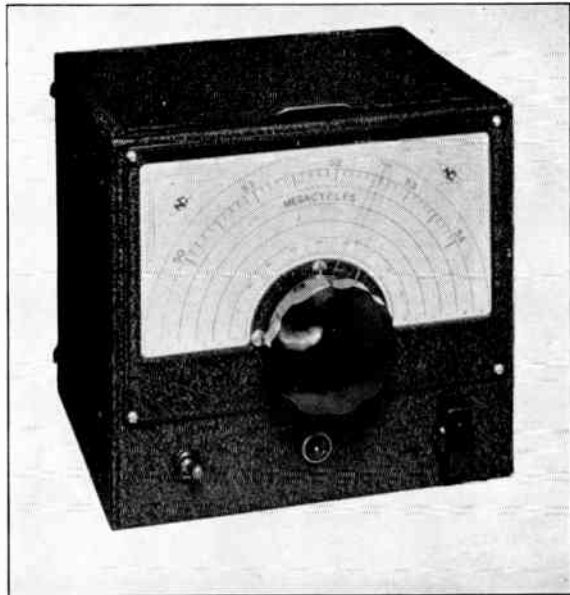
Fig. 12-8 — This two-tube 50-Mc. converter incorporates miniature tubes and obtains its power from the communications receiver with which it is used. The toggle switch at the left cuts the filament circuit when the unit is not in use. The control at the lower right transfers the antenna from the converter to the receiver for normal reception.
