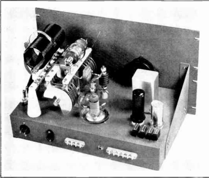
Fig. 6-63—Rear view of the two-stage high-power transmitter, showing the vacuum-type padding condenser in place on top of the tank condenser.
