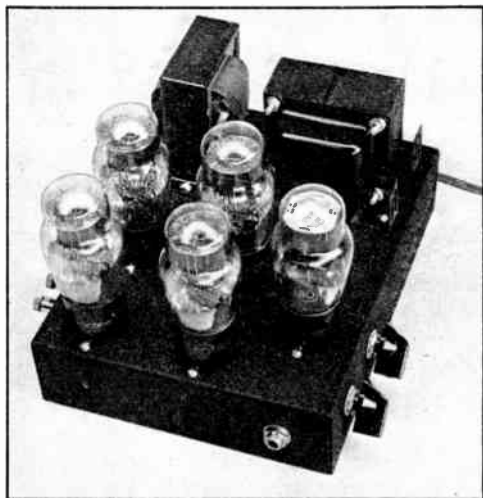
Fig. 8-9 — A vacuum-tube keyer, built up on a 7 × 9 × 2-inch chassis with space for four or less keyer tubes and the power-supply rectifier. The resistors and condensers which produce the lag are underneath, controlled by the knobs at the right. The jack is for the key, while terminals at the left are for the keyed circuit.
