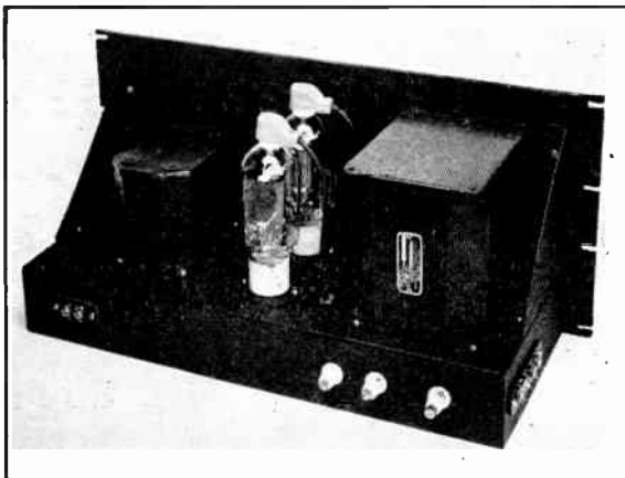
Fig. 9-41 — A conventional chassis arrangement for low- and medium-power Class B modulator stages. The mechanical layout in general follows the typical circuit diagrams given in Fig. 9-40.
