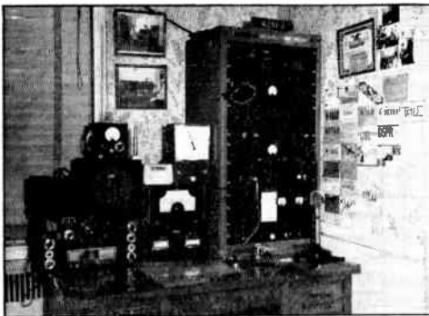
An example of the compact station, complete on the operating table. The receiver is mounted on the left side of the table, for left-hand tuning. The beam-direction indicator and switches are housed in a small box sitting on the YFO. (W2NFL, Forest Hills, N. Y.)
