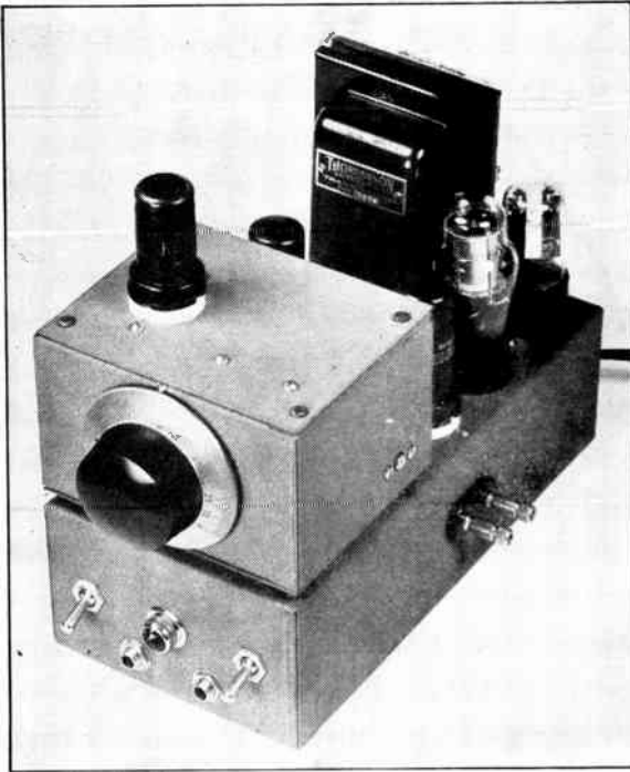
Fig. 6-74 —The complete VFO unit. The oscillator is housed in a separate compartment which is shock-mounted on rubber grommets. The oscillator tube is on top of the compartment. To the rear are the two 6F6 amplifier tubes, the VR tube, the rectifier and the power transformer. In front are the stand-by switch, the power switch, pilot lamp and the two keying jacks. The output terminals are to the right.
