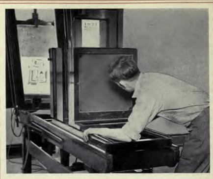
THE first step in making an engraving is shown above—photographing the original. Below, the etcher has just taken the zinc plate out of the acid bath after a "bite."
