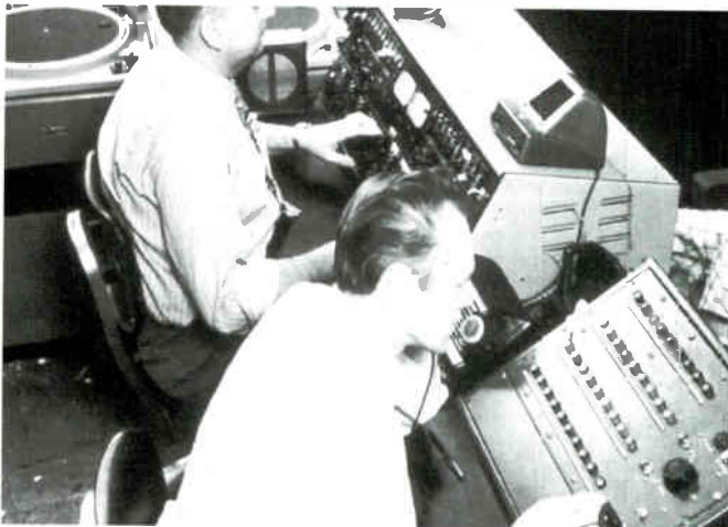
Master control of WGEM TV in 1954 was primitive by today's standards. The video switcher is in the foreground with the audio console behind. The turntables were available to play music during the frequent technical problems and program interludes.
