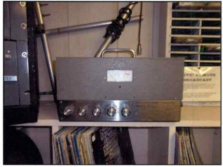
View of "Marti" FM Remote Pickup Unit used for the remote broadcasts of KWNS. Invented by George Marti. Marti Electronics, beginning in 1960, manufactured the model M-30BT fulltime in Cleburne, Texas. The "Marti" was specially designed for use within a 10-15 mile radius from the station. Located behind is the Loop antenna and coax line for the unit. "Marti" remote unit currently preserved and on display at the Pratt County Historical Society Museum. Photo Courtesy: Ron Detwiler
