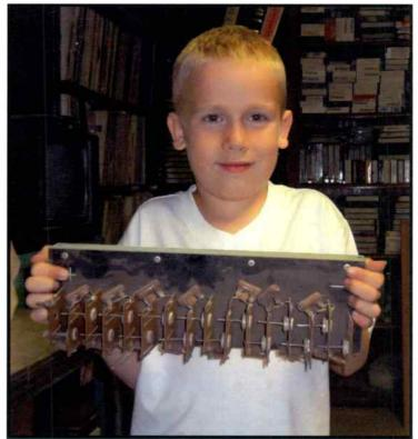
Anthony Detwiler holding a power supply rectifier board for the Gates FM-5G FM transmitter.
