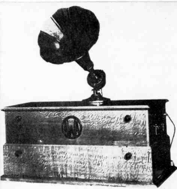
On sale in 1926 for £90 was the Radiola Super Six, a six-valve super heterodyne receiver, capable of receiving stations from Adelaide to Brisbane
