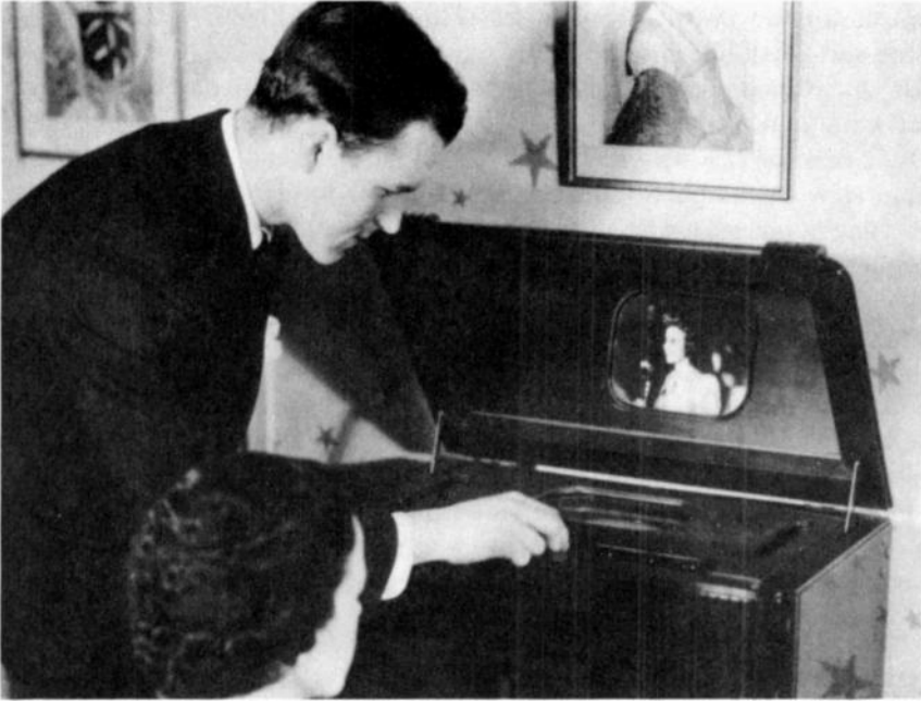
An RCA television receiver, its picture viewed in a mirror in the upraised cabinet top, 1940. (Courtesy of the Library of Congress)
