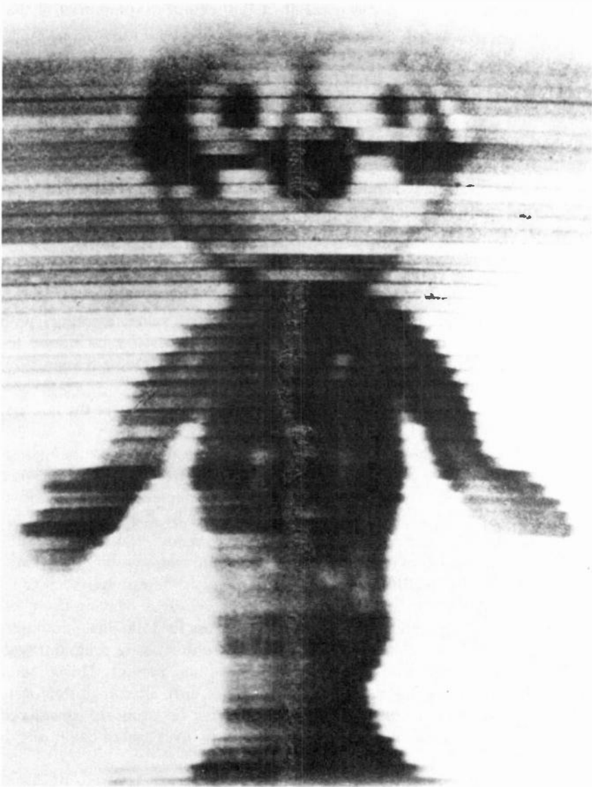
Felix the Cat as he looked in the 60-line pictures that appeared on the screens of television receivers during a 1928 telecast by RCA-NBC. (Courtesy of RCA)
