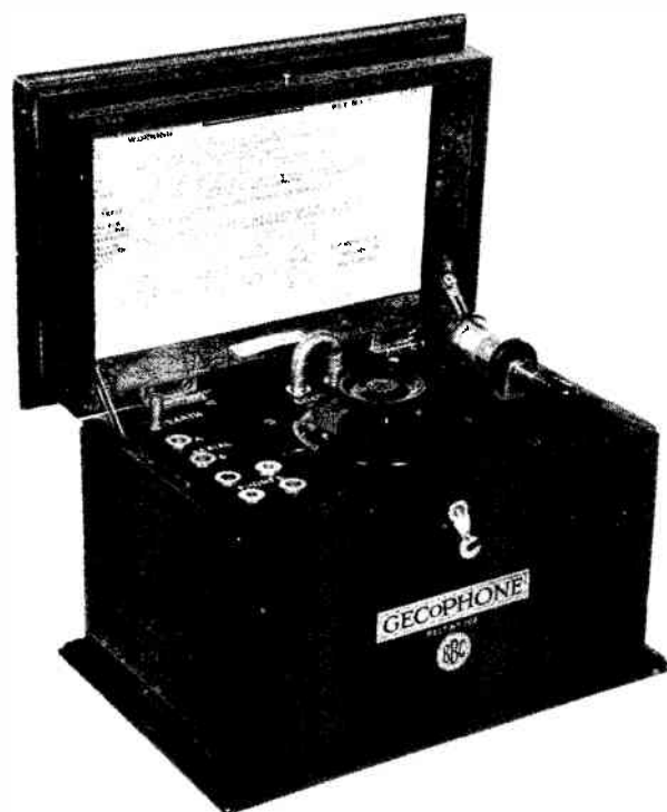
fig. 39. Gecophone Model No.1 Type BC 1002, by General Electric Co. Ltd. 1922. BBC/PMG Stamp, GPO Reg.No.102. Crystal set for headphone use, glass-enclosed cat's whisker/galena detector (open detector version also known), provision for plug-in coils, variometer tuning, ebonite control, nickel-plated fittings, mahogany box with lift-up lid. 6 ¼ in. x 9 in. x 6 in. (closed). £5.10s.0d.
