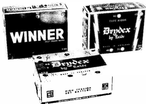
fig.44 . High tension ("HT") batteries, which were also known as 'primary' batteries, were necessary to provide the valves with anode voltage, and comprised a large number of series-connected 1\frac{1}{2} volt dry cells usually arranged neatly in a strong cardboard box and well sealed in with paraffin wax or pitch to form a single unit. Depending on the valves and the type of receiver used, HT batteries in sizes from 45 volts to as much as 180 volts were available, and these were provided with tappings taken from groups of cells at regular intervals so that variations in voltage could be obtained as desired. While being non re-chargeable, a good quality HT battery could, with average use, last for about three to four months and in 1922, one of 60 volts in a 3\frac{1}{2} in. x 9 in. x 2\frac{3}{4} in. container cost around £1.0s.0d. HT batteries were sometimes made up of series-connected accumulators, but these were usually used only by listeners who were in a position to do their own re-charging or had a regular collection and re-charging service. The HT batteries in the photograph date from the 1930s.
