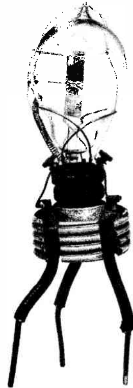
fig. 14 . 'Fleming Diode'. c.1904. An experimental 'diode', used as a detector and rectifier of wireless signals. Turned boxwood socket, brass terminals. 8¾ in. high x 2¼ in. diameter.
