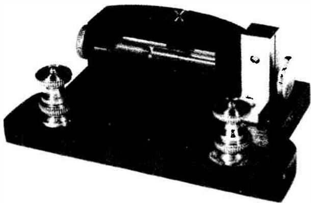
fig. 11 . 'Italian Navy' Coherer. c.1899. A 'self-restoring' mercury-iron coherer, originally devised by P. Castelli, a signalman in the Italian Navy. The illustration shows the original one used by Marconi during his transatlantic wireless telegraphy tests of 1901. Ebonite base, brass fittings, glass tube containing an iron plug and a carbon plug bridged by a globule of mercury. Base, 1\frac{1}{4} in. x 3\frac{1}{4} in. 2 in.
