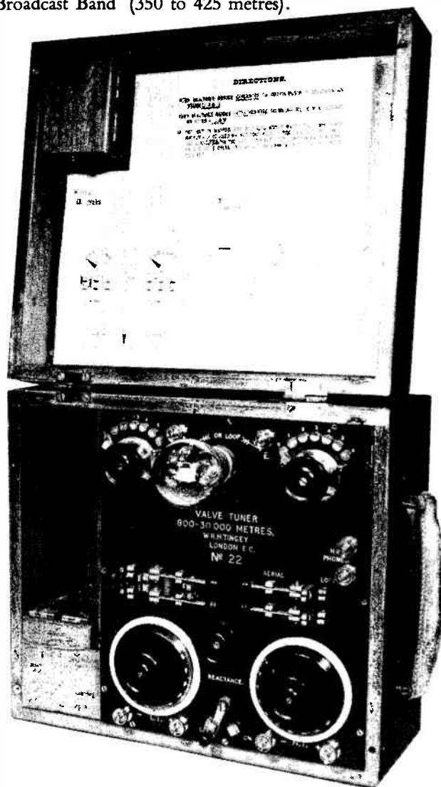
fig. 35 . Tingey 'Valve Tuner No.22', by W.R.H. Tingey, London EC. 1920. A 1-valve battery receiver for headphone use, tuning between 800/30,000 metres. Made using parts from surplus 'Mark III Short Wave Tuners' (fig. 27). Canvas-covered mahogany case, 8 in. x 14 in. x 12 in.
