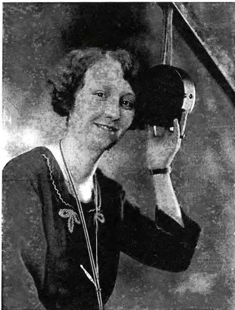
The glow-discharge microphone that was used in the broadcast of a human heartbeat.
