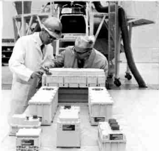
Boxes containing voice portion of the Apollo command module communications system are examined by North American Space Division personnel.
