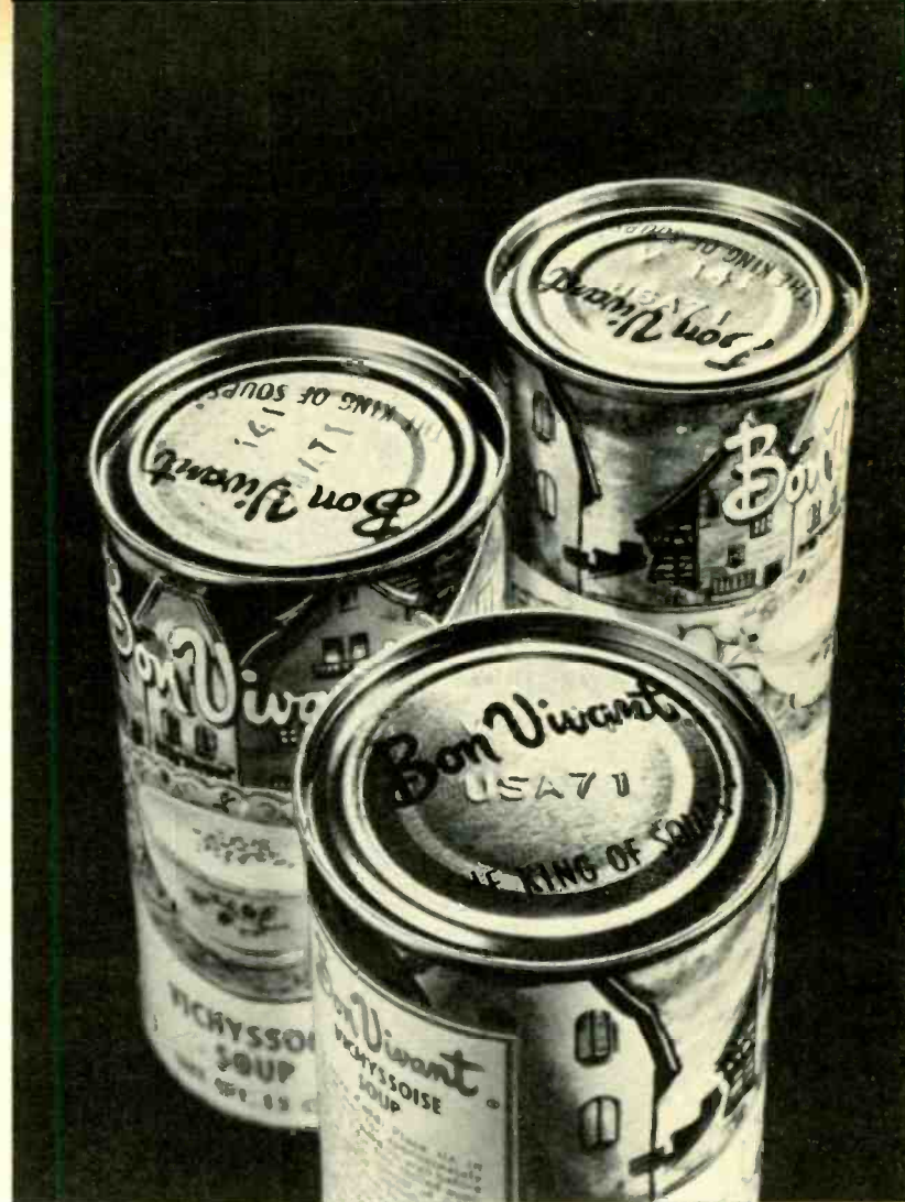
The top of the bad can in foreground, above, is slightly swollen due to pressure from gases inside, while normal cans at rear have indented tops. If food sprays out when a can is opened, as shown below at FDA's New York laboratories, the entire contents of the can should be discarded without tasting.
