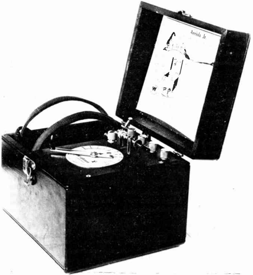
Fig. 32. First popular-priced home radio set, the Aerola Jr. used headphones and cost $25. Courtesy of Radio KDKA.
