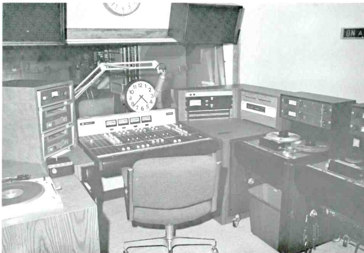
A Harris M90 console is shown in the new studios of Station WKEZ-FM, Norfolk, Virginia, where it is used as an on-air and a production board... often simultaneously.
