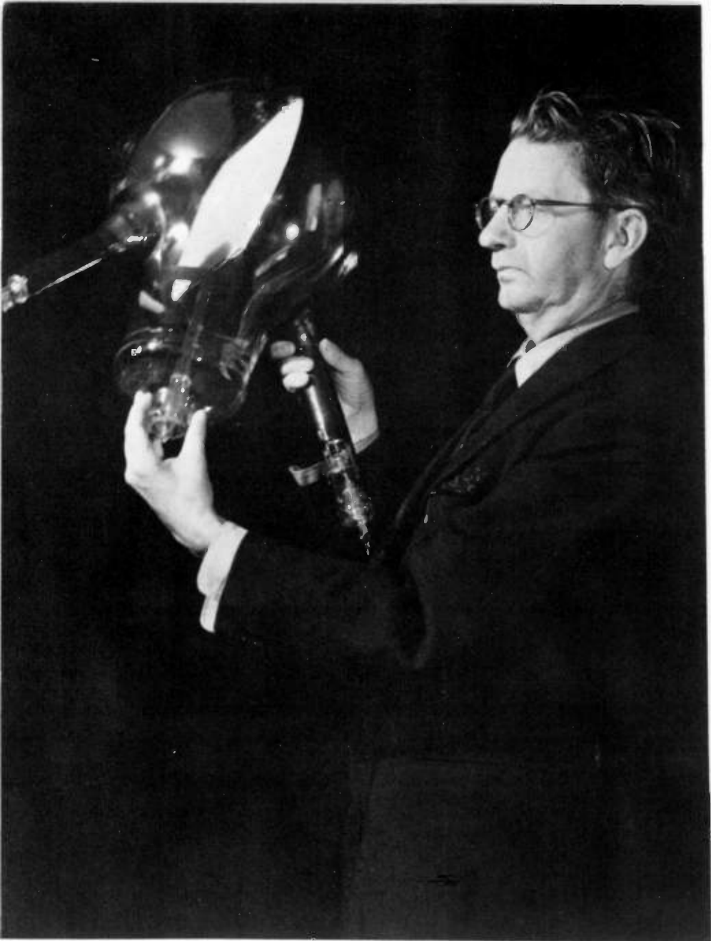
John Logie Baird demonstrating in 1939 the large cathode-ray tube which he named the Telechrome. The apparatus produced a three-dimensional picture in colour
