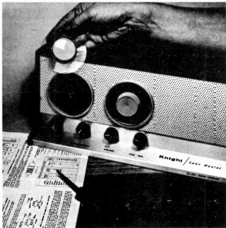
Fig. 4-3. Knight-Kit Span Master is an inexpensive regenerative receiver which can be assembled at home.
