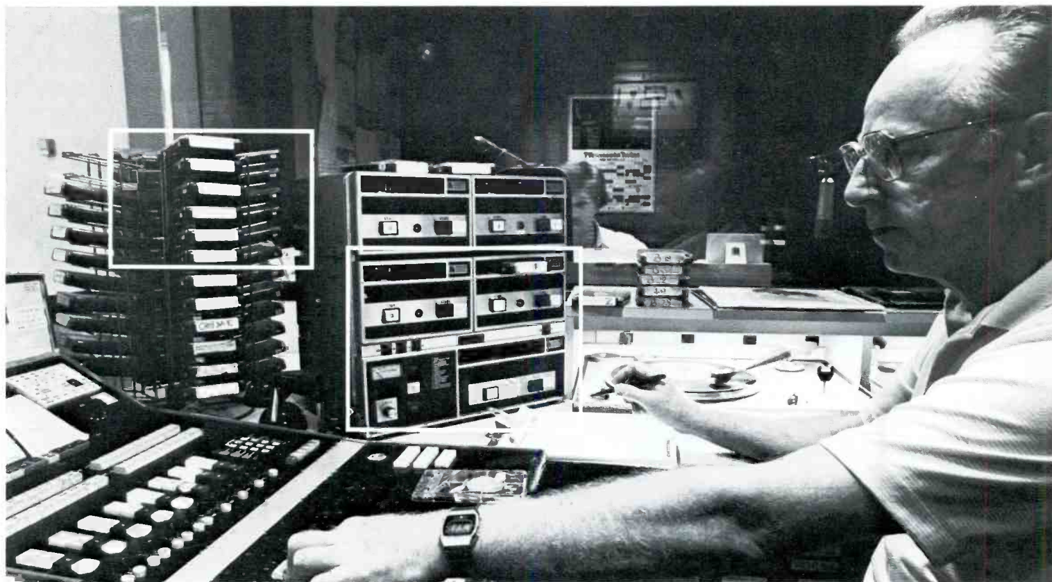
From the control room, technician Art Johnson can operate tape recorders, turntables, cassette cartridge players, telephone lines, and all of his other equipment.
