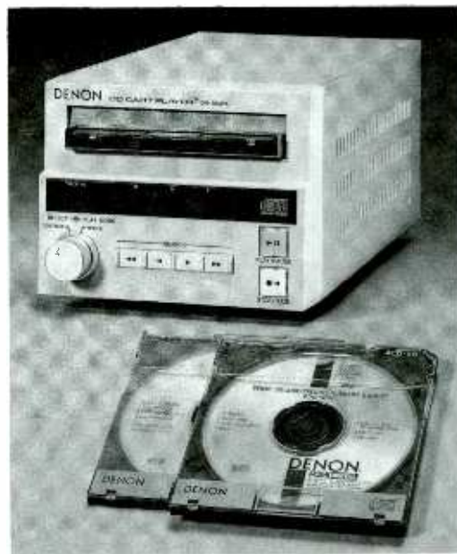
FIGURE 9.20 CD cart players are popular in both the on-air studio and the mixing room. Courtesy Denon.
