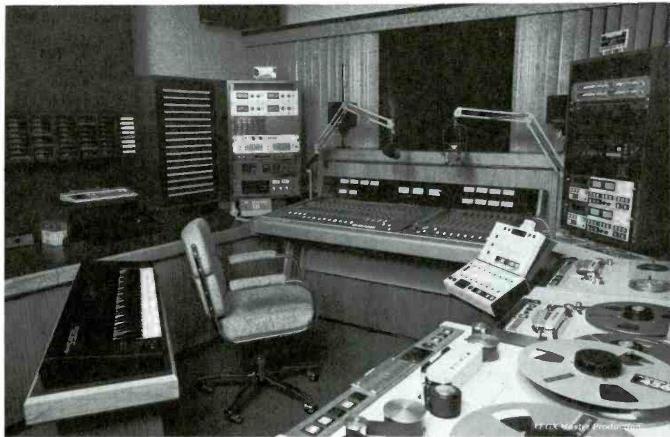
FIGURE 9.4 Although each production studio is unique, the basics of layout are fairly consistent from station to station. For the sake of ease and accessibility, most studios are developed in a U shape or a variation thereof. Courtesy WEGX and WHJJ/WHJY.
