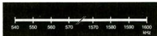
FIGURE 10.11 Standard AM and FM band. From FCC Broadcast Operator's Handbook , figs. 4-7 and 4-8.
