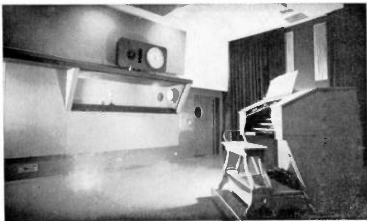
View within an organ studio and looking toward the control booth. Notice the adjustable curtains over the straight, flat wall of the "live end" of the studio.
