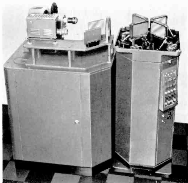
RCA TP-15 universal multiplexer showing vidicon camera and slide projector
