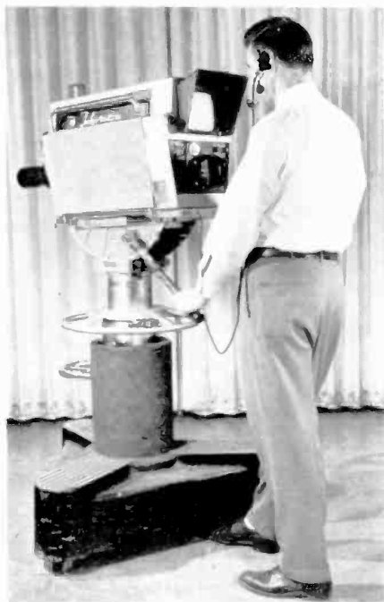
RCA TK-12 image orthicon camera with 4½-inch tube and pedestal
