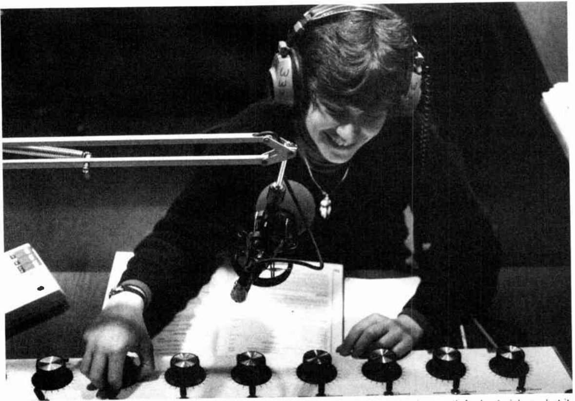
Fig. 2-4. Proper microphone placement—top view. The microphone must be aimed at the mouth for best pickup, but it need not be directly in front of the announcer. Positioning it a little off to one side will also work well. (Pictured: Carol Bozena in production studio of WWUH, West Hartford, CT)
