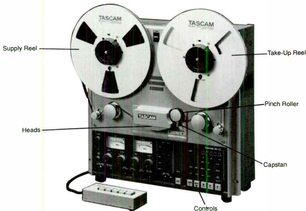
FIGURE 5.4 Audio tape recorder transport. (Courtesy of TASCAM Division, TEAC America, Inc.)
