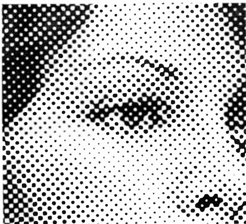
Figure 7-9 A halftone image is created using a screen process with different amounts of ink adhering to the printing plate. At a distance, the illustration becomes an eye. Close up we can see the various "dots" created by the halftone screen. In this halftone, both vertical and horizontal lines were used to create the screen, whereas in Figure 7-10, only vertical lines were used.
