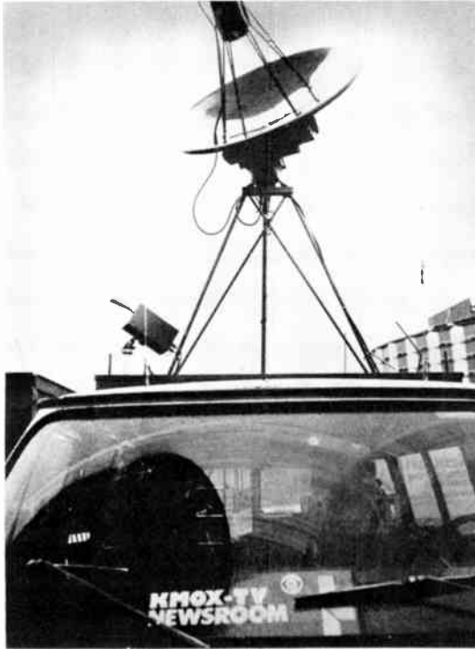
Figure 6-10 A microwave receiver is mounted on a mobile van alongside the larger dish for the link-up to the news center at the television station. (CBS)
