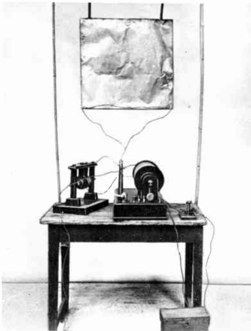
Figure 5-1 Marconi's early transmitting device used in the first experiments of wireless in Italy and later England. The large tin sheet served as the antenna. (The Marconi Company Limited, Marconi House, Chelmsford, Essex)
