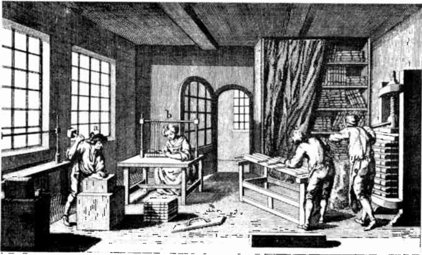
Figure 4-1 The early bookbinding shop shows the workers (left to right) beating the folded sections of the book, stitching the book, trimming the edges on a ploughing press (Figure 4-3), and pressing the edges on a standing press (Figure 4-4). (From DIDEROT and courtesy, The Printer in 18th Century Williamsburg . Williamsburg, Va.: Colonial Williamsburg, 1955)
