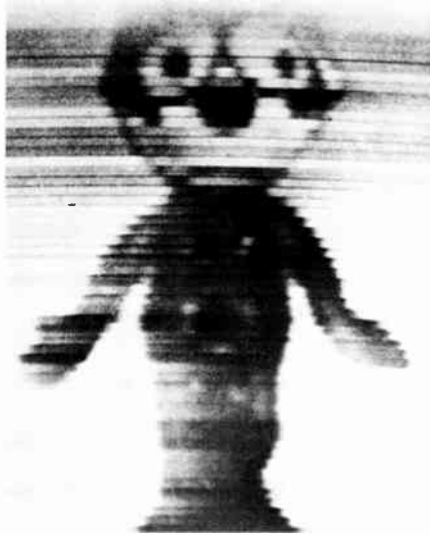
Figure 6-1 Felix the cat became television's first star as the crude scanning process resulted in a picture far inferior to modern transmission techniques. (RCA)
