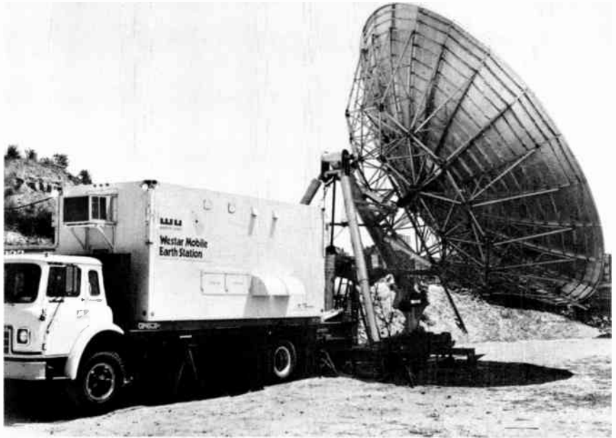
Figure 12-6 Satellite relay permits even greater flexibility to communicate over very long distances. The earth station can send and/or receive signals from a satellite in space, which in turn can relay signals to other earth stations thousands of miles away. (Western Union)
