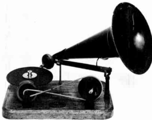
Figure 9-10 The Berliner gramophone of 1893, manufactured by the U.S. Gramophone Company of Washington, D.C., was one of the early disc phonographs on the market. Hand powered, it required the operator to crank the handle up to a speed of about 70 revolutions-per-minute in order to get a satisfactory playback. (Smithsonian Institution and the Recording Industry Association of America)
