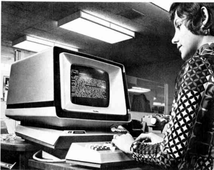
Figure 2-24 Visual display terminals (VDTs), also called cathode ray tubes (CRTs), are replacing the typewriter and becoming commonplace in major newspapers and other media. (Courtesy, Dow Jones & Company, Inc.)
