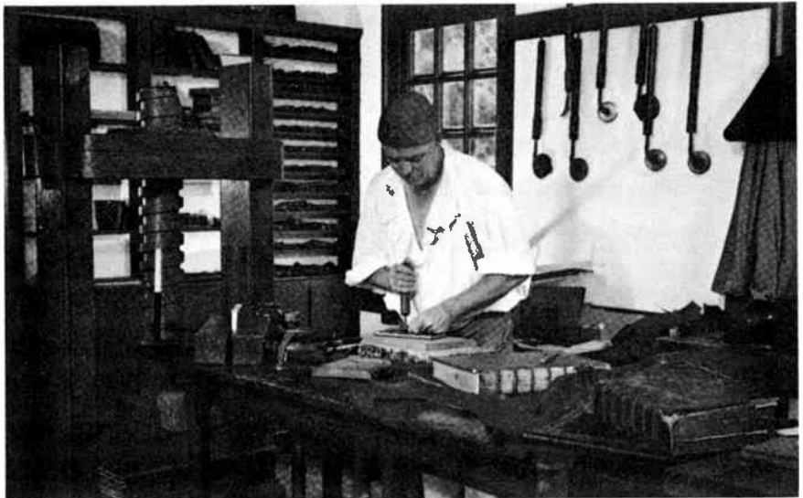
Figure 4-2 Notice in this illustration of a colonial bookbinder the hand tools on the back wall. The tools are used to “engrave” the ornate borders on leather bound books. The standing press is at the left, and immediately behind it are shelves with sheets of uncut leather. (Courtesy, Colonial Williamsburg)
