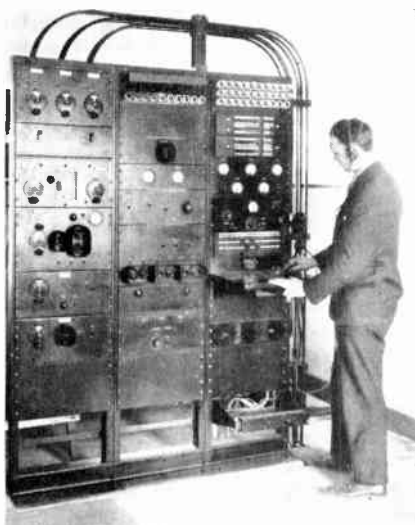
FIG. 16.—The type of receiver used by the American Telephone and Telegraph Company for transoceanic telephony. It is being monitored by an operator who is probably experienced in both Morse and Continental.
