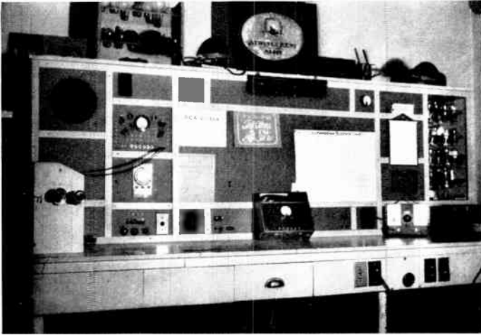
FIG. 5.—A modern service bench. By mounting the more important apparatus on removable panels, such test sets can be made to serve both as portable and shop equipment until business warrants duplication.
