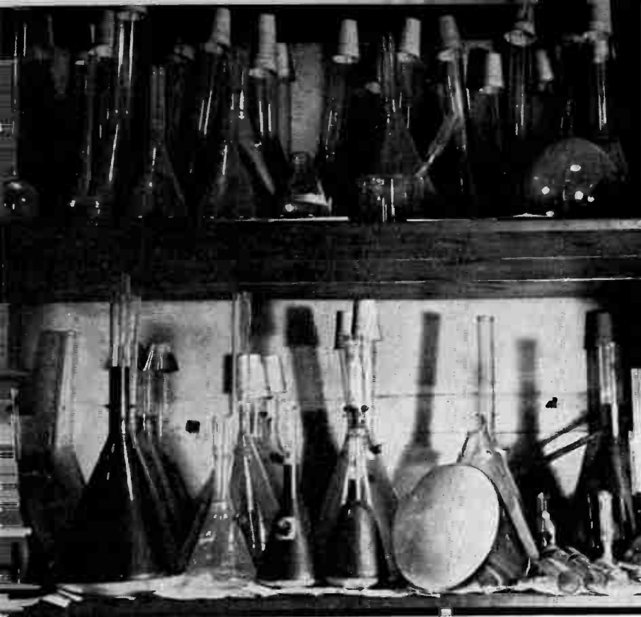
Experimental cathode ray tubes waiting to receive their electron guns. The tube at lower right shows the fluorescent material on the flat end
