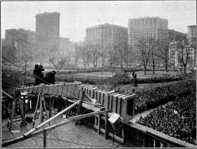
FIG. 1.—When, on Armistice Day, November, 1921, 155,000 people were enabled to hear President Harding's address at Arlington Cemetery, through public address systems, connected by wire lines at Arlington, New York and San Francisco, the world was amazed. Commercial radio programs reach ten times such numbers nightly in their own homes. ( Courtesy of Radio Broadcast. )
