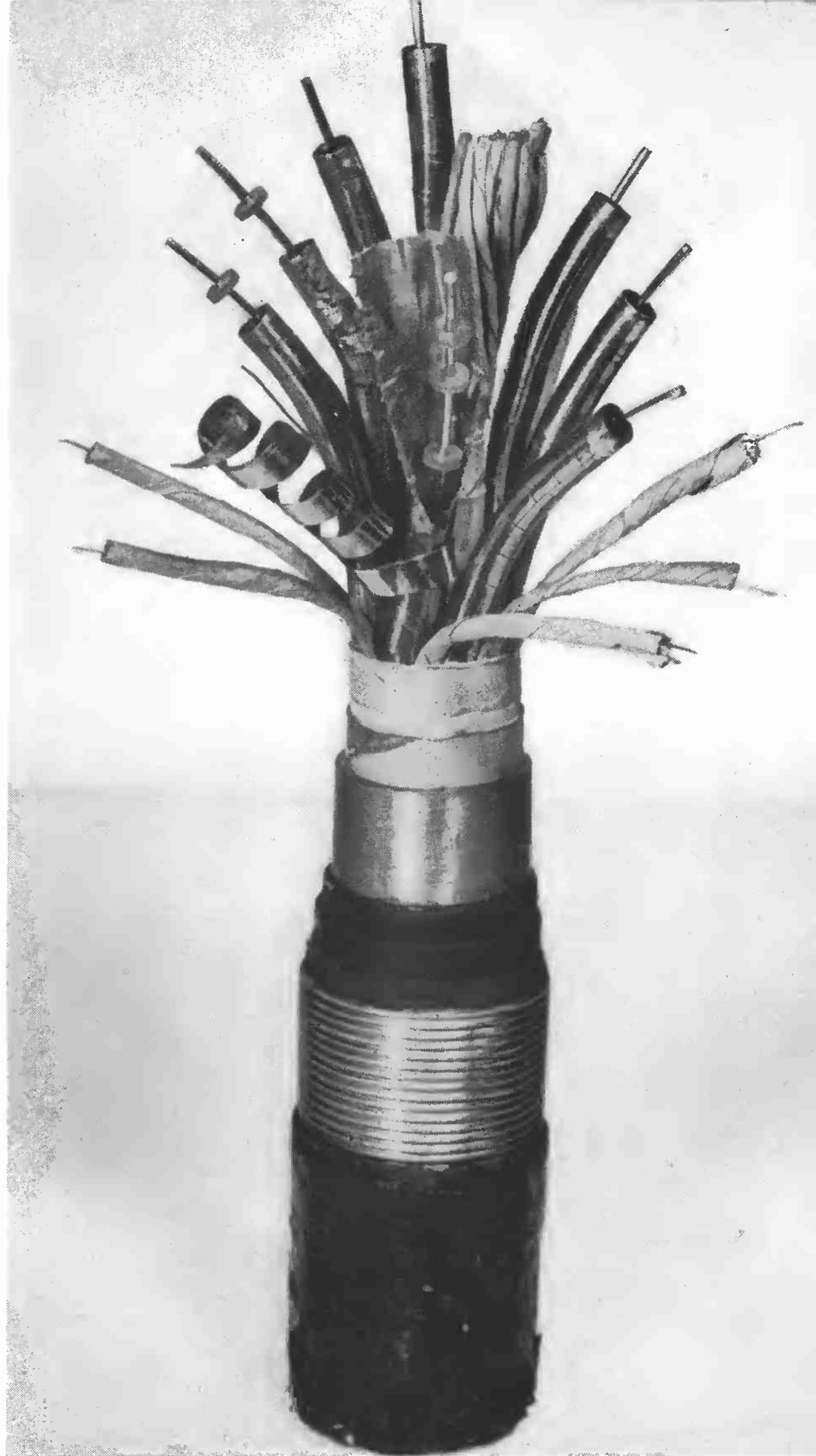
Typical coaxial cable showing the eight coaxial conductors (the large cylindrical tubes), and the secondary conductors which are used to carry control signals and power supply to the repeater or booster stations, located every 5 to 7 miles.
