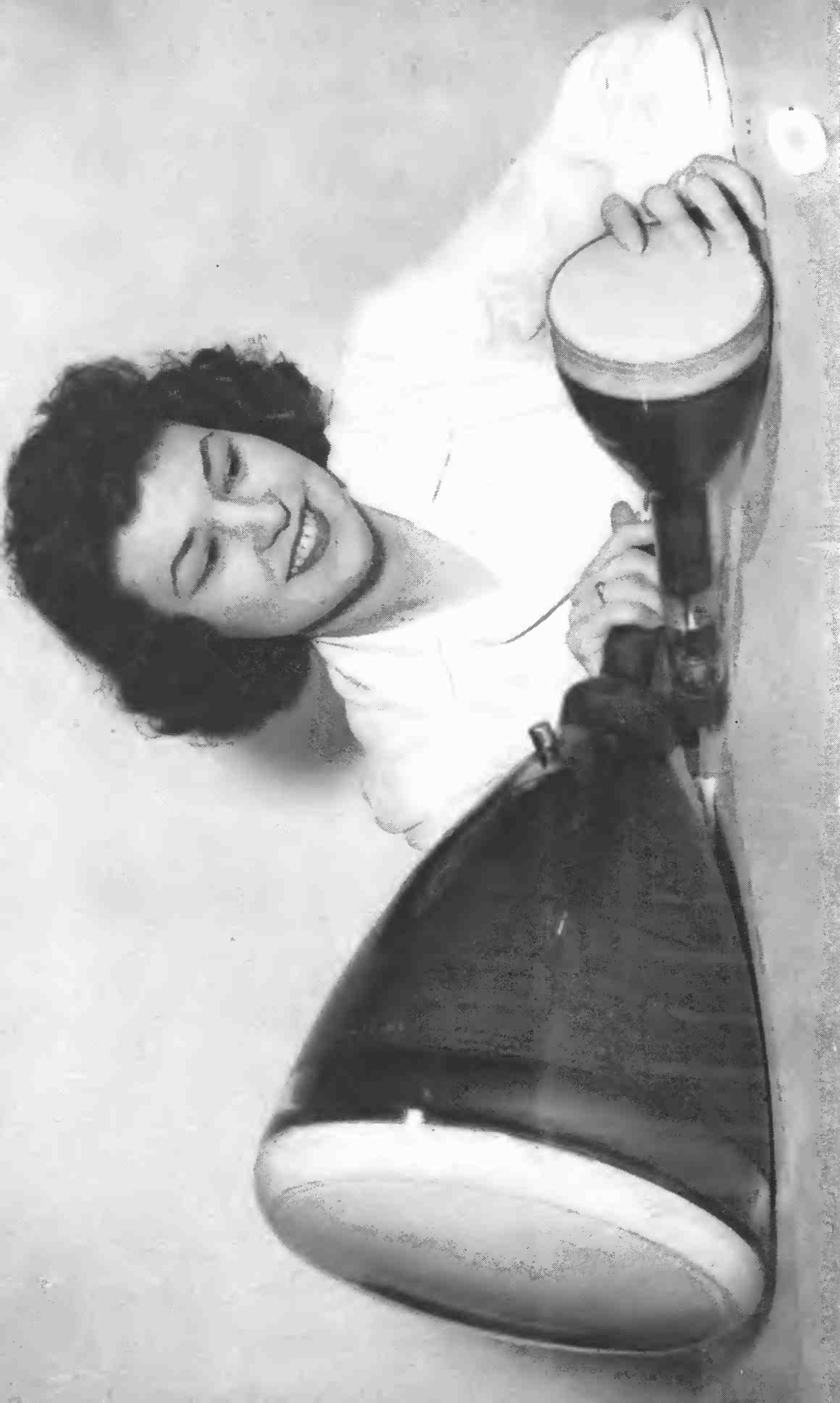
The kinescope, or picture tube, on the fluorescent face of which the television picture appears; an electron gun in the long neck of the tube generates, controls and focuses the electron beam that "paints" the picture on the "screen."
