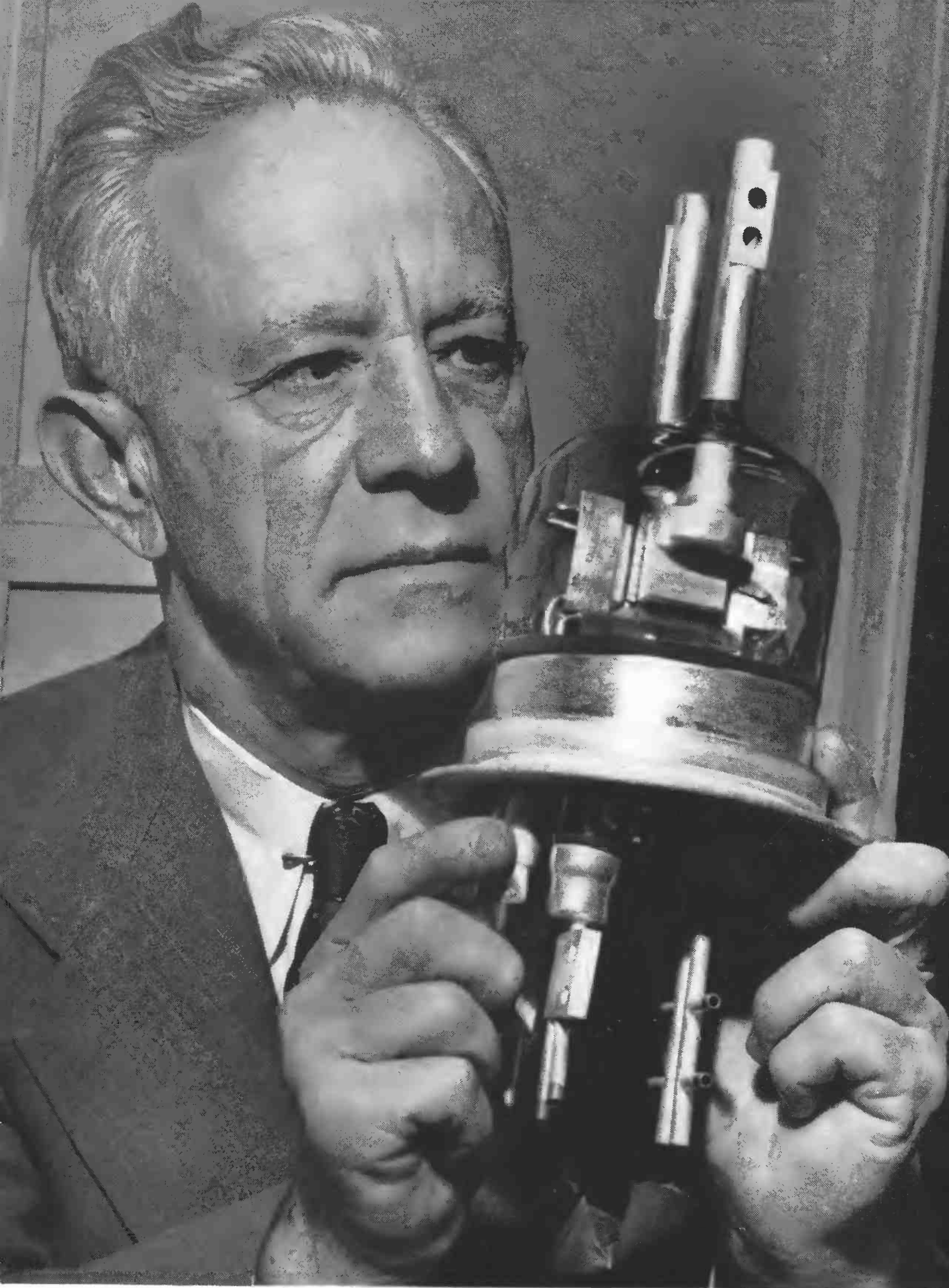
Dr. Dayton Ulrey examines the 5-kilowatt power tube developed by RCA, the first electron tube of its kind for transmission of both television sight and sound.
