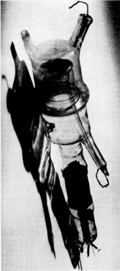
Photographs of Zworykin's 1925 camera tube. (Left) broken tube, three-quarters view, no grid in front of target; (right) three-quarters front view, grid in front of target. Courtesy of the David Sarnoff Research Center.
