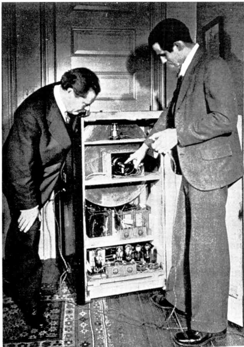
Alexanderson (left) and Ray Kell with 1928 General Electric television receiver. Courtesy of the Hall of History Foundation, Schenectady, N.Y.
