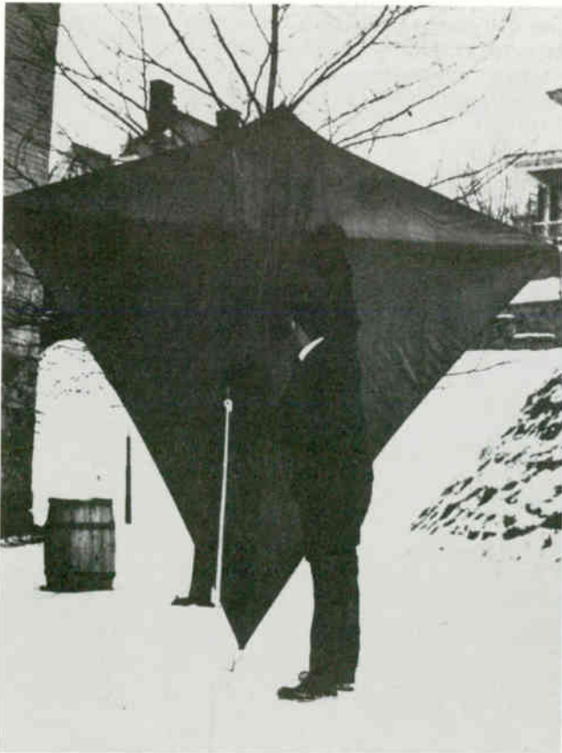
Armstrong constructed large antenna kites which he flew from the upper stories of "1032" in an attempt to improve reception.
