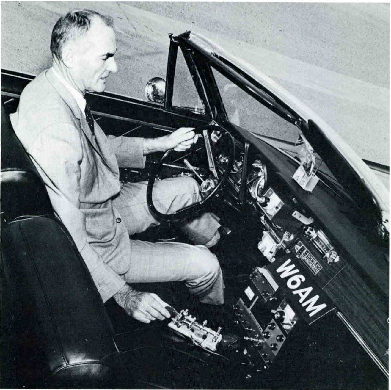
Don operating his mobile 1-kW CW rig.
