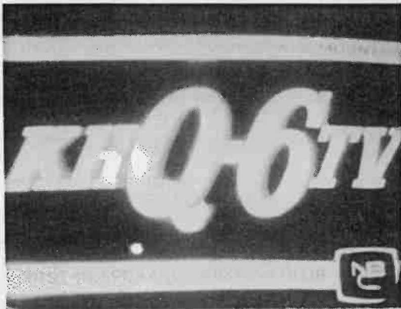
Fig. 11-1. KHQ-TV, channel 6, Spokane, Washington, received by Es over a 2025 km path at Enid, Okla. (All remaining photos in this chapter show signals received at Enid, Okla.)
