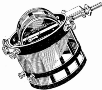
Figure 2. A space wound tuner of excellent design that sacrifices electrical efficiency wisely for greater mechanical strength
